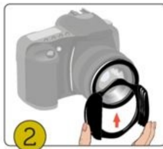
2 Slide the filter holder onto the adapter ring until it snaps in place. The filter holder is now solidly attached to the lens, yet it can rotate both left and right.
