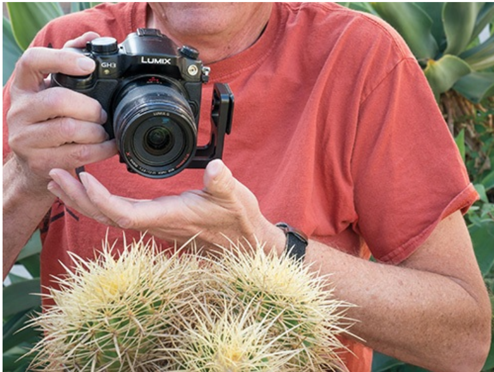
Figure 3.7 Grab your camera in your right hand, then place it into the palm of your left hand. The camera bracket seen on my camera is an L-bracket used for quick-release tripod heads.
