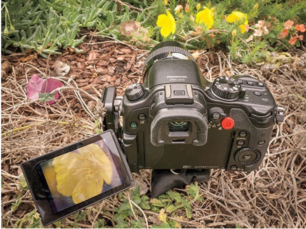
Figure 2.14 My GH3 in action, down low and up close on a beanbag. This really shows the value of the swivel LCD.
