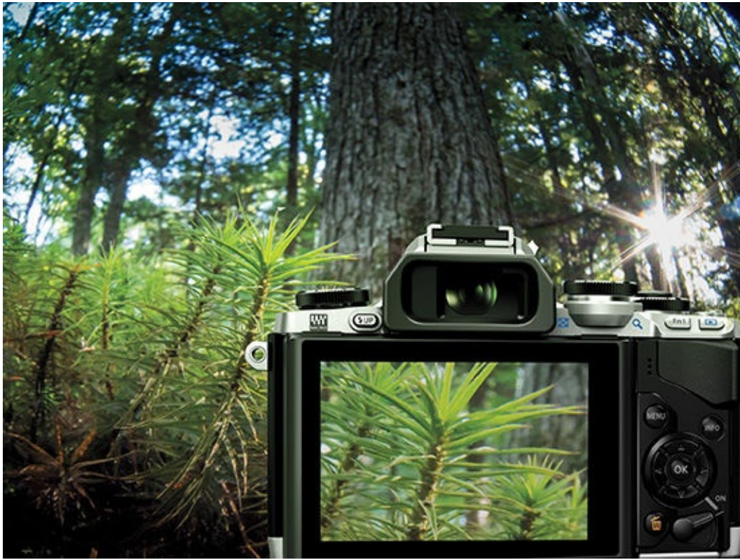
Figure 4.5 Live View allows you to focus quite precisely by seeing exactly what the sensor sees and by enlarging the view.
