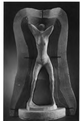
Fig. 31. Step 4. The surface of the clay model core is scraped, reducing it by the desired thickness of the final bronze. [For large sculptures this requires experienced foundry workers who know where to use thicker bronze to enhance the structural integrity of the piece.]
