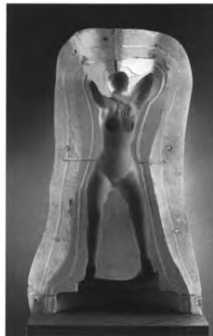
Fig. 29. Step 2. An impression of the model is made in a bed of very fine elastic material (such as latex) supported by a rigid outer mold. The supportive outer layer is designed to withstand the pressure of melted wax running through the mold.
