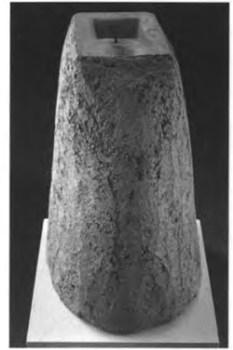
Fig. 35. Step 8. The investment mold is then heated to a high temperature and covered with a coating, which must be completely dry before bronze pouring begins. [For large casting there is often a reinforcement of the mold by metal mesh.]
