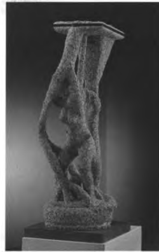
Fig. 34. Step 7. A finely granulated ceramic is gradually applied to the surface of the core model and its conduits until it becomes thick and coarse. The end result is called an investment mold. The mold is then dried and heated; the melted wax now flows through and out of the mold, leaving a space between the fire-resistant clay core and the investment mold. This method of losing the wax is called "the lost-wax process."
