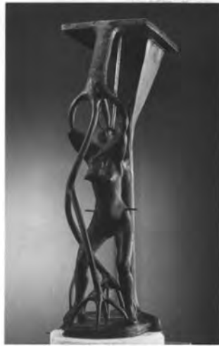
Fig. 33. Step 6. A network of wax conduits, called sprues and gates, are attached to the core model. They will act as channels through which the wax when heated will escape from the mold.
