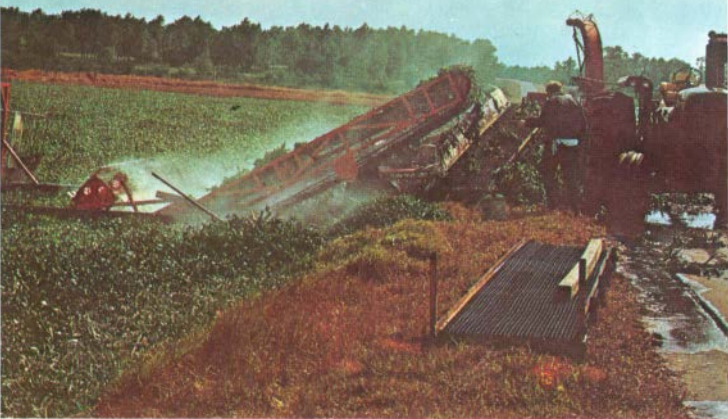
Dredging to remove water hyacinths that clog waterway
