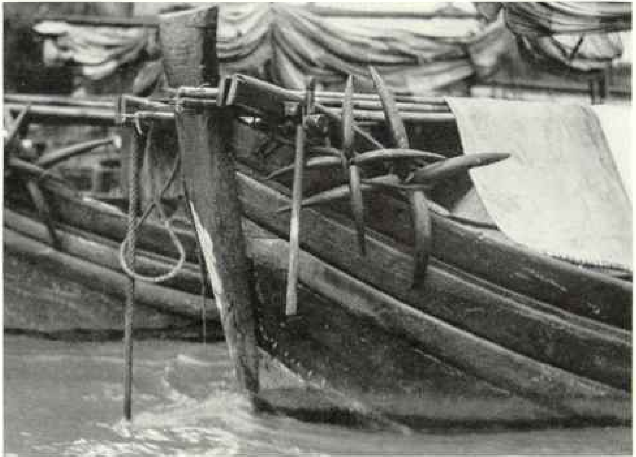
THE CHINESE ANCHOR IS USUALLY FOUR-PRONGED
