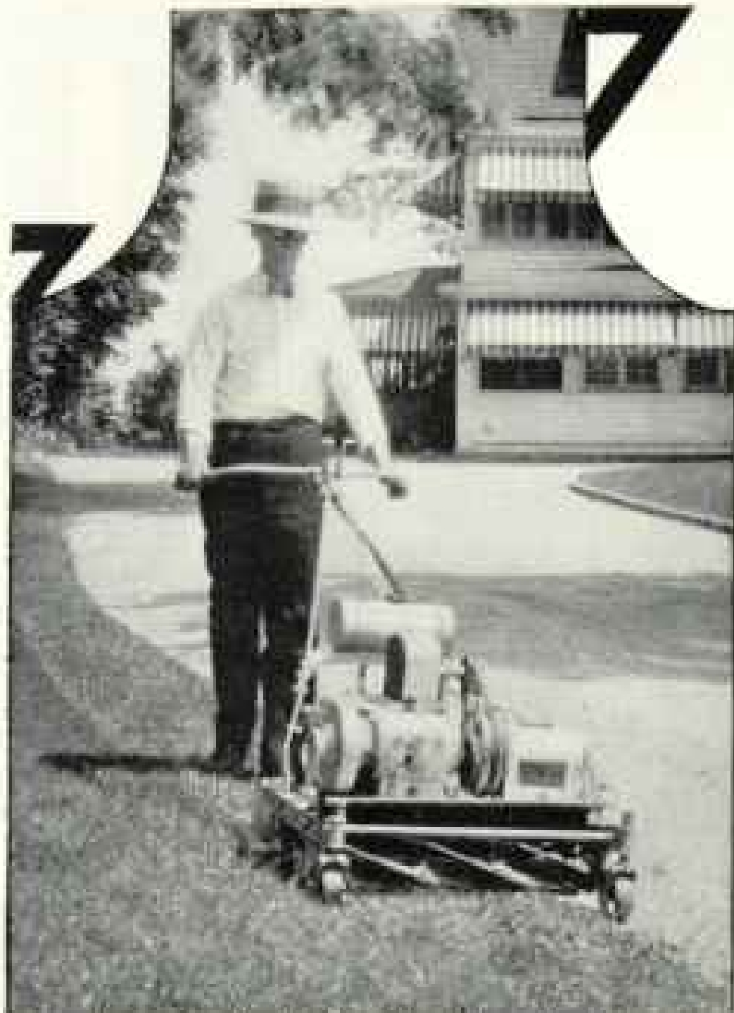
Above: Coldwell "Twin-Thirty" motor lawn mower and roller. Mows and rolls simultaneously 8 to 8 acres a day on one gallon of gasoline. Riding sulky may be had as extra equipment.
