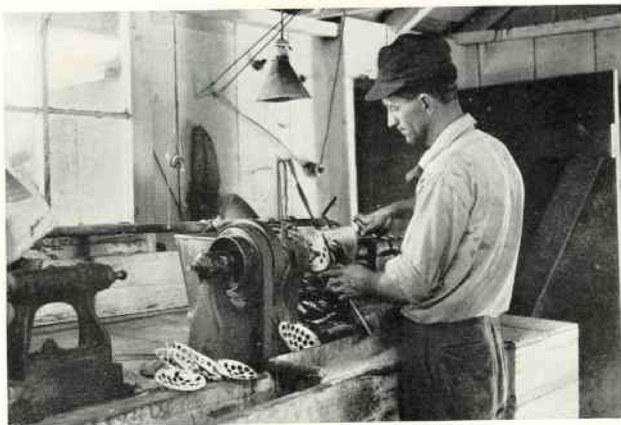
CUTTING "PEARL"-BUTTON BLANKS FROM MUSSEL SHELLS
