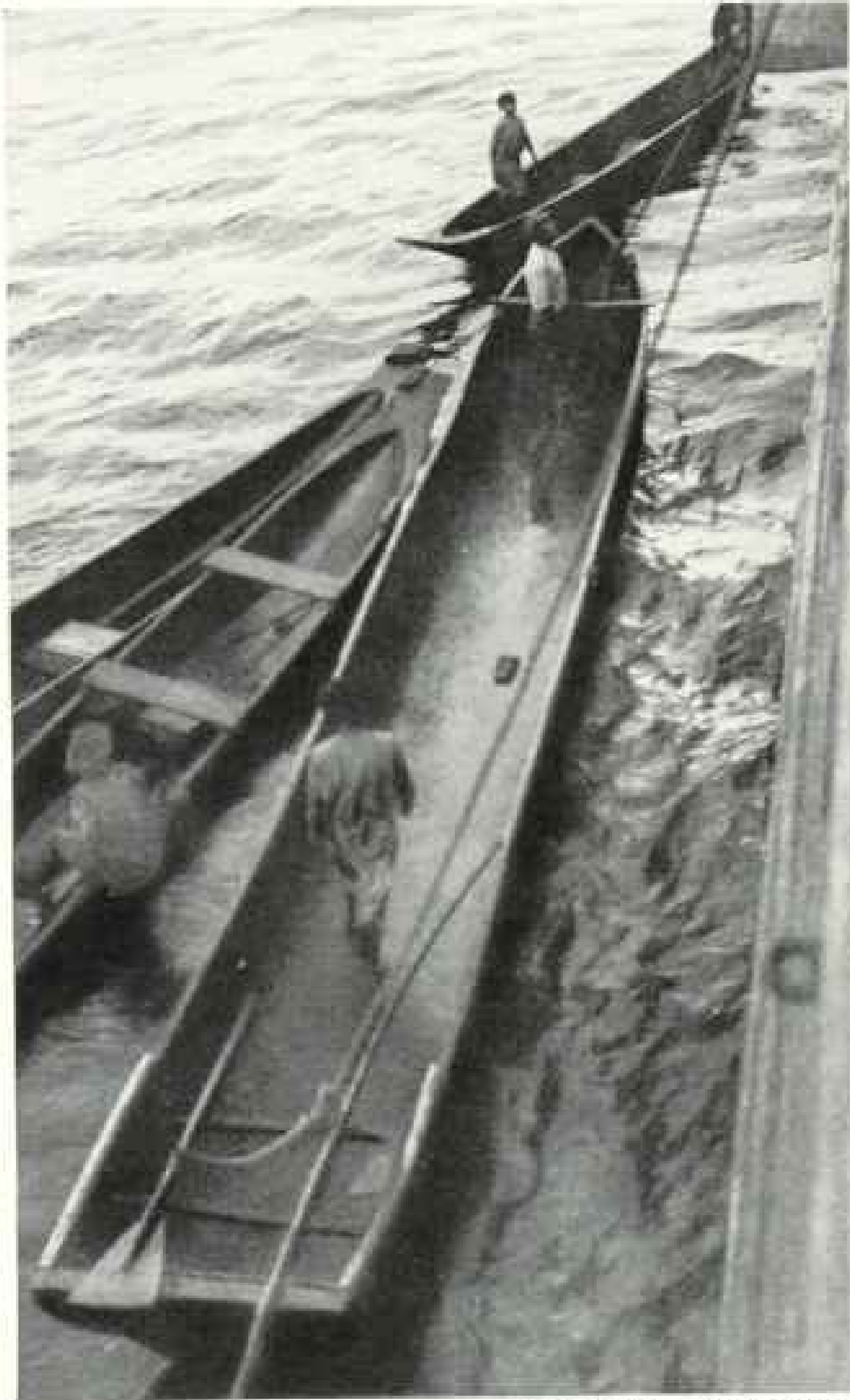
Photograph by Richard B. Huit HEWN FROM AN IMMENSE MAHOGANY LOG, THIS ROOMY COLOMBIAN CANOE HAS A BEAM OF 3½ FEET, AND IS 4 FEET DEEP
