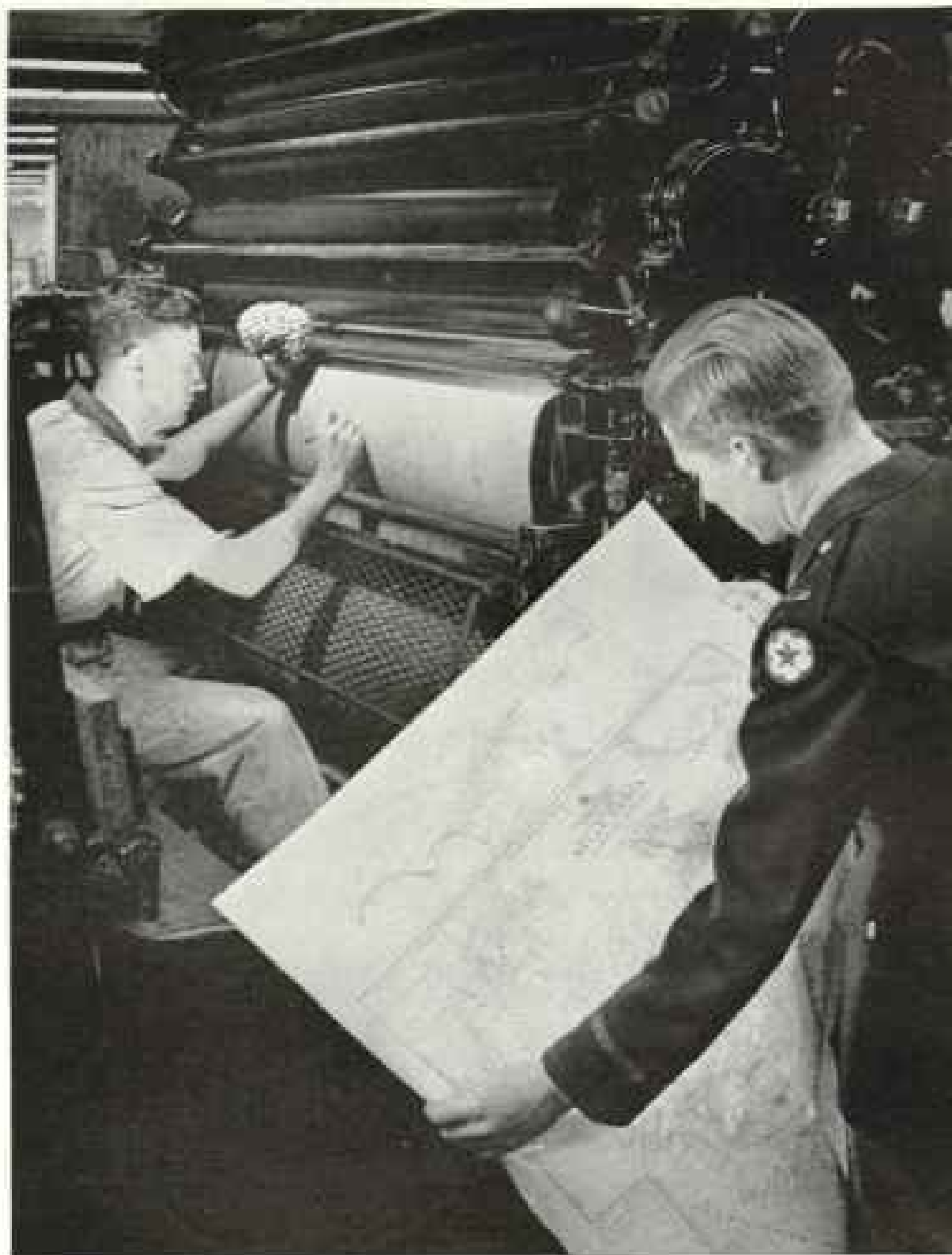
With the Plate on the Press, He Strengthens a Line Here, Corrects a Detail There
