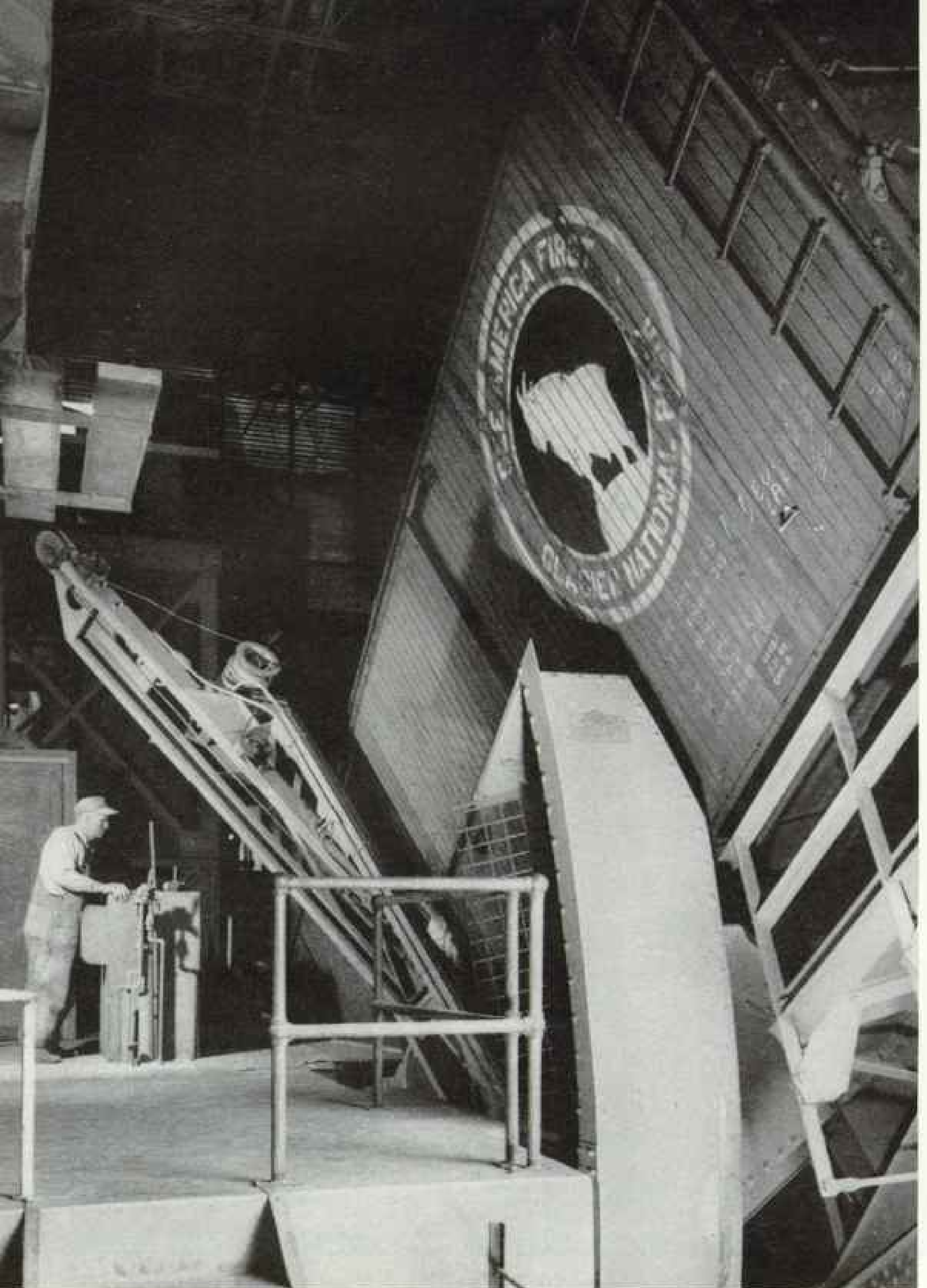
Unloading Wheat, an Electric Dumper Tilts a Ponderous Boxcar with Herculean Ease Car and contents at a Grand Forks terminal weigh about 80 tons. In seven minutes of lifting and canting, 60 tons of grain pour down chutes to storage bins. Most North Dakota wheat goes to Minnesota mills.
