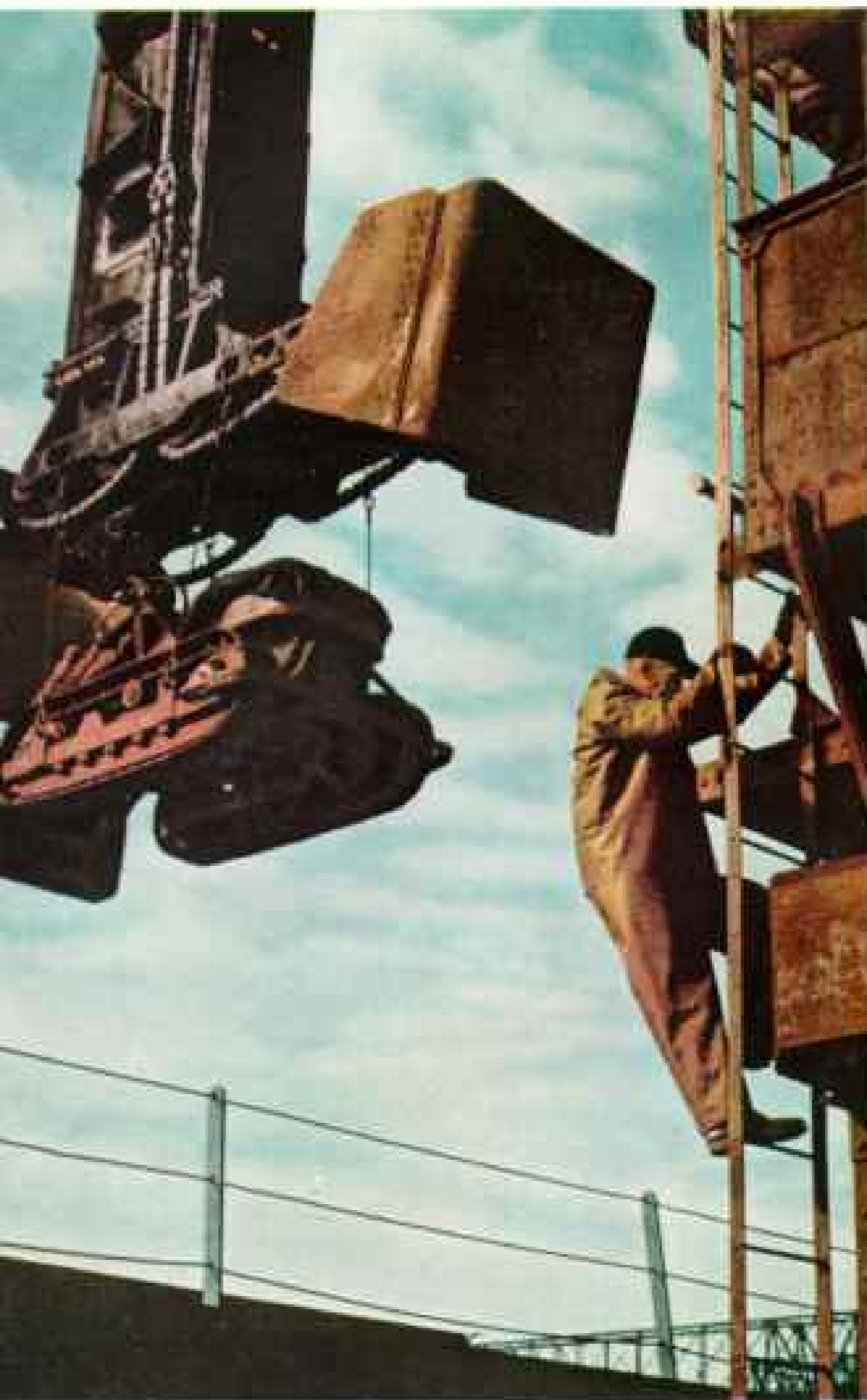
Bulldozer rides an electric shovel into an ore carrier at Ashtabula, Ohio. Called a Hulett unloader, the shovel will empty the ship's hold (right) with the tractor's assistance.
