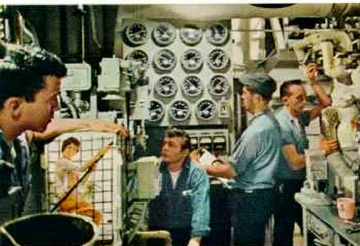
270 Distilling salt water into fresh, sailors check gauges that control evaporation. Poster girl inspires them.
