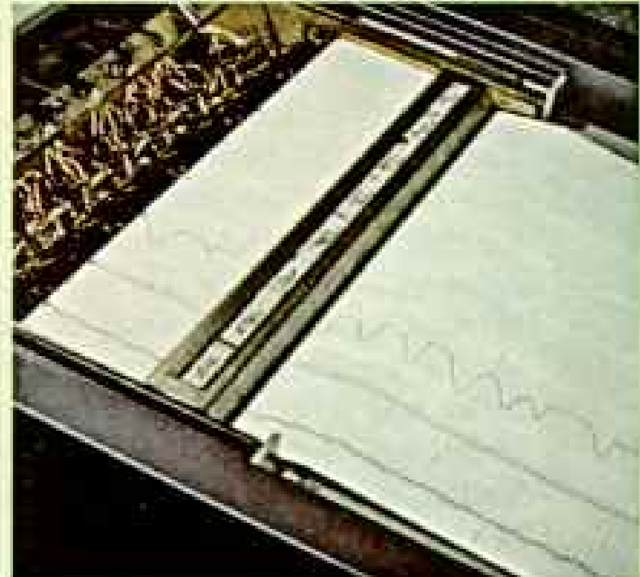
Wavy curves on a strip-chart recorder inscribe astronaut's heartbeat and respiration and the acceleration forces.
