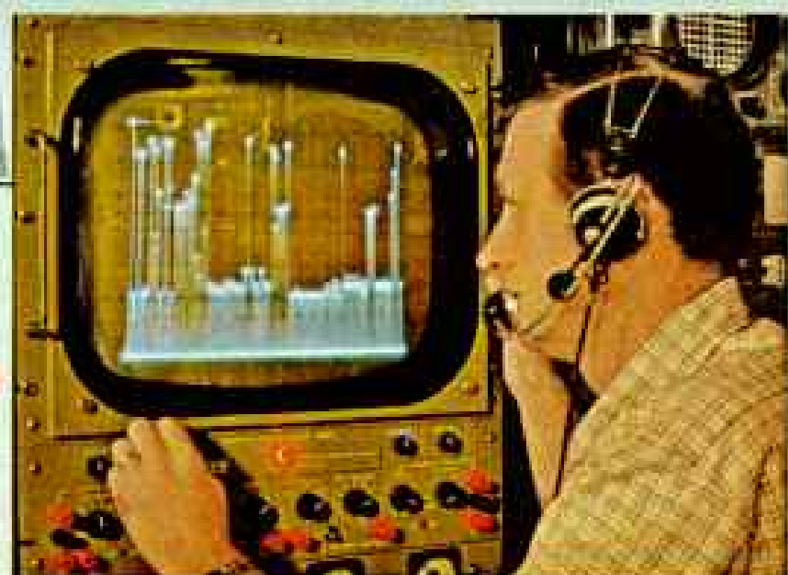
Telemetry scope shows multiple peaks representing some 90 items of information carried by radio signal from the capsule to the ground stations.
