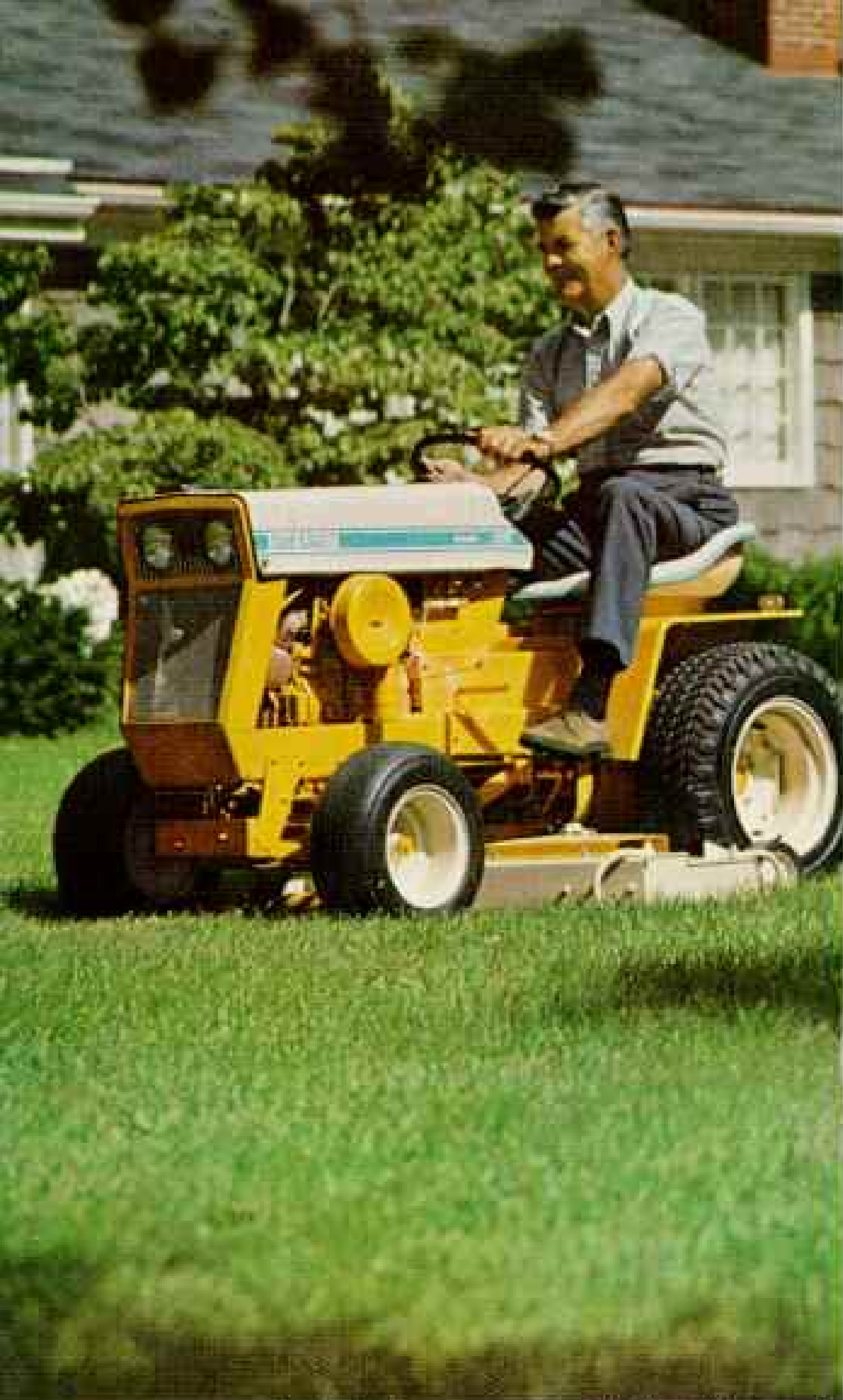
Quick-attach rotary mowers—36, 42 or 48 inches wide.
