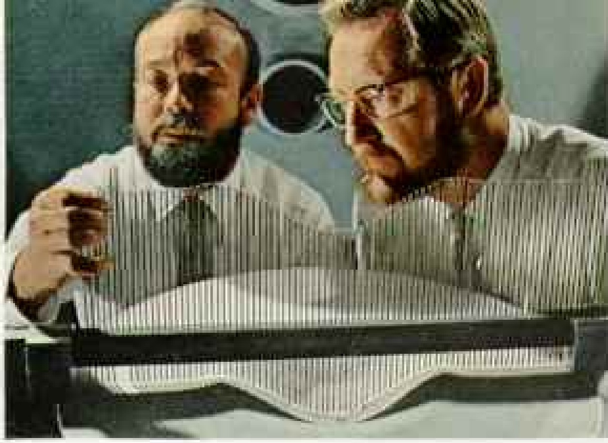
DONALD E. GAULT , right, and William L. Quaide, experts on craters, adjust rods that register contours of a man-made crater at NASA's Ames Research Center near San Francisco. An aeronautical engineer, Mr. Gault has developed a gun that hurls projectiles up to 28,000 feet a second to simulate meteorites, aiding study of crater formation.
