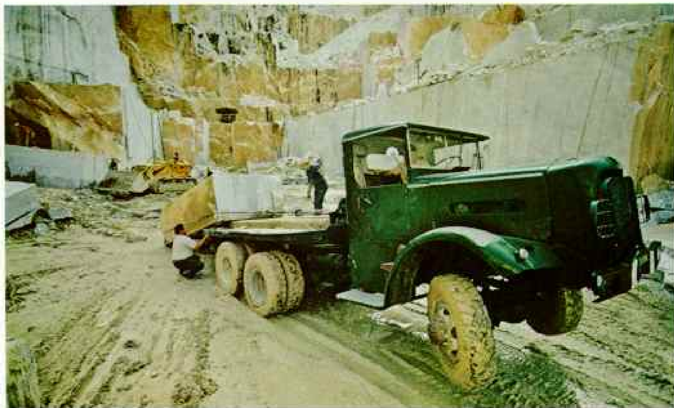
Tipping the scale against a truck's front end, a heavyweight block of marble from quarries near Carrara is eased onto a flatbed. Precarious but practical roadway to the quarries (right) has wishbone curves too sharp for trucks to round; vehicles must back along one grade, then go forward on the next.
