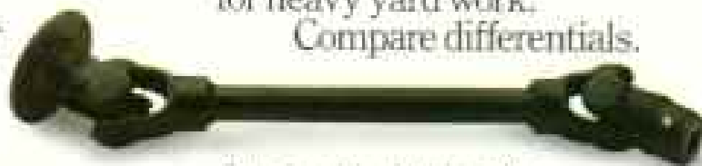
One-piece drive shaft is similar to the kind used in cars.
