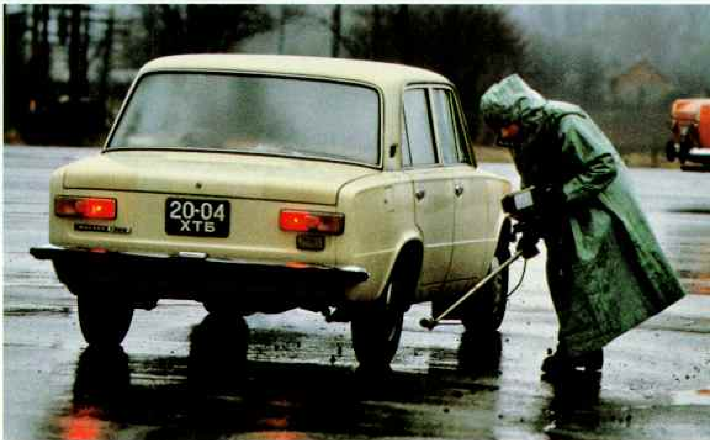
At a radiation checkpoint outside Kiev, a civil defense worker tests incoming cars with a Geiger counter, eight months after the accident. Those with excessive radiation were washed before entering the Ukrainian capital. Although fallout in Kiev never posed immediate danger, most of the city's children were sent to Young Pioneer camps for the summer, and Kievans were advised to shower frequently.
