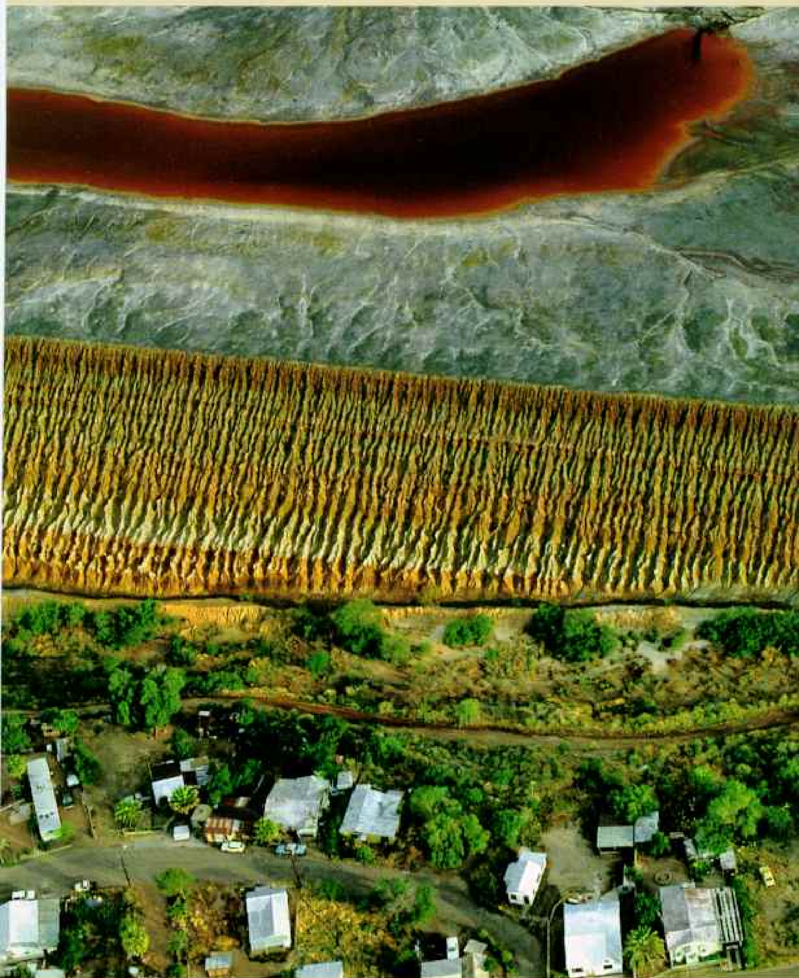
ARIZONA Backyard nightmare, a copper-tailings impoundment in Arizona reveals its toxicity in the sulfide-tinged rainwater pooling on its surface. Unless such piles of mining residue are properly contained, chemicals may leach freely into the groundwater.
