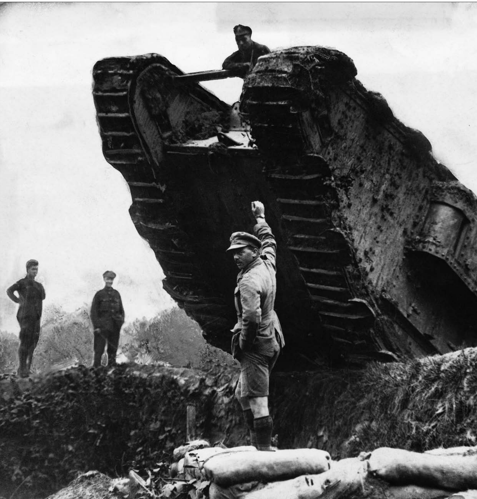
The tank was immune to machine-gun fire. It could crush barbed wire and cross trenches, and its tracks could even cope with the mud of the Western Front.
