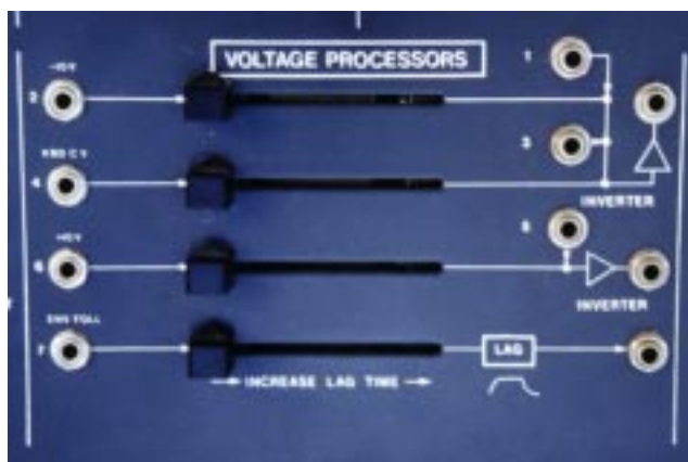
Figure 12-1: The voltage processors
