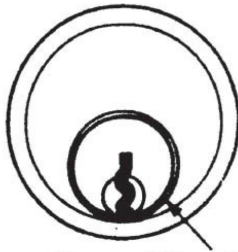
Diameter differential between plug and hole cut into shell
