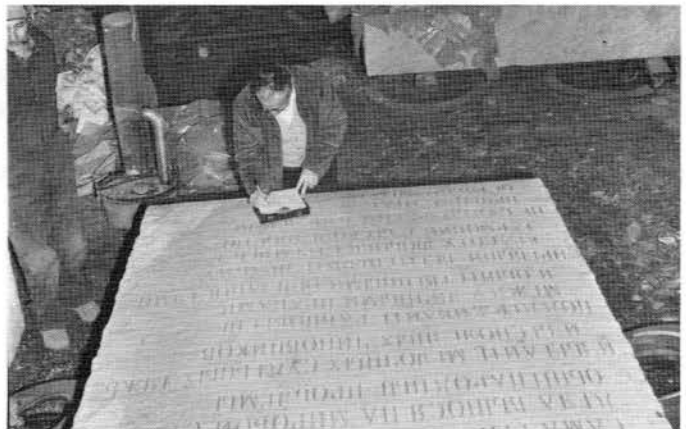
George Gaines, Chief Inspector for E.G.A.'s Certified Memorial Program, closely examined each of the units as it was completed to guarantee that each piece met specifications. The special E.G.A. seal certifying inspection was sandblown on each unit.
