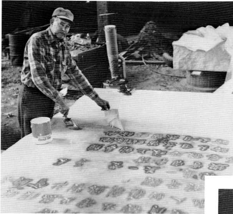
Charlie Clamp, a specialist in sandblast engraving and cleaning granite, glues stencils of the Chinese characters on one of the stones. The four outer stones are inscribed with the same "message" but in eight different languages. The capstone is inscribed in four languages.
