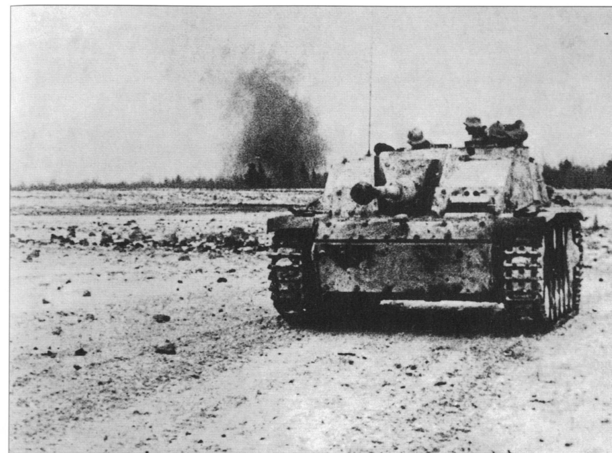
Above: A Leibstandarte Sturmgeschütz (assault gun) III or StuG III seen at Kharkov in the spring of 1943. The StuG III was used in both a support and an anti-tank role, the latter increasingly important as Soviet tank numbers grew.
