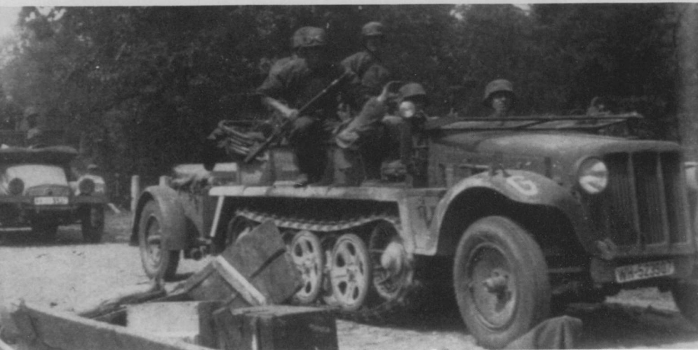
An SdKfz 10 one ton halftrack of Reich is seen being followed by a Krupp Protz L2H143 gun tractor Kfz 69, more commonly known as Boxer. The White "G" indicates that Reich was part of Guderian's 2. Panzer-Gruppe. The use of a Wehrmacht vehicle, without bothering to change the license numbers, indicates the haste with which the establishments of the SS divisions had been increased between campaigns.
