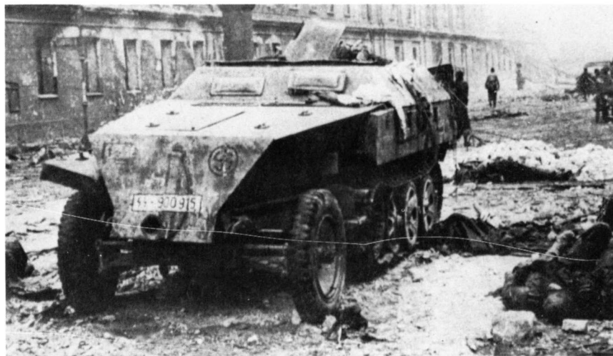
Having withdrawn all the way from Oranienbaum to Berlin, Nordland fought its last battles around the grave of its Führer. It died too. Among the last of its vehicles, this late SdKfz 250/1 ISPW is seen in the streets of Berlin. It was painted overall Sand Yellow with a hasty Red Brown overspray and a great deal of dirt. The division fought on for a few more days, surrendering in Charlottenberg, just West of the city.
