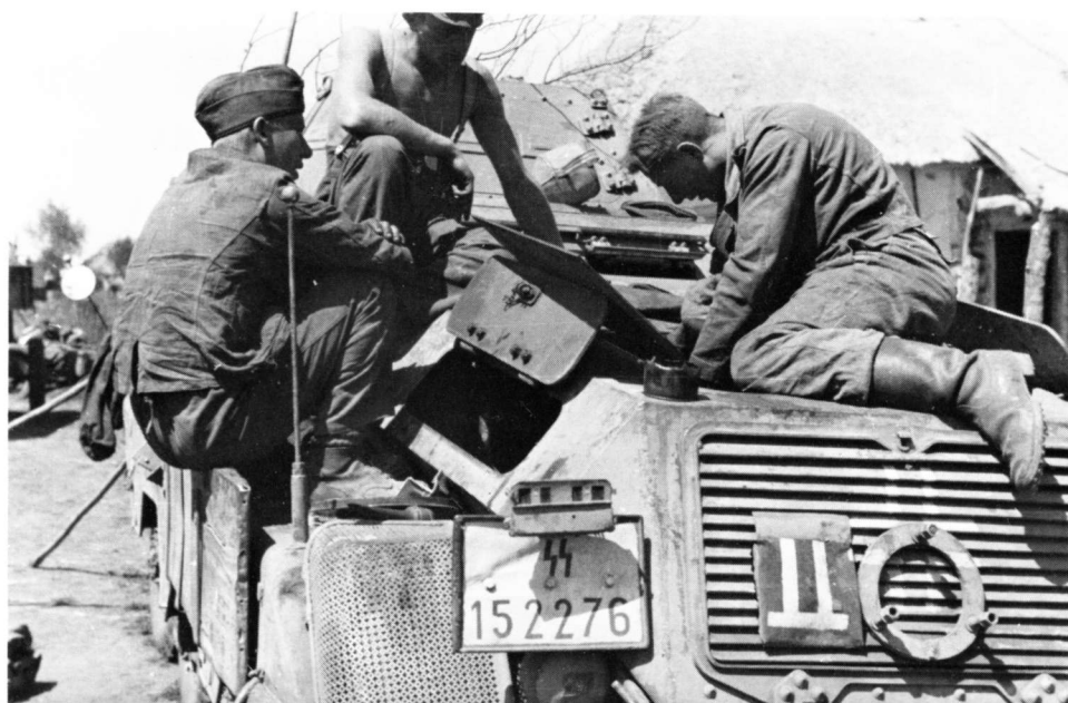
An interesting shot showing three mechanics working on the engine of a Das Reich SdKfz 231 eight wheel armored car. The spare tire obviously was missing before the vehicle was repainted Sand Yellow. Of interest is the plate upon which the divisional insignia has been painted. It was partly masked off during repainting, showing to good advantage the apparent difference in tone between Panzer Grey and Sand Yellow. [Bundesarchiv]
