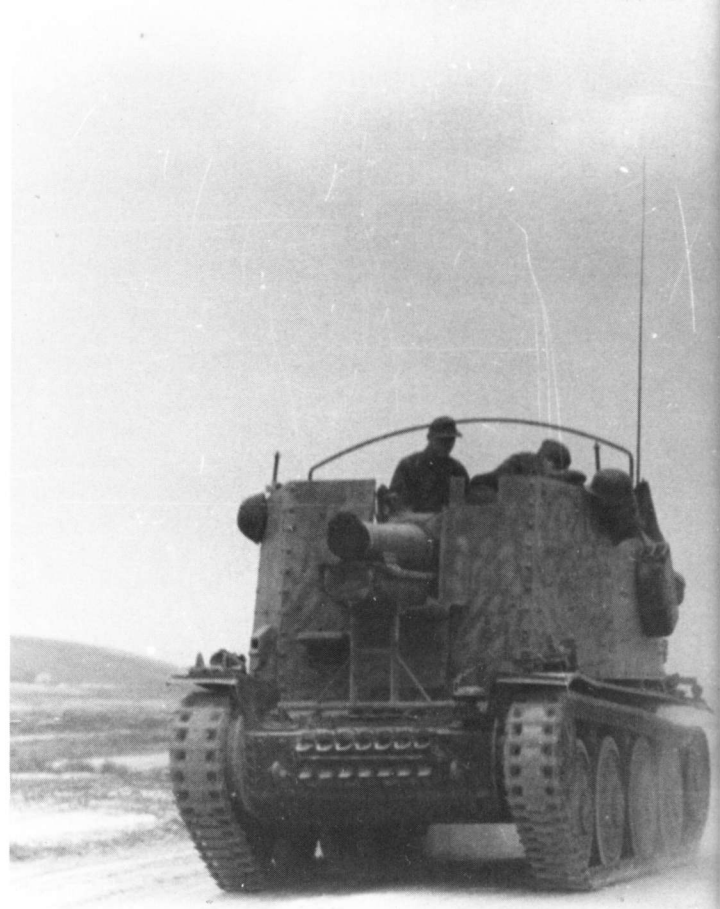
[Above & Left] Two views of a convoy of armored vehicles of Das Reich on a dusty road behind the Kursk front. The 15cm sIG Bison seen above is Sand Yellow with a complex overspray of Olive Green. At the left is an SdKfz 251/1 mSPW carrying a member of the division's Feldgendarmerie [Military Police]. He can be seen leaning on the edge of the APC's fighting compartment, holding his Red and White traffic control paddle. [Bundesarchiv]
