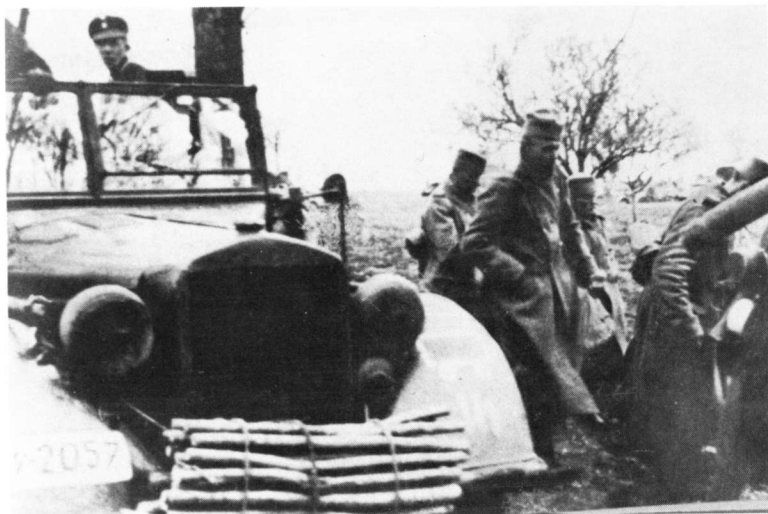
One of Reich's original vehicles [as can be ascertained from the four-digit license number], a Kfz 15 Horch, is being passed by a column of Yugoslav prisoners during that division's brief participation in the Balkan Campaign. Of note is the small bundle of sticks tied to the front bumper in case mud is encountered.
