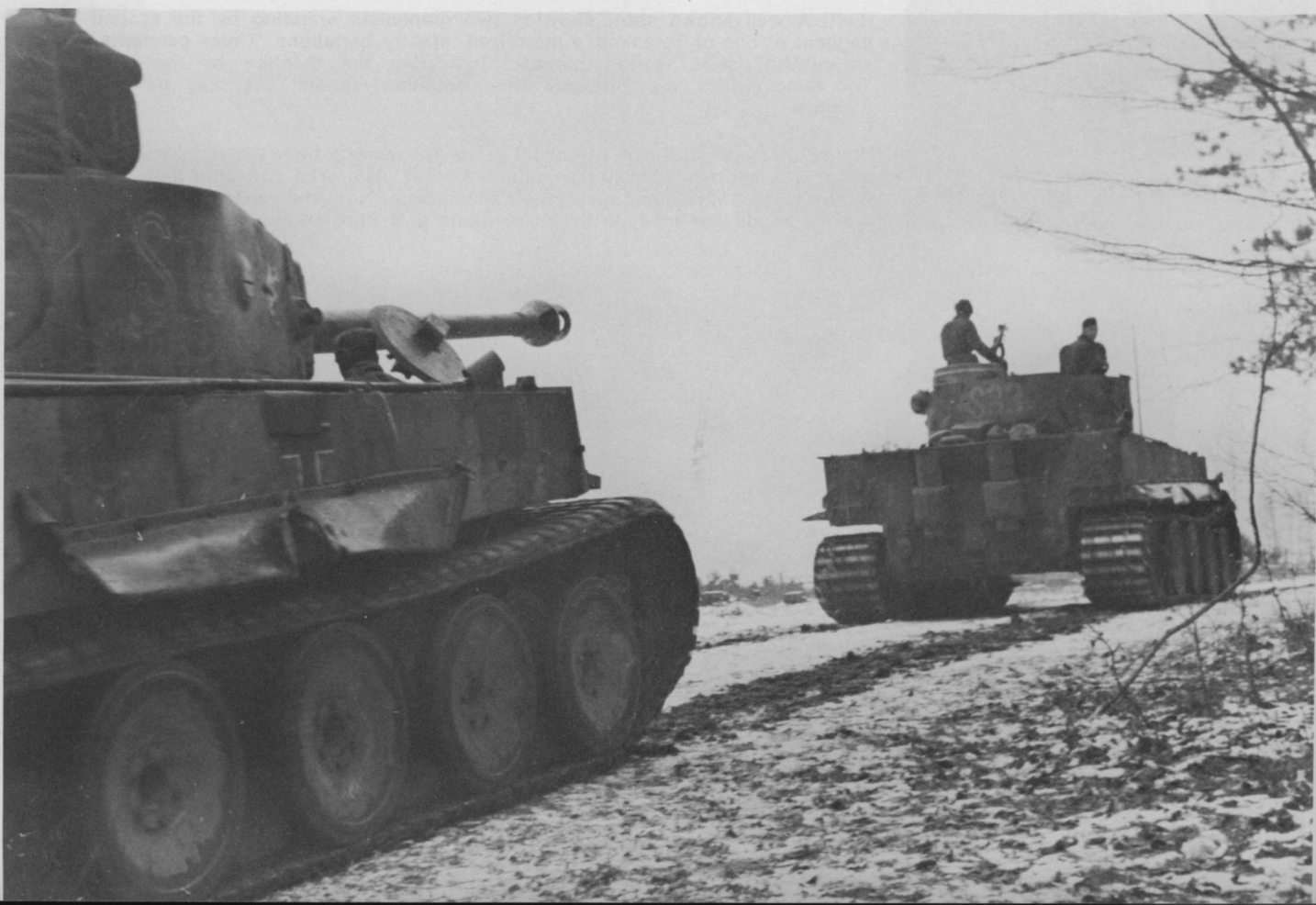
An old friend, "S13" of Das Reich's sPz-Abt follows "S33" through the first snow of the Winter 1943. Last seen in the wheat fields around Kursk, these Tigers are now a little worse for the wear. Note the extensive damage to the external fittings such as the Feifel system, "S" mine projectors and hull skirts. In spite of the onset of Winter, these vehicles are still in their Sand Yellow and Red Brown camouflage. [Bundesarchiv]
