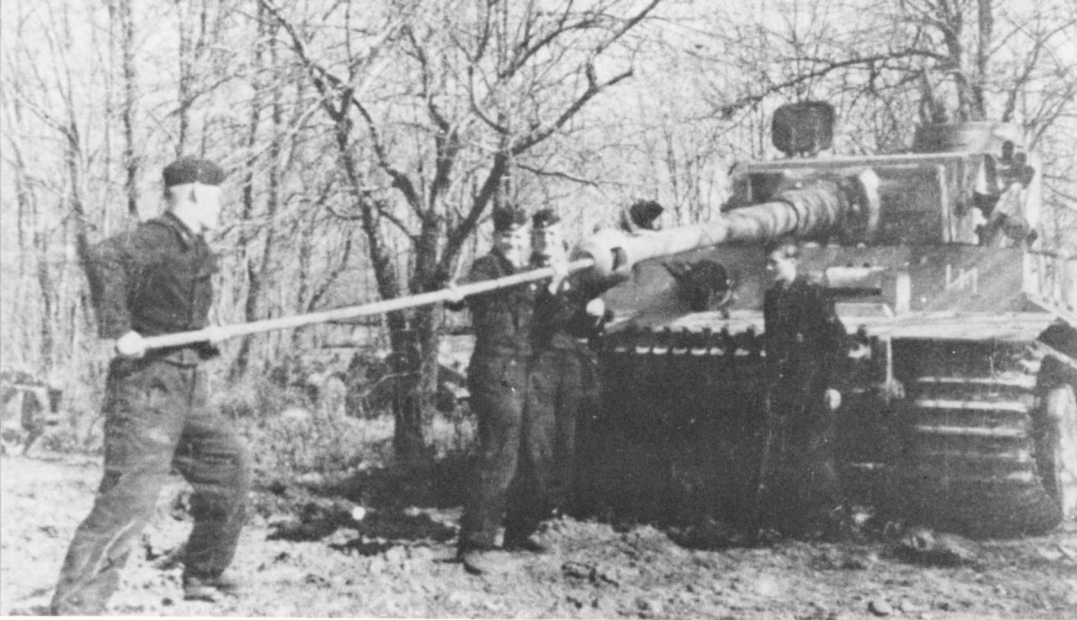
Two views of the new Tiger ausf Es that were being issued to the heavy tank battalions of the SS divisions. These Tigers of Das Reich are extremely early models, complete with the "S" mine projectors at the corners, early stylized cupola and Feifel air cleaning system. The tank to the right in the shot below is a PzKpfw III ausf M or N. Many new vehicles at this date were arriving still painted in overall Panzer Grey, these have had their original color oversprayed. In the view to the left, notice that in combination with natural shadow, this camouflage scheme was effective in breaking up the shape of the vehicle. [Bundesarchiv]
