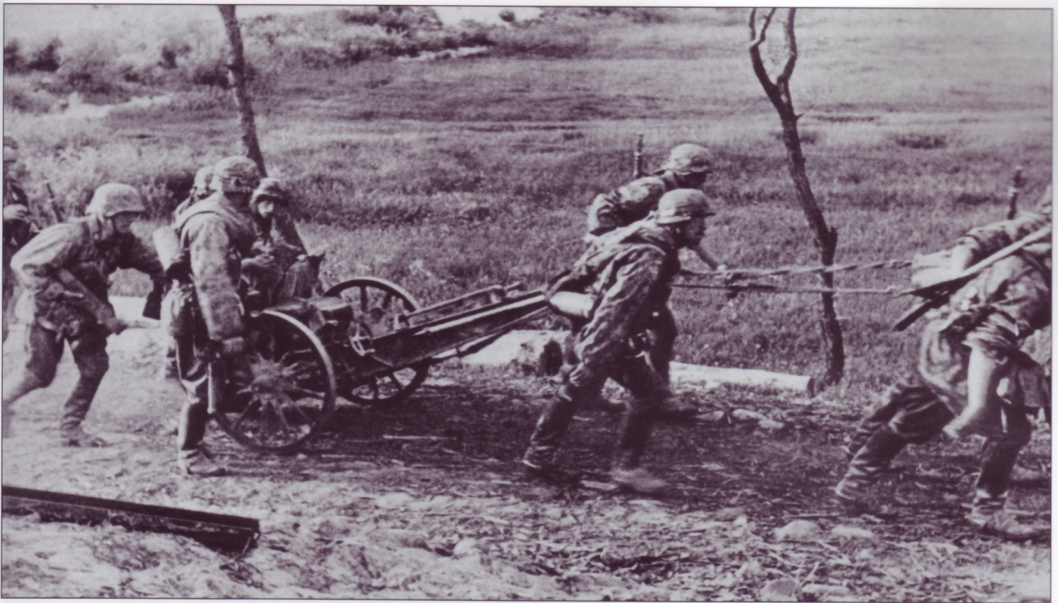
Waffen-SS troops haul a 7.5cm I.I.G.18 light infantry gun. This version has wooden-spoked wheels for transport by horse teams, while a rubber-tired version was available for vehicle towing. The infantry gun was introduced as the result of lessons learned in World War I, where the guns of the era proved too heavy to keep up with infantrymen crossing the extremely rough terrain of "no-man's land". This infantry gun was relatively light, simple to operate, and capable of direct fire against enemy machine-gun nests. It could also fire at a high trajectory against dug-in troops. An infantry regiment's 13.Kompanie usually had four 7.5cm I.I.G.18s and two 15cm s.I.G.33s, although the SS often lacked the latter.
