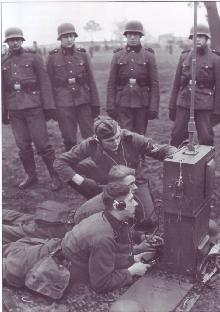
Radiomen undergo training with a Tornisterfunkgerät b1 (Torn. Fu. b1 (S/E), or "pack radio"), a widely used portable tactical radio, in March of 1941. The radio's upper and lower halves were each carried by a soldier on a specially designed back-pack frame, and when connected to each other via cables, could be used "on the march". The standard training practice was for some students to operate the equipment under the tutorage of an instructor as the others watched; then they would take their turn.
