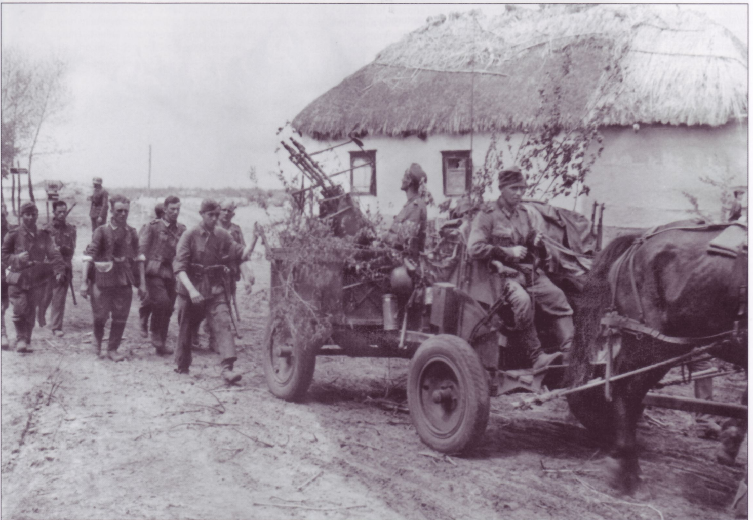
Troops pass through a Russian village accompanied by an If.5 machine gun wagon (Maschinengewehr-Wagen) with twin 7.92mm MG34 machine guns on a mount 36 (Lafette 36). Besides ammunition and machine gun accessories, the six-man crew's individual equipment was carried as well. Typically log cabins were encountered, what the Germans called an Isba, the barrowed Russian word for a log cabin. However, this one has plastered walls, but still a thatch roof.
