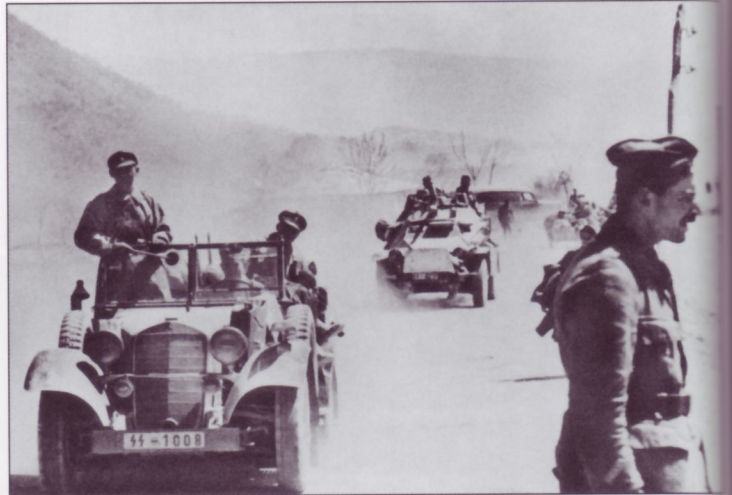
The Kfz.15 medium cross-country car was one of the most common models used by the Waffen-SS. It is followed by an Sd.Kfz.222 armed with a 2cm automatic gun and a 7.92mm machine-gun.
