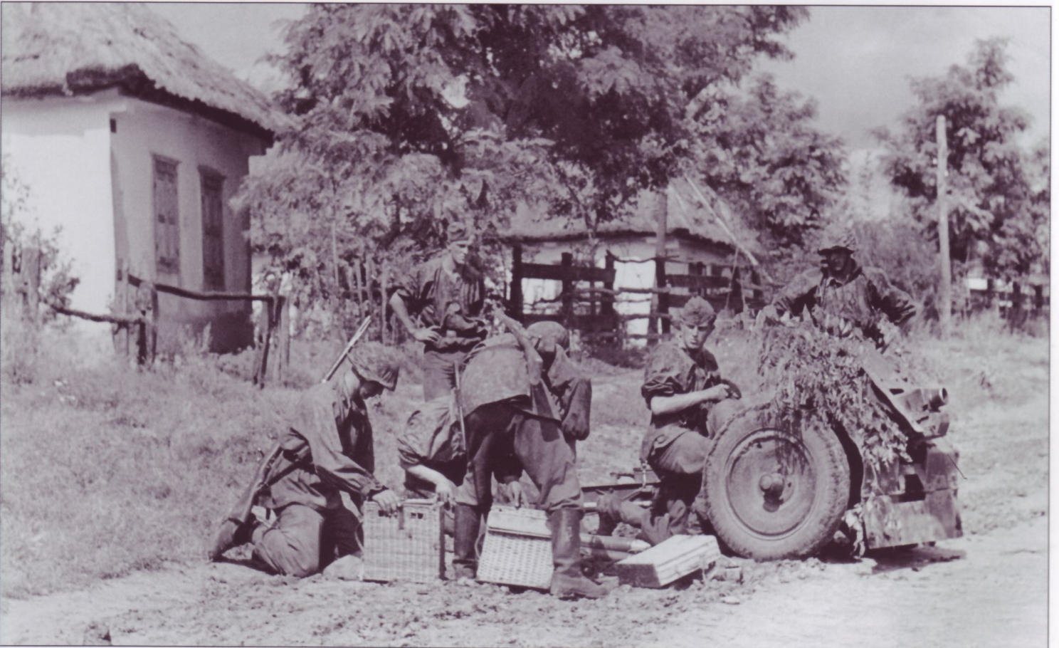
The Waffen-SS crew of this 7.5cm I.G.18 prepare to open fire. This version had the rubber tires, which were optimized for motor vehicle towing. The ammunition is carried in wicker containers each holding four rounds. Their individual weapons are 7.92mm Gew98 rifles.
