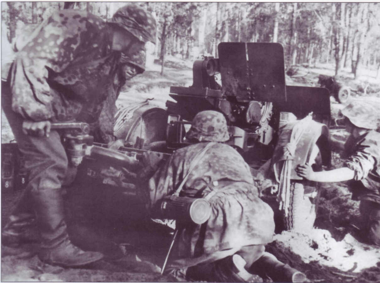
The crew of a 2cm FlaK38 anti-aircraft gun (probably from the "Totenkopf" Division) manhandle it into position. The gun was normally emplaced after being detached from its two-wheel Sd.Ah.51 carriage. Besides air-defense, these light weapons (which fired both high-explosive-tracer and armor-piercing-tracer ammunition) were used against ground targets to include personnel, field fortifications, and light armored vehicles.
