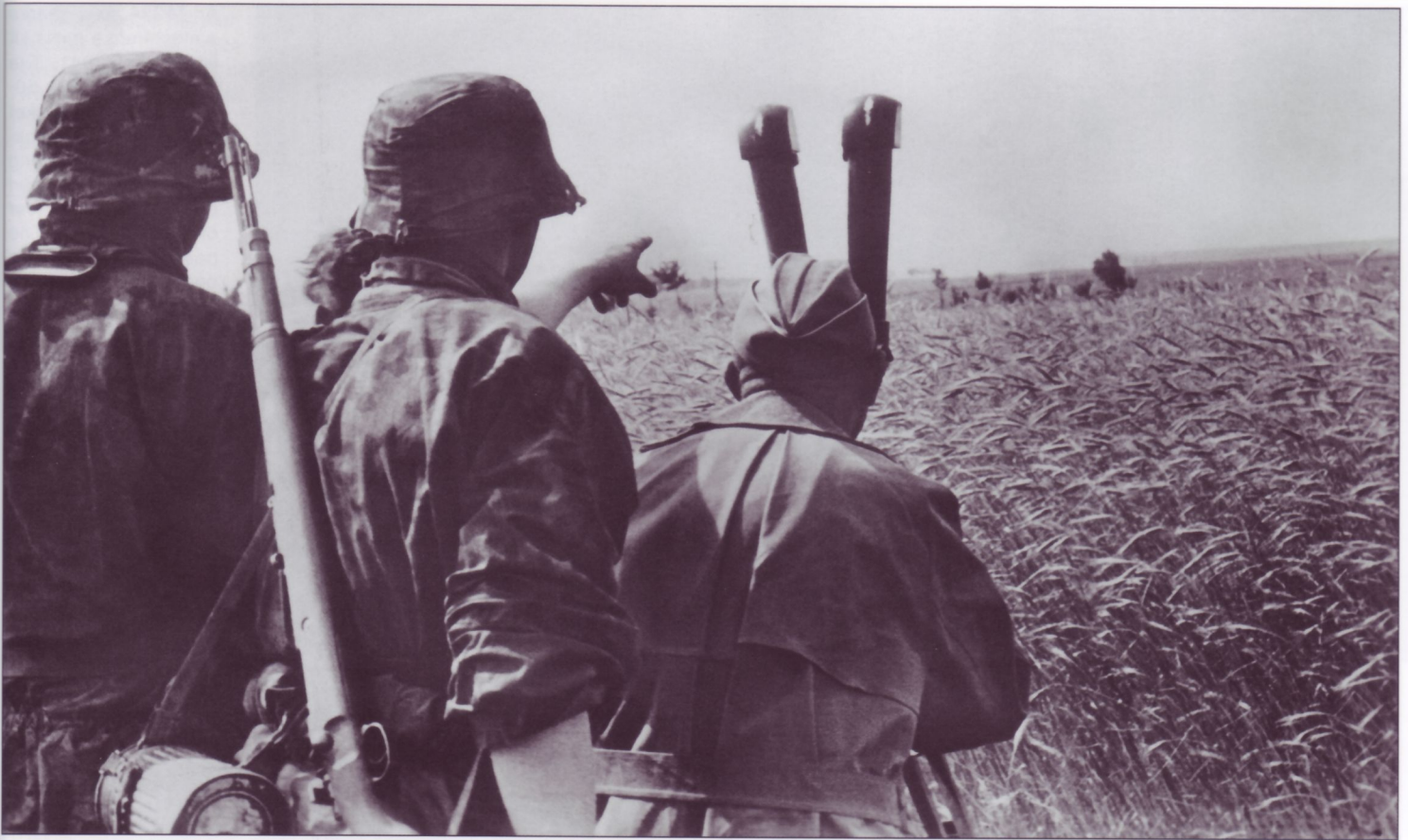
An artillery observer searches for a target hidden in a vast field of wheat, August 1941, somewhere in Russia. The observer is using a 6x30 Sf.14Z scissors periscope. The oval object on the back of the soldier's neck to the left is a leather eyepiece cover for binoculars. Attached to the carrying strap they were often pushed out of the way to the back. The man in the center carries a Kar98k carbine, but this being a Waffen-SS unit, it could just as well be license-produced copies made in Czechoslovakia, Poland, Yugoslavia, or Austria.
