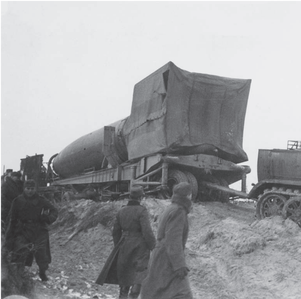
Rugged and highly mobile, the A4 rocket can be hauled around the countryside on its mobile Meillerwagen transporter and launch rig. Here it is dragged into position on a dune near Peenemünde in 1944.
