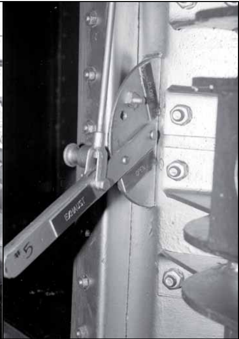
Fig. 85: Closeup of lever used to open and close exhaust stack.
