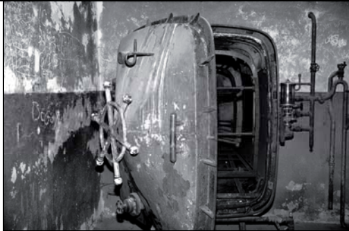
Fig. 79: Hot air disinfestation autoclave in Mauthausen camp, similar to that in Birkenau (see previous Fig.).
