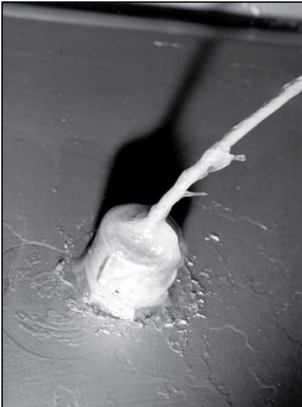
Fig. 98: Closeup of where monitoring line enters chamber also coated in vaseline.
