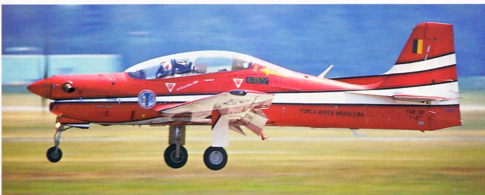
Below: The Embraer EMB 312 Tucano is a very successful Brazilian turboprop, tandem-seat trainer. The Brazilian Air Force aerobatic team Esquadron de Fumaca or Smoke Squadron operates it. Tucano T27 FAB 1311 is airborne at Abbotsford, BC, August 1986.
