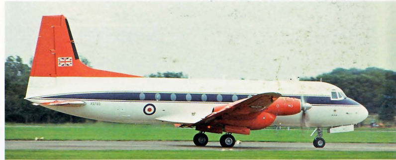
Left: The Andover C1 was a special military freighter. The entire rear end was redesigned to accommodate a rear-loading ramp that could open in flight to airdrop paratroopers or cargo. The undercarriage had a 'kneeling' facility to lower the loading ramp to floor level. Andover C1 XS612 of 46 Squadron RAF is at Leuchars, September 1974.
