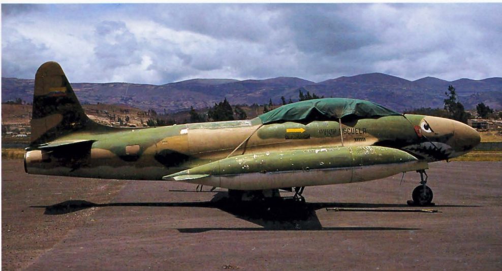
Above: The US Navy variant of the T33 was the TV2 . As can be seen, the area behind the cockpit is quite different. The aircraft is also equipped with a tail hook. 144204 7W is the base flight aircraft at Willow Grove, August 1970. (SGW)
