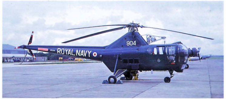
Right: The Westland Dragonfly was a British-built version of the Sikorsky S51. A single 550 hp Alvis Leonides piston engine provided power. Dragonfly HR5 WN500 904/BY is operated by RNAS Brawdy as a station flight aircraft; it is pictured there in July 1962. (AG)
