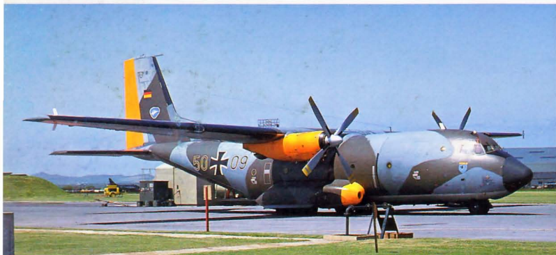
Below: The Transall C160 was a joint German/French transport aircraft powered by two Rolls-Royce Tyne turboprops. C160D 50+09 of Luftwaffe transport unit LTG 62 is at Brawdy, May 1980.
