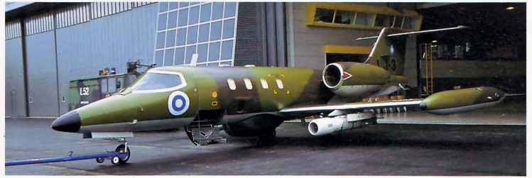
Below: The Finnish Air Force uses its three Learjets to perform a multitude of tasks. These include target towing, aerial mapping, electronic warfare training and maritime patrol. Learjet 35A LJ3 is pulled from its hangar with a target towing device under the wing. It is operated by the 1st Flight of the Air Support Squadron at Tikkakoski where it was photographed in June 1998.
