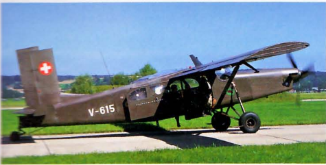
Below: The Pilatus PC6 Porter has been built with both piston and turboprop power. The aircraft is a single-engine, high-wing utility type with STOL performance. V-615, a turbo, of the Swiss Air Force is seen at Dübendorf, August 1987.
