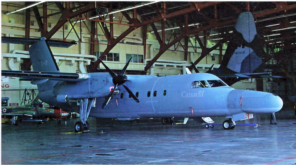
Above: To train its navigators the Canadian Armed Forces have adapted the popular de Havilland (Canada) – now Bombardier – DHC8 Dash 8 short-haul airliner. To do this they have added mapping radar in an extended nose. CT142 142804 of the Air Navigation School was at its Winnipeg base in June 1990.
