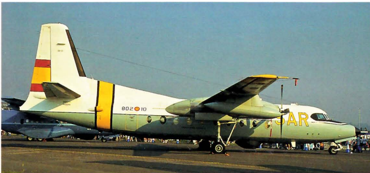
Above: During 1975 Fokker produced a Maritime Patrol F27. Equipped with search radar and a twelve-hour endurance it sold in small numbers. F27-400MPA D.2.01 802/10 is operated by Esc 802 of the Spanish Air Force. From its base at Gando in the Canary Islands it can cover a large area of the Atlantic Ocean. It is seen at Fairford, July 1996.
