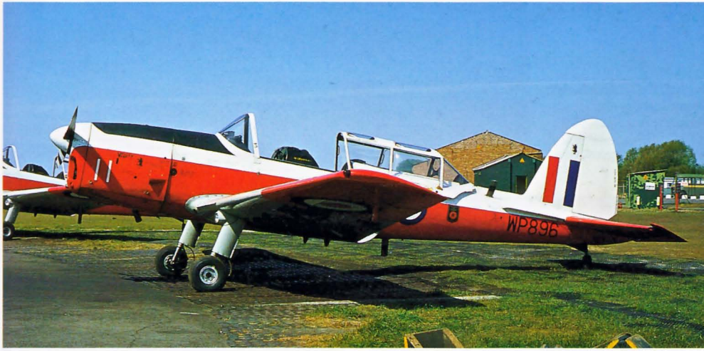
Above: The de Havilland (Canada) DHC1 Chipmunk was a single-engined, tandem-seat, basic trainer for the RAF. Chipmunk T10 WP896 is operated by 10 AEF (Air Experience Flight). It is seen at its Woodvale base, May 1984.
