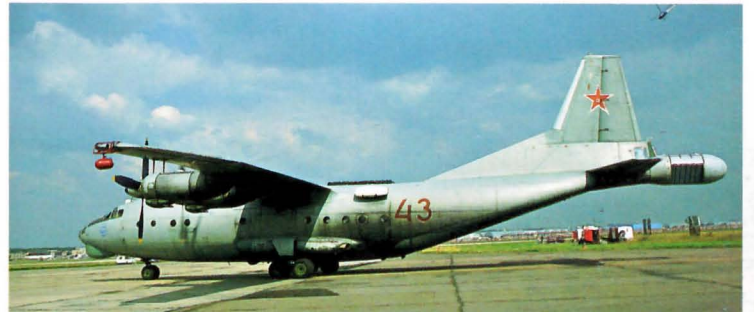
Below: Like the C130 the An-12 has had many more roles than just transport. This example 43(Red) is an An-12BP (Mod) of the Russian Air Force. It is used to test ejector seats, these can be fired either up or down from the cone in the tail. On the wing tips are cameras to record the events. It is pictured at its Zhukovsky base, August 1997. (JDS)
