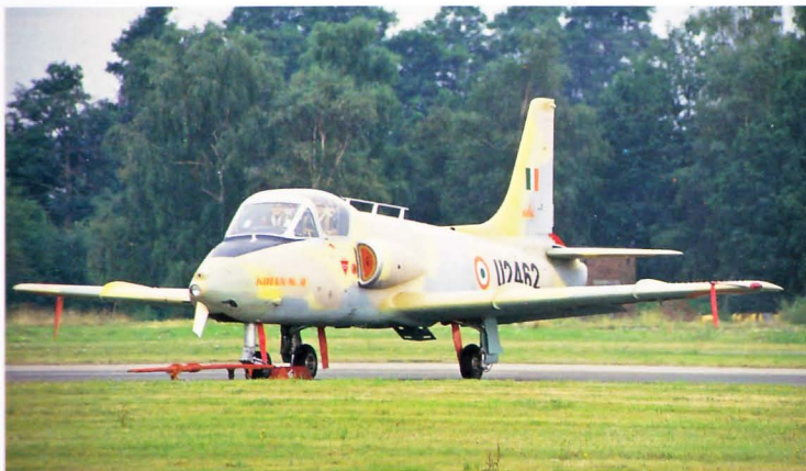
Above: India in a desire to adopt a local design for its requirement of a basic jet trainer produced the Hindustan HJT-16 Kiran . It first flew in 1964 and was quite advanced having zero altitude Martin-Baker ejector seats and cabin pressurisation. U2462 is seen at the Farnborough Air Show, September 1964 on a sales trip.
