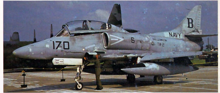
Above: The TA4J was used by the US Navy as an advanced trainer. It was basically an 'F' model with the weapons systems removed. 154291 170/B of training squadron TW2 is at London, Ont, June 1990. It carries the name of USS Lexington , the then training carrier.
