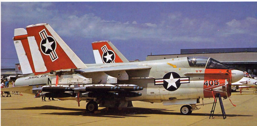
Above: The conversion trainer for the Corsair II was the TA7C. These were converted 'B' & 'C' models. Showing the two cockpits open is 156795 204/NJ of VA122 (USS Lexington), at Lemoore, CA, October 1979.
