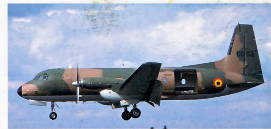
Above: One of the successful 'Dakota Replacements' the Avro (Hawker Siddeley) 748 has sold well world-wide. Powered by a pair of Rolls-Royce Dart turboprops, it could operate from grass runways. HS748-288 CS-03 of the Belgian Air Force is seen at Farnborough prior to delivery, September 1976. Note the cargo door is open in flight. The aircraft are used for either passenger or freight operations and are quickly converted to either role.
