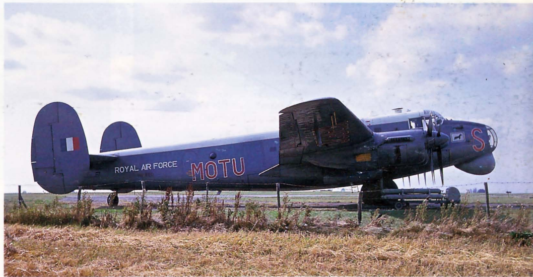
Above: Training for Shackleton crews was provided by the MOTU (Maritime Operational Training Unit) on the T4 model. This variant had the armament removed and additional radar positions for trainees. WB820 of S/MOTU is at Odiham, September 1964. (AG)
