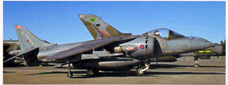
Below: The T10 Harrier is a combat-capable trainer based on the new generation airframe. ZH654 of the A&AEE is at Fairford, July 1995.
