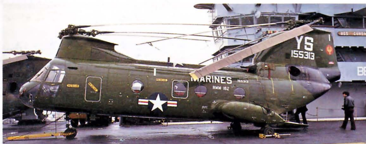
Above: The Boeing Vertol H46 Sea Knight was produced for the US Marine Corps as an assault troop carrier. It could carry seventeen fully equipped Marines or a 4000 lb cargo load. CH46F 155313 1/YS of HMM162 is aboard USS Guadalcanal , October 1978.
