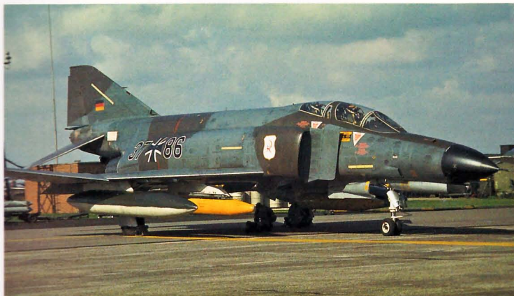
Above: The F4F Phantom was a special German variant. It was in essence a simplified and lighter F4E with many parts built in Germany and shipped to St Louis for final assembly. 37+86, an F4F of JG 71 'Richthofen', based at Wittmundhafen was photographed at Binbrook in September 1977.
