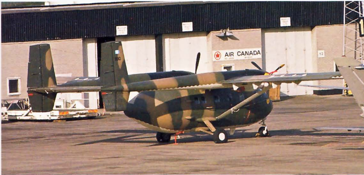
Below: With the same powerplant and a similar size and layout, except for the twin tail fins, the Max Holste MH1512M Broussard was the French equivalent of the Beaver. No. 18 is seen at Châteaudun, June 1977.
