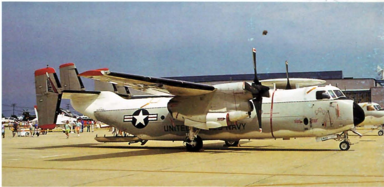
Above: With the Hawkeye in service a COD version was soon developed. This was much needed as the previous COD aircraft, the Trader, had piston engines and thus ran on petrol. No current carrier-based aircraft used this type of fuel and so ships stopped tanking it. The Trader was range-limited as it had to depart its shore base and fly to and from the carrier without being able to fill its tanks. The Greyhound, as the new aeroplane was called, was a much bigger airframe and could carry up to thirty-nine passengers. C2A Greyhound 162140 of the Naval Air Test Centre is seen at its Patuxent River, MD base, May 1989.
