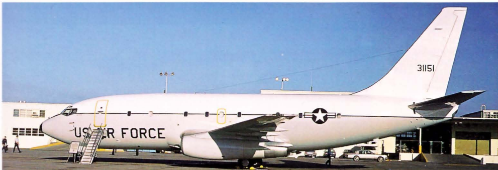
Below: Currently the best selling airliner in the world, in volume terms, is the Boeing 737. Military use is low. The USAF operates a navigator training aircraft based upon the 200 series. Inside are console stations for twelve trainees. T43A 73-1151 of the 323rd FTW, based at Mather AFB, CA, is at Travis AFB, CA, October 1979.
