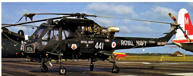
Below: Royal Navy use of the Wasp was as a light anti-submarine attack platform armed with homing torpedoes or depth charges. With a folding tail it flew from the rear decks of frigates. Wasp HAS1 XS452 441 of 829 Squadron is based on HMS Falmouth . It is seen at Valley, August 1973.
