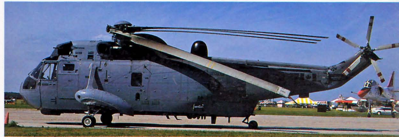
Below: Derived from the civil Sikorsky S62 the HH52 was operated by the US Coast Guard in an SAR role. Powered by a single 1250 shp GE T58 engine, the type was fully amphibious. HH52A 1400 from USCG Miami is at its Opa Locka base, October 1981.
