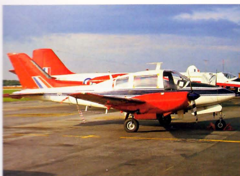
Left: The Beagle 206 was a British made 5/8-seat cabin monoplane powered by a pair of Rolls-Royce Continental piston engines. Twenty were built for the RAF as the Basset CC1 and they were used by a number of communications squadrons. XS770 was the last on charge being used by the A&AEE at Boscombe Down. It is pictured at Finningley, September 1984.
