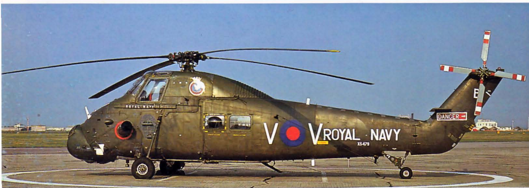
Above: Developed as an assault helicopter for the Royal Marines the Wessex HU5 could go into action with guns or wire-guided air-to-surface missiles. Wessex HU5 XS479 V/V of 848 Squadron, Royal Navy, is at Valley, August 1975. This unit was based on HMS Bulwark .
