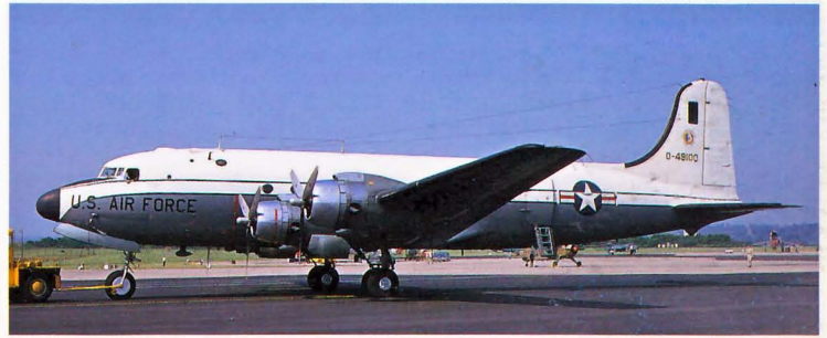
Below: The military variant of the Douglas DC4 Skymaster was the C54. It was used by the USAF in large numbers as a general transport aircraft. C54E 44-9100 is at Upper Heyford, June 1969. (SGW)
