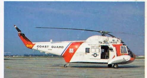
Below: Derived from the civil Sikorsky S62 the HH52 was operated by the US Coast Guard in an SAR role. Powered by a single 1250 shp GE T58 engine, the type was fully amphibious. HH52A 1400 from USCG Miami is at its Opa Locka base, October 1981.
