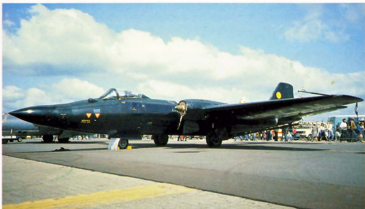
Below: Many Canberra airframes have been used as test vehicles. Canberra B2 (Mod) WV787 is used by the A&AEE for icing tests. It is seen at Greenham Common, June 1981
