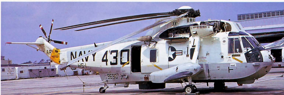
Below: Designed by Sikorsky the H3/S61 Sea King has been one of the most popular and widely used helicopters of all time. Seen at Jacksonville NAS, FL, in July 1974, is SH-3H 149690 430/AR of HS1. This variant was used by the US Navy for ASW operations. (SGW)
