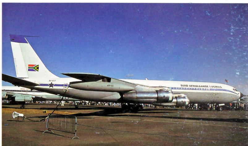
Above: South African Air Force Boeing 707-344 AF-617 is an ex-Air France aircraft. Now operated by 60 Squadron at Waterkloof it is an air tanker with a three-point hose and drogue system. It is pictured at Fairford, July 1995.
