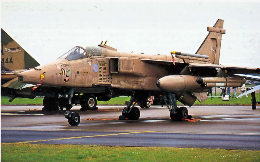
Below: Jaguar GR1A XX725 of GU/54 Squadron, RAF is at Scampton, July 1991. It is in desert camouflage and shows the missions flown in the Gulf War earlier that year. Note that for self-protection the Jaguar can carry air-to-air missiles above the wings.
