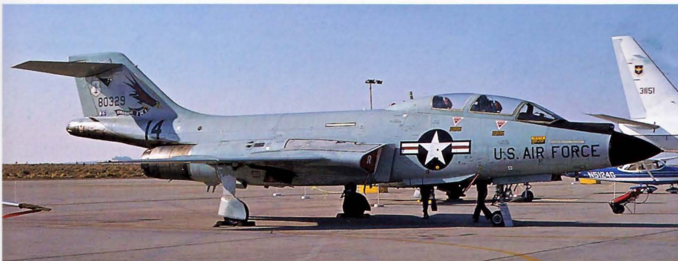
Below: Texas, the lone star state, operated F101F Voodoos . The 'F' variant was a reworked 'B' with an improved fire control and infra-red detection systems. These replaced the in-flight refuelling probe. 58-0276 is seen visiting Eglin AFB, Florida, in October 1981, and is operated by 111th Fighter Squadron, Texas ANG.
