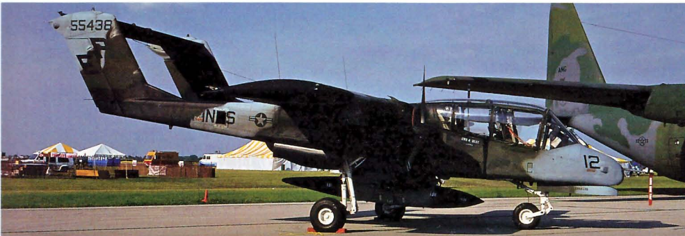
Below: Designed from scratch as a COIN (Counter Insurgency) aircraft the North American Rockwell OV10 Bronco has two seats in tandem and is used in light attack and forward air controller roles. 155438 OV10A ER/12 of VMO-1 'Yazoo' is seen at Hamilton, Ont, June 1990. The aircraft is based at the US Marine Corps station New River, NC.
