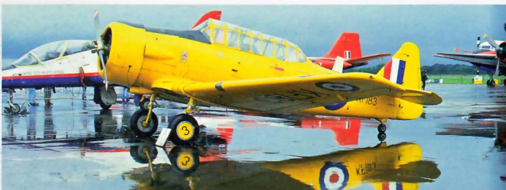
Above: The North American Harvard/Texan can claim to be the most important and perhaps widely used training aircraft ever. Powered by a single 550 hp P&W Wasp air-cooled radial engine it first entered service in 1938 and can still be found in service today. Two are used by the A&AEE at Boscombe Down as low-speed chase aircraft for trials. Harvard T2B KF183 basks in the type's reflected glory at Fairford, July 1987.
