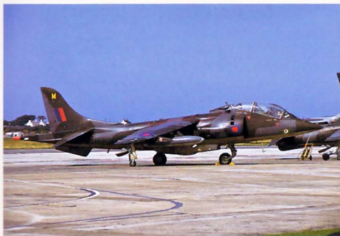
Below: Like a number of types the first Harrier pilots converted, in 1969, without the aid of a two-seater. The T2 was soon forthcoming the following year. XW926 M of 3 Squadron is at Valley in August 1973. It shows the extended nose and tall tail of the trainer.
