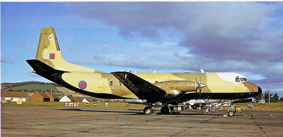
Left: The Andover C1 was a special military freighter. The entire rear end was redesigned to accommodate a rear-loading ramp that could open in flight to airdrop paratroopers or cargo. The undercarriage had a 'kneeling' facility to lower the loading ramp to floor level. Andover C1 XS612 of 46 Squadron RAF is at Leuchars, September 1974.
