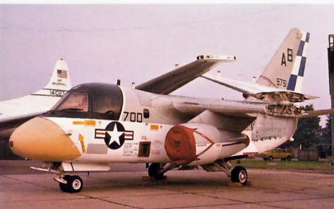
Above: Lockheed's S3 Viking was designed as a carrier-based anti-submarine warfare aircraft. It was a replacement for the piston-engined Grumman Tracker. S3A 159751 700/AB of VS32 'Maulers' is at Mildenhall, August 1978.
