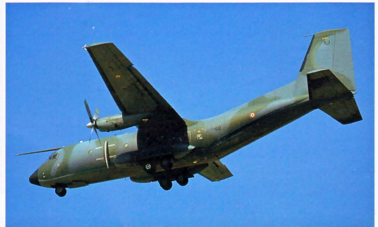
Above: In the late 1970s France decided it needed more aircraft and re-opened the Transall production line. Twenty-five more aircraft were built as C160NGs (New Generation). Extra fuel tanks were added as was an in-flight-refuelling capability. F217 64-GQ of French Air Force transport unit ET64 is seen landing at Athens, June 1993.
