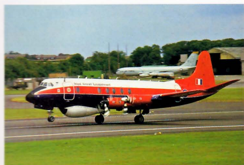
Left: Military use of the Vickers Viscount has been low. In the UK they have been used in small numbers as trials aircraft. Viscount 837 XT575 is from RAE Bedford and used as a radar test bed. Note the dish under the front fuselage. It is pictured at Fairford, July 1985.
