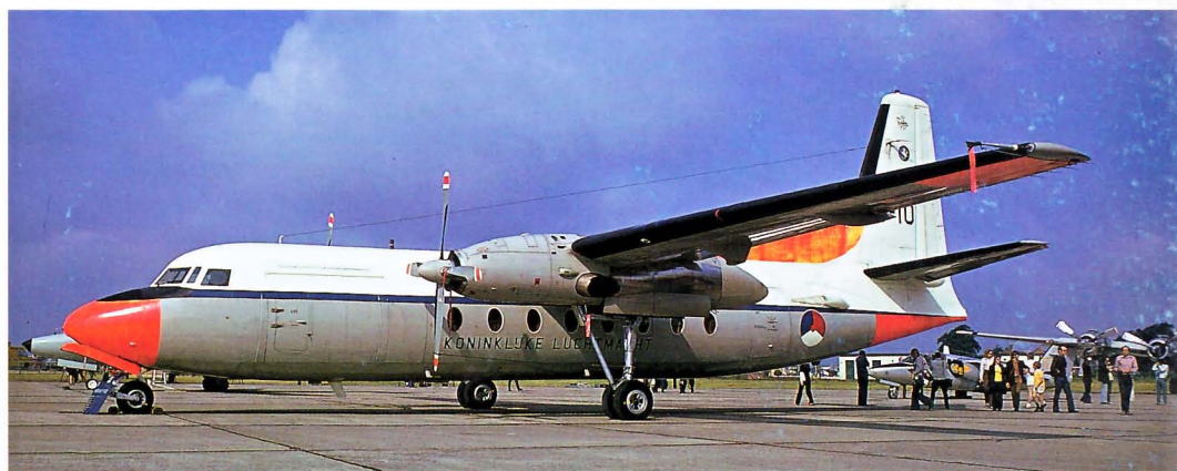
Below: As a follow-on to the F27, Fokker produced the F50; the military version of this is the F60 Utility. This is a stretched airframe (64 inches/1.62 m) with new generation P&W Canada PW125 turboprops. Fokker 60U U.04 of 334 Squadron, Royal Dutch Air Force, is at Fairford, July 1996.
