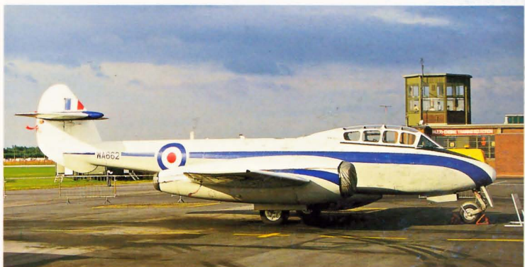
Above: The two-seat Meteor trainer was the T7 . It is of note that this aircraft did not have ejector seats. WA662 is operated by the RAE in this smart colour scheme. It is seen at Finningley, September 1984.
