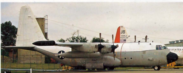
Below: The role of US Navy squadron VQ4 is known as TACAMO (Take Charge and Move Out). This involves communications with the fleet of ballistic missile submarines. The aircraft will trail a very long aerial and transmit in very low frequency. EC130Q 162312 of VX4 is at Patuxent River, MD, May 1989.
