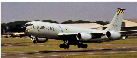
Above: Engine technology had evolved a great deal since the 1950s so in 1980 the USAF announced an upgrade in the KC135 powerplants. This involved fitting four CFM56 jets of 22,000 lb thrust; the original P&W J57 had 13,750 lb. KC135R 62-3554 of the 19th ARW departs Fairford, July 1989, showing the new, larger engines well.
