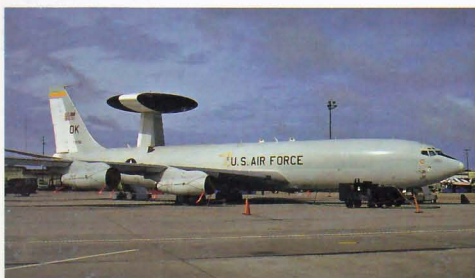
Below: The most distinctive Boeing 707 variant is the AWACS (Airborne Warning and Control System). The rotodome above the fuselage 30 ft (9.14 m) in diameter houses the radar set. E3B 77-0356/OK of the 522nd ACW is at Tyndall, FL, April 1994. American AWACS airframes do not have the big fan engines.
