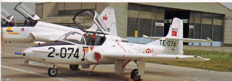
Below: Turkey is one of the countries to adopt the T37 as its basic trainer. T37B 88074/2.074 of 2 AJU is seen at its Cigu base, May 1998. The 'B' variant of the T37 had more powerful engines as well as improved navigation systems. All 'A' models were brought up to 'B' standard. (PJD)
