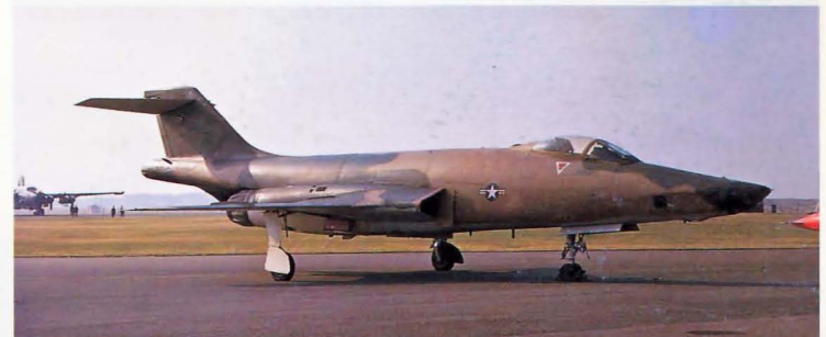
Below: A reconfigured nose shows this aircraft to be a photo reconnaissance version of the Voodoo. RF101C 56-0112 is operated by the 66th TRW, which was based at Upper Heyford during the period this picture was taken. It was photographed at RAF Valley in August 1968, in the camouflage colours worn at this time.
