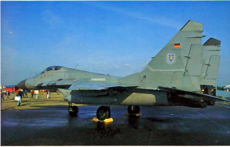
Above: NATO gave the reporting name Fulcrum to the MiG-29 . This aircraft is a relatively small interceptor with a very high performance from its two RD33 bypass turbofans. The output is 18,300 lb st (with afterburner/reheat). It was first seen in the west during a 1988 visit to Farnborough. However its secrets were laid bare when the East German air force was integrated into the Luftwaffe following the country's reunification. 29+14 of JG73 is seen at Mildenhall, May 1996.
