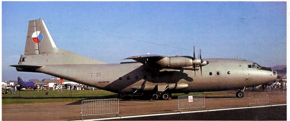
Above: The Warsaw Pact countries operated the Antonov An-12 in the same roles as the west did with the C130. Both aircraft have the same general layout of high wings, four turboprops and rear ramp loading. The An-12 had been developed from the earlier twin-engined An-8. An-12BP 2105 of 1 SDLP of the Czechoslovakian Air Force is at Boscombe Down, June 1992.
