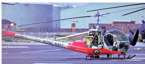
Above: Operated by 705 Squadron Fleet Air Arm for basic helicopter training, the Hiller HT2 served in this role from 1963 until 1975. A single 305 hp Lycoming piston engine powered it. XS162 is at Portland, August 1974.
