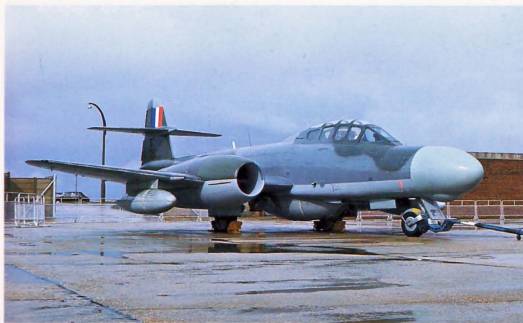
Below: Armstrong Whitworth Aircraft developed the Meteor TT20 from the NF11 night-fighter variant. The Royal Navy required a shore-based target tug to train gunners and guided missile operators. WM255 of the Fleet Requirement Unit is at its Hurn base, April 1968.
