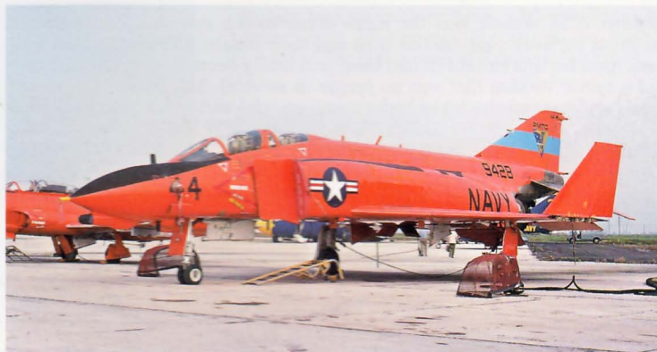
Above: The US Navy converted F4Bs into QF4B drones whilst the type was still in front-line service. 149428 is operated by the Pacific Missile Test Centre, Point Magu, CA where it was photographed in October 1976 in this high-visibility dayglo-orange colour. (SGW)
