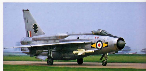
Above: To extend the range for ferry flights Lightnings could carry over-wing tanks. XP769 of J/11 Squadron is seen departing Binbrook, May 1972.
