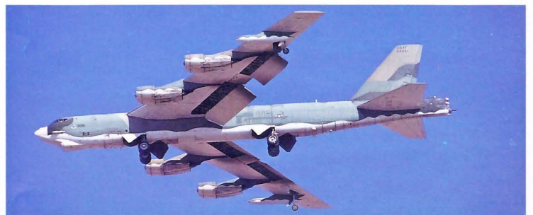
Above: The Boeing B52 Stratofortress was the big stick of SAC during the cold war. It has been in service since 1955 and is planned to be still operational in 2030, a staggering eighty-five years. B52H 60-0051 of the 93rd BW is in the circuit at its then base Castle AFB, CA in October 1979. The 'H' model was the eighth production variant; it had a shorter tail and TF33 turbofans.
