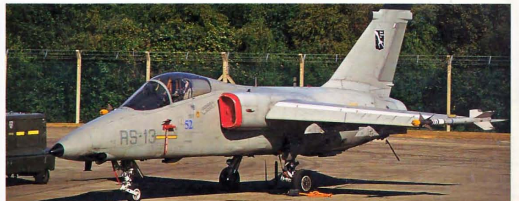
Above: The AMX is a joint venture between Italy and Brazil for a light strike and reconnaissance aircraft. It is powered by a single Rolls-Royce Spey turbofan. MM7131 RS-13/RSV is operated by the Italian Air Force test wing from its base at Pratica di Mare, near Rome. It is pictured at Fairford, July 1995.
