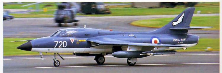
Above: XL603, photographed at Fairford in July 1985, is a Hunter T8M 720/899 of 899 Squadron. The T8 is the Fleet Air Arm variant of the T7 trainer. This special version features an extended nose with radar to train Sea Harrier pilots. 899 Squadron is the Royal Navy training unit for the Sea Harrier.
