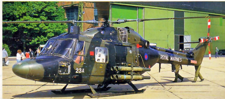
Above: Holder of the helicopter world speed record, the Westland Lynx is currently one of the best selling multi-role rotary-wing craft on the market. There are two main versions, the land and the shipboard. Lynx AH1 XZ182 23A of 3 CBAS Royal Marines is at Mildenhall, May 1986. Land variants up to the Mark 9 had skid undercarriages.
