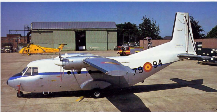
Below: Spanish built, the CASA 212 has found a market in the light transport role. A high-wing twin turboprop, it has as well as the traditional tasks been converted to other specialist military versions. TE.12B-41 79-94 of Ala 72 of the Spanish Air Force is at Boscombe Down, June 1992.
