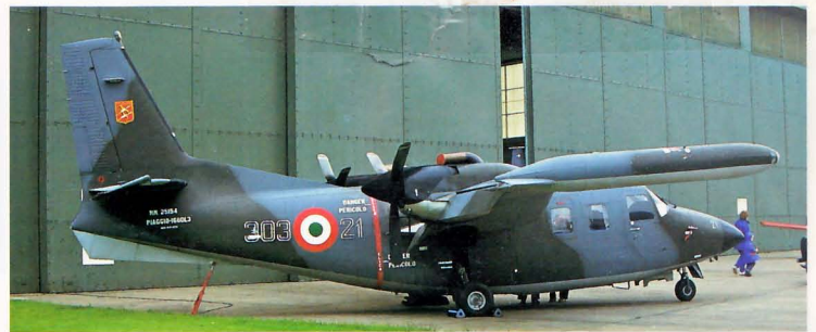
Below: The powerplants on the twin-engined Piaggio P166 are distinctive in that they act as pushers with the propellers being on the trailing edge of the wing. Italian-built, their role is communications between bases. A number are however configured for photo survey work and have vertical mounted cameras in the fuselage. Such an example is P166DL-3 MM25154 303-21 of 303 Gruppo. It is pictured at Cottone, June 1988.
