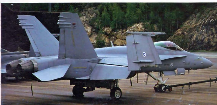
Below: Finland is in the process of assembling Hornets for delivery to its air force. F/A18C HN407 of HaLLv 21 was photographed at its Pirkkala base in June 1998. It is of note that the aircraft has its wings folded. This feature was designed as the US Navy needed this facility for carrier operations. Even though Finland does not operate such ships all aircraft have wing folding capabilities because it would have been more expensive to delete the feature.
