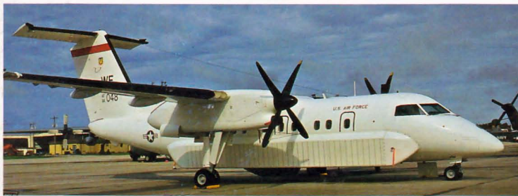
Above: Two de Havilland (Canada) DHC8 Dash 8s were converted for the USAF as range support aircraft. As can be seen in this picture the fuselage side has a fairing containing phased array radar. As well as this, telemetry equipment is fitted for the pilotless target jets flying in the range area off the Florida coast. E9A 84-0048/WE is operated by the 475th WEG from Tyndall AFB, FL, where it is pictured, April 1994.
