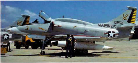
Above: The A4M was in fact called the Skyhawk II such was its level of upgrades. Most important was a new engine, the P&W J52-P408, which gave a 20% increase in thrust over earlier variants. 160252 3/VL of USMC squadron VMA 331 is seen at Pensacola, October 1981.
