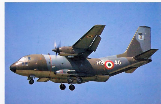
Below: The Alenia (Aeritalia/Fiat) G222 is a twin-turboprop high-wing transport. A variant was acquired by the USAF as the C27A Spartan. MM62128 RS-48 of the Italian Air Force RSV (Test Unit) is at Fairford, July 1989.
