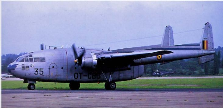
Above: The Fairchild C119 Flying Boxcar was a logical development from the company's earlier C82 Packet. It was a twin-boom tactical transport loaded from rear cargo doors. It was later used as a gun ship. CP35 is a Belgian Air Force C119G of 15 Wing. It is at North Weald, May 1972.
