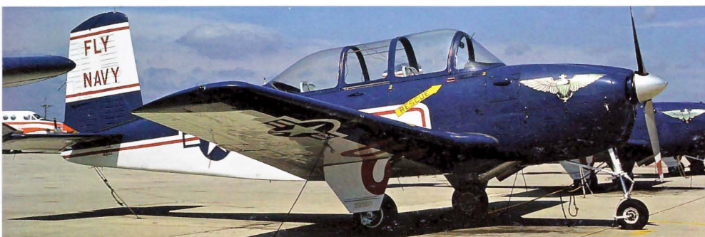
Left: The Beech T34B Mentor was a US Navy primary trainer powered by a 225 hp Continental piston engine. (The USAF had used the 'A' model.) Some 423 were delivered by 1957. 144044 is seen at Pensacola, October 1981 with 'Fly Navy' titles. This is one of many T34Bs used by Recruiting Command (part of Training Command). They are used to fly potential recruits to see if they have problems with flying such as airsickness before they get on to an expensive training syllabus.
