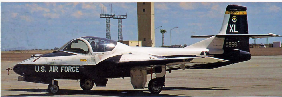
Above: The USAF entered the Cessna T37 basic jet side-by-side trainer into service in 1957. The aircraft is powered by two 1025 lb (465 kg) thrust Continental J69 turbojets. Seen on the ramp at Williams Gateway, AZ, in October 1998 is 58-1956/XL T37B of the 85th TFS/47th TFW from Laughlin AFB, TX.
