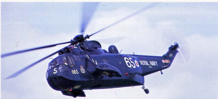
Above: Westland licence-build the Sea King and have out-sold their American counterpart. The Royal Navy is the largest UK user, ASW operations being the main role. Sea King HAS1 XV675 665/PO from 737 Squadron, a Portland-based training unit, is seen at Lee-on-Solent, July 1974.
