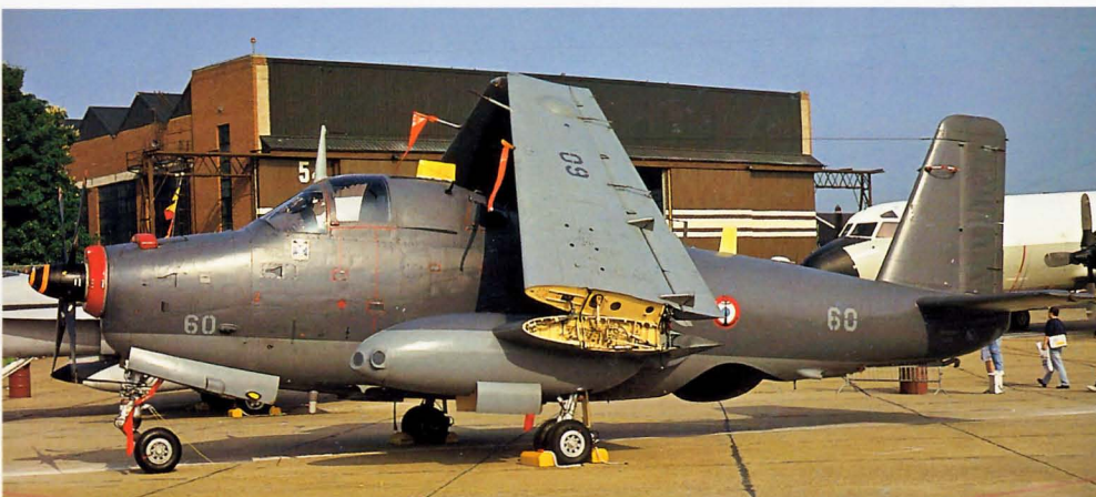
Below: One of the oldest designs currently flying off aircraft carriers is the Breguet BR1050 Alize . Operated by the French and Indian Navy, it is an ASW aircraft powered by a single Rolls-Royce Dart turboprop. No. 60 of 4F, French Navy, is seen at Mildenhall, May 1992.
