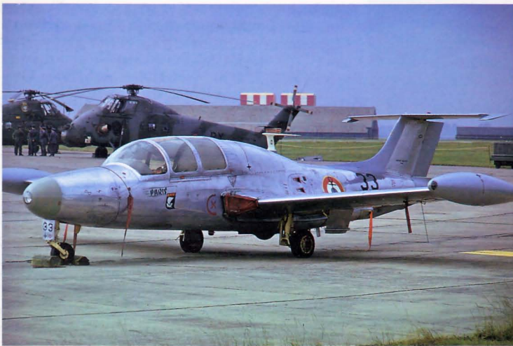
Above: Built by Morane-Saulnier, the MS760 Paris is a four-seat, twinjet liaison aircraft. The powerplants are a pair of 882 lb (400 kg) Turbomeca Marbore turbojets. No. 33/F-YETD is operated by the French Navy in a liaison role and is pictured at Greenham Common, July 1974.
