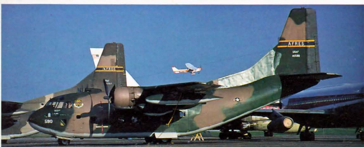
Below: Fairchild's C123 Provider was a twin piston-engined variant of the Chase C20 glider. The C123 had a rough field performance and was heavily involved in the Vietnam War. To give extra power some were converted to have a pair of 2850 lb thrust J85 jets under the wings, these were known as C123Ks. C123K 54-0580 of the US Air Force Reserve is at Harlingen, TX, October 1979.
