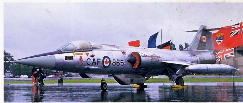
Below: Canadian Armed Forces (CAF) Starfighter CF104 104865 has a Vicon reconnaissance pod fitted to the underside of the fuselage. This could house up to four 70 mm Vinten cameras. It is seen on a very wet June day in 1971 at Upper Heyford in the early silver colour scheme.
