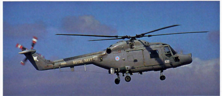
Above: This Navy Lynx is defined by a wheeled undercarriage. The type is used to operate off small ships and can carry a range of guns and missiles together with more and more improved avionics. Lynx HAS 3 ZD262 632/PO is operated by the then Portland-based 702 Training Squadron. It is pictured at Abingdon, September 1990.
