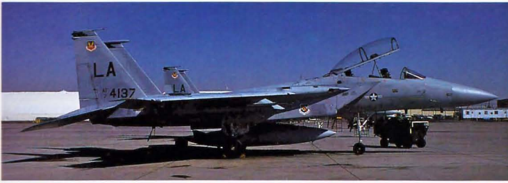
Left: The two-seat version of the F15A was the F15B . Fifty-seven were ordered. 74-0137 was photographed at LA/Luke AFB, its home with the 405th TFW, in October 1979.
