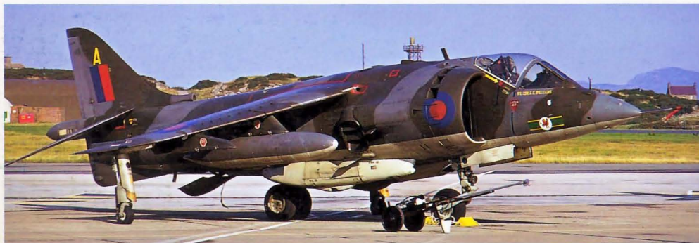
Above: The BAe Harrier serving today with the RAF can trace its roots from the Hawker P1127 VTOL research aircraft. The success of the type was to have engine nozzles that rotated from down for take-off to back for level flight. When the P1127 first flew in 1960 most other VTOL projects had two sets of engines, one for lift and the other for wing borne flight. This was impractical due to carrying the weight of engines not used in normal flight. The P1127 led to the Kestrel and then to the Harrier. Harrier GR1 XV741 of A/3 Squadron is seen at Valley, August 1973. This unit was part of 2nd TAF based in Germany.
