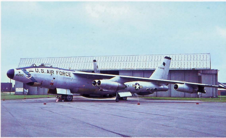
Above: The Boeing RB47H was an electronic reconnaissance variant of the original B47 six-engined bomber. 53-4280 is seen at Upper Heyford, May 1967. Note that the serial has the 'O' prefix. This was to indicate the aircraft was over ten years old. This procedure has since been dropped as the life of military aircraft has grown to figures that would not have been believed at one time. (AG)
