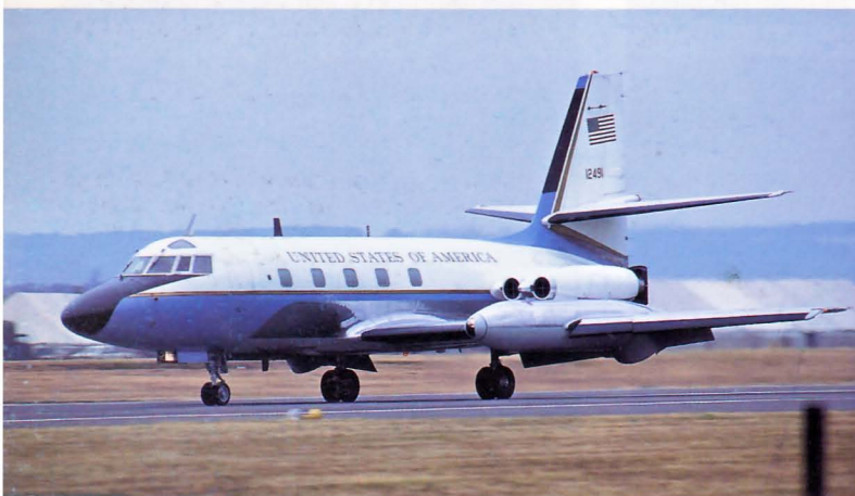
Above: First flown as a twin, production Lockheed Jetstars have four rear-mounted engines. The type is used for among other tasks the transport of VIPs. C140B 61-2491 of the 58th MAS is at Greenham Common, July 1983.
