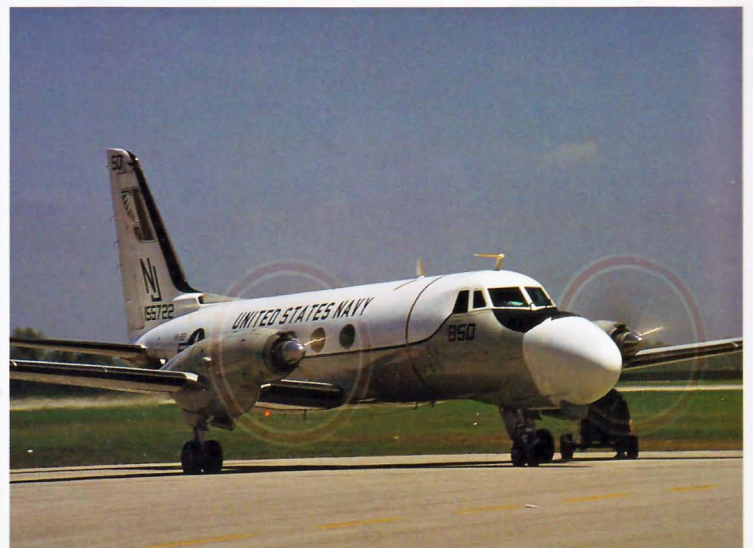
Below: The TC4C Academe is based upon the airframe of the Grumman G159 Gulfstream 1 twin-prop executive transport. This US Navy aircraft has a new nose into which is fitted the radar from the A6 Intruder. In the cabin there are locations for training the navigator/bombardier. 155722 850/NJ of VA128 is seen at London, Ont, June 1990.
