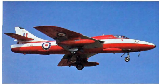
Above: Hunter T7 XL573 is seen at Finningley, September 1989. 12 Squadron, at the time a Buccaneer unit, operates this aircraft. The reason for the Hunter's presence was that there were no two-stick Buccaneers so each squadron had a Hunter converted to Buccaneer-style instruments in the left-hand seat. This eased the conversion to type process. Another use was to give pilots flight experience whilst the squadron's own aircraft were grounded.
