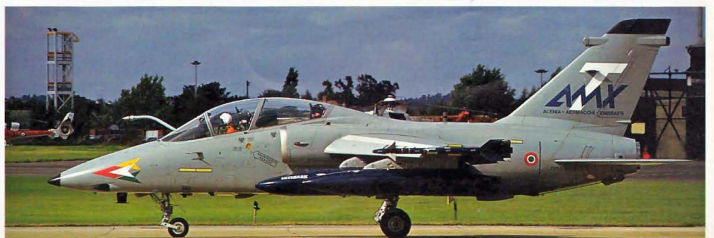
Above: The AMX is a joint venture between Italy and Brazil for a light strike and reconnaissance aircraft. It is powered by a single Rolls-Royce Spey turbofan. MM7131 RS-13/RSV is operated by the Italian Air Force test wing from its base at Pratica di Mare, near Rome. It is pictured at Fairford, July 1995.
