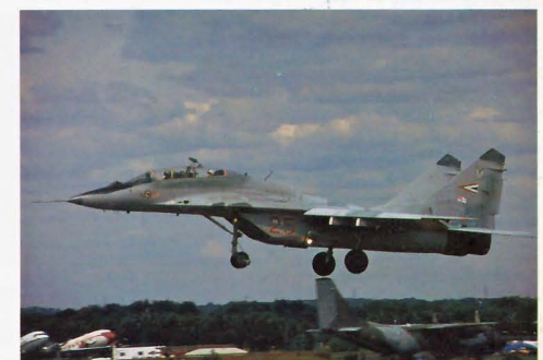
Below: Now a member of NATO, Hungary has left what was the 'Warsaw Pact' group as that alliance has now collapsed. Seen landing at Fairford in July 1998 was MiG-29UB 25(Red) of the 59th Tactical Fighter Regiment. Note the periscope above the rear seat cockpit.
