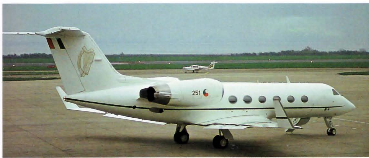
Above: Gulfstream stretched the G3 by 54 inches (1.37 m), changed the engines from the Rolls-Royce Spey to the Tay and called it the Gulfstream 4 . The Irish Air Corps operates a single example in a VIP role; 251 is seen at Liverpool-Speke, April 1993.
