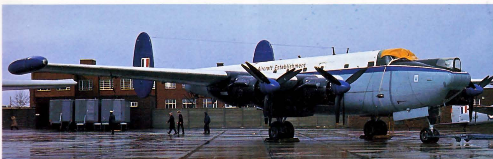
Above: Training for Shackleton crews was provided by the MOTU (Maritime Operational Training Unit) on the T4 model. This variant had the armament removed and additional radar positions for trainees. WB820 of S/MOTU is at Odiham, September 1964. (AG)
