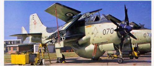
Below: First flown in 1949 the Fairey Gannet was a carrier-borne anti-submarine aircraft powered by a single Armstrong Siddeley Double Mamba turboprop. Training variants were the T2 and T5. Gannet T5 XG883 733/BY of 849 Squadron is seen at its base, RNAS Brawdy, August 1968.
