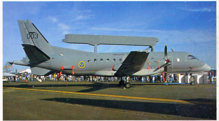
Above: Sweden has produced a complete AWACs package. This Swedish Air Force SAAB 340 has been mated with sideways-looking Ericsson airborne reconnaissance radar. Tp100 Argus 100003 of F16M from Malmsslatt is at Fairford, July 1998.
