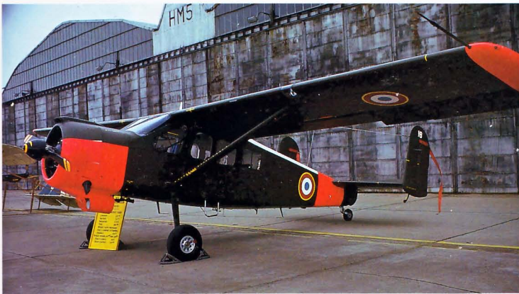
Below: With the same powerplant and a similar size and layout, except for the twin tail fins, the Max Holste MH1512M Broussard was the French equivalent of the Beaver. No. 18 is seen at Châteaudun, June 1977.
