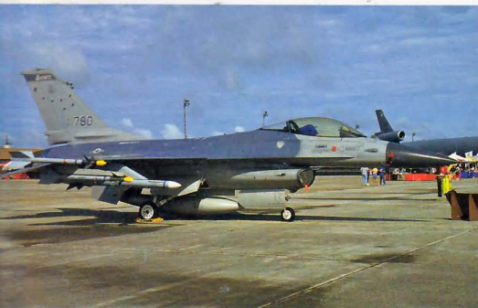
Above: The Minnesota ANG's 179th FS is an air defence unit. Note the bulge at the base of the fin and the aerial array in front of the cockpit. F16A 81-0780 is at Tyndall AFB, FL, April 1994. The stars on the fin are a representation of the constellation 'Little Dipper'.
