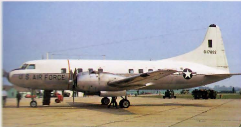
Above: Ordered first as a navigation trainer and then as a transport the T29 was based upon the civil Convair 240. T29B 51-7892 is operated by 513rd TAW at Mildenhall as a general hack. It is pictured at Bentwaters, May 1972.
