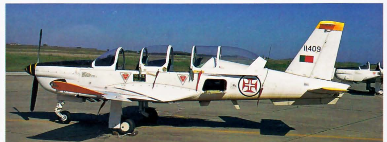
Above: The light aircraft subsidiary of Aerospatiale (SOCATA) designed the TB30 Epsilon trainer to have the layout of instruments and handling characteristics of the Alpha Jet. This plan would ease the pilot from basic to advanced trainer as painlessly as possible. As well as French use it has been sold to the Portuguese Air Force, which had the airframes assembled in country by OGMA. 11409 of Esq 101 is seen at its Beja base, March 1997. (PJD)
