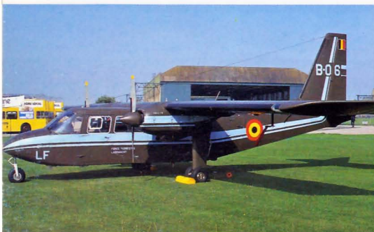
Above: A general-purpose light transport of very rugged construction the Britten-Norman Islander has found many military customers. As well as a multi-role liaison aircraft it can be configured with underwing hard points for attack duties or with a nose radar for maritime patrol. BN2A Islander B-06 of the Belgian Army is at Middle Wallop, July 1982.
