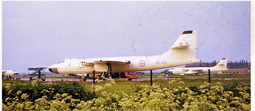
Above: The Vickers Valiant was the first of the three 'V' bombers in service, and due to metal fatigue in the main spar, was the first to be retired. Valiant B(PR)K1 WZ392 of 543 Squadron was seen at its Wyton base in May 1964, along with two others. (AG)
