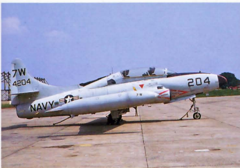
Above: The US Navy variant of the T33 was the TV2 . As can be seen, the area behind the cockpit is quite different. The aircraft is also equipped with a tail hook. 144204 7W is the base flight aircraft at Willow Grove, August 1970. (SGW)
