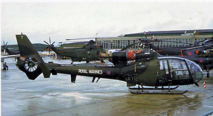
Below: The main task of the Gazelle is observation, but Royal Marines operations have included machine-guns and air-to-ground unguided rockets fired from out-rigger pods. Gazelle AH1 XX412/Y 3 CBAS RM is at Yeovilton, August 1984.
