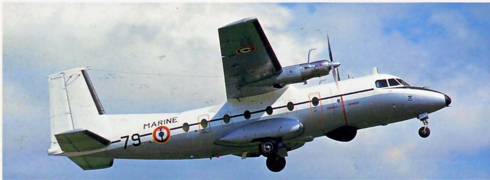
Below: Developed from the earlier Nord 260 the 262 Fregate is a twin-engine, high-wing light transport. It sold in both civil and military markets. No. 79 of 2S, French Navy, is seen departing Fairford, July 1985.
