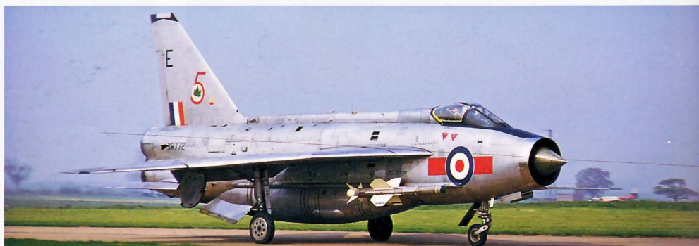
Below: The first unit to get the definitive Lightning was 5 Squadron at Binbrook. This was the F6 and had the larger ventral fuel tank. XR772, E/5 Squadron is seen departing its base, May 1972.
