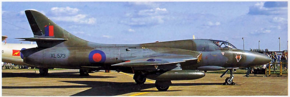
Above: Hunter T7 XL573 is seen at Finningley, September 1989. 12 Squadron, at the time a Buccaneer unit, operates this aircraft. The reason for the Hunter's presence was that there were no two-stick Buccaneers so each squadron had a Hunter converted to Buccaneer-style instruments in the left-hand seat. This eased the conversion to type process. Another use was to give pilots flight experience whilst the squadron's own aircraft were grounded.
