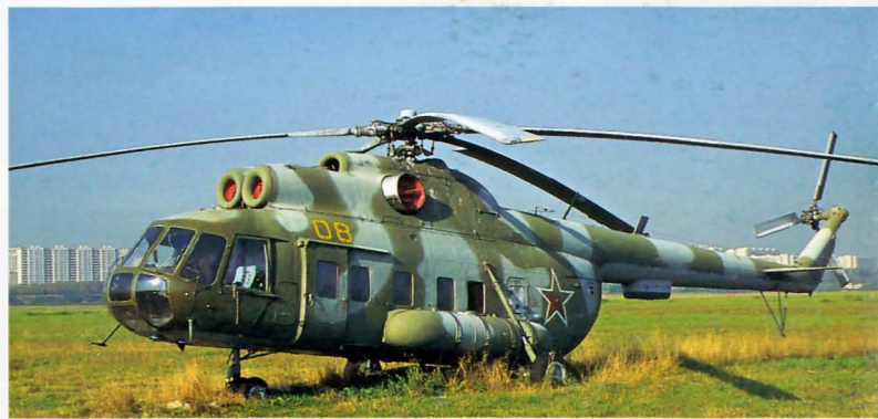
Below: With the Mi-8 being built in vast numbers there are lots of upgrades and sub types. 08(Yellow) of the Russian Air Force is at Tushino, August 1995. This is a Hip-C with five rotor blades.
