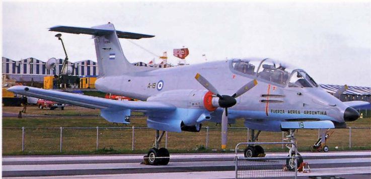
Above: The FMA IA-58 Pucara is an Argentine designed and built twin turboprop light attack and close support aircraft. As well as guns it has four wing hard points and one under the fuselage. A-19 of the Argentine Air Force is at Farnborough, September 1978.
