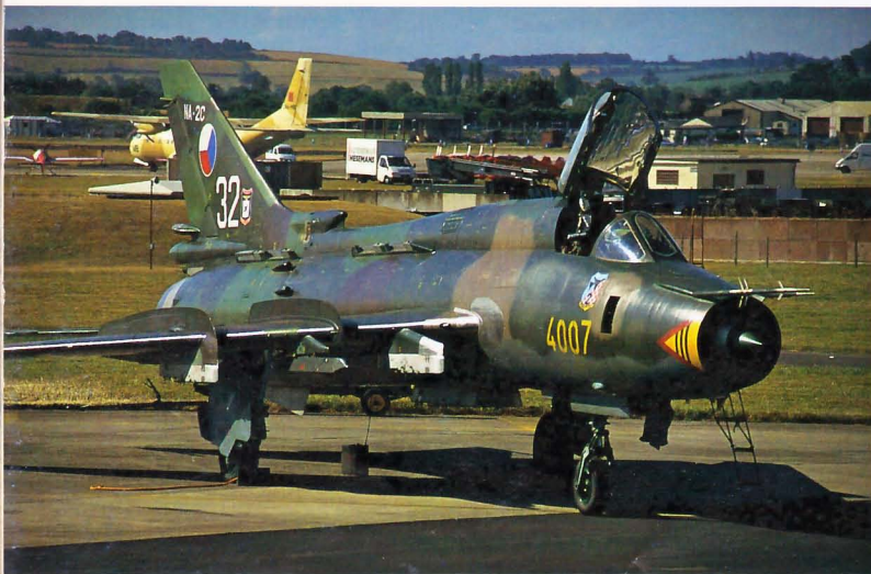
Above: NATO gave the code-name 'Fitter' to the range of Sukhoi ground attack fighters starting with the Su-7. The final 'Fitter' variant is the Su-22M-4 . The quickest recognition point is the ram air inlet at the base of the tail fin. 4007 (Fitter K) code 32 of 32ZTL Czech Air Force is at Fairford, July 1995.
