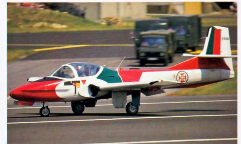
Above: The 'C' model of the T37 has provision for both tip tanks, for extra fuel, and to be able to carry weapons. T37C 2406 of the Portuguese Air Force aerobatic team 'Asas de Portugal' is at Fairford, July 1989.
