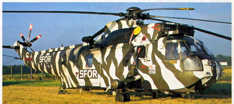
Above: The Sea King HC4 is configured for commando operations with the Royal Marines. It has seats for twenty-eight troops together with floor armour. ZD477/Y of 845 Squadron, Royal Navy, is seen in SFOR marking at Fairford, July 1997.
