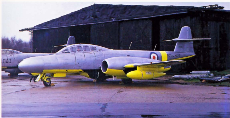
Below: Armstrong Whitworth Aircraft developed the Meteor TT20 from the NF11 night-fighter variant. The Royal Navy required a shore-based target tug to train gunners and guided missile operators. WM255 of the Fleet Requirement Unit is at its Hurn base, April 1968.
