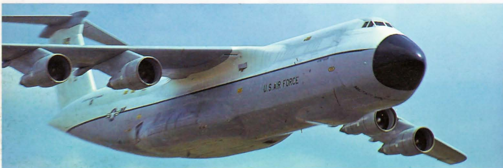
Above: The Lockheed C5A Galaxy is well known for its vast size. It is a four-engined high-wing strategic transport with a capacity for up to 350 troops or 265,000 lb of cargo. 69-0019 of the 436th MAW departs Greenham Common in the original white and grey colours, June 1981.
