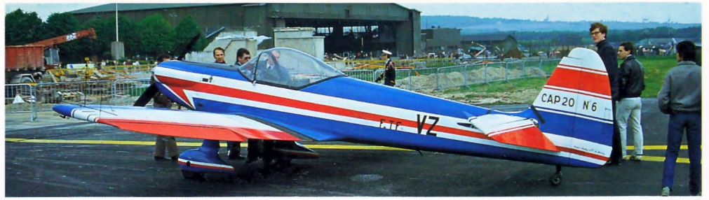
Above: The Mudry CAP 20 is a single-seat aerobatic aircraft. Designed for +8 and -6 G, it was acquired in small numbers by the French Air Force for aerobatic practice. No. 6/VZ is at Reims, May 1983.
