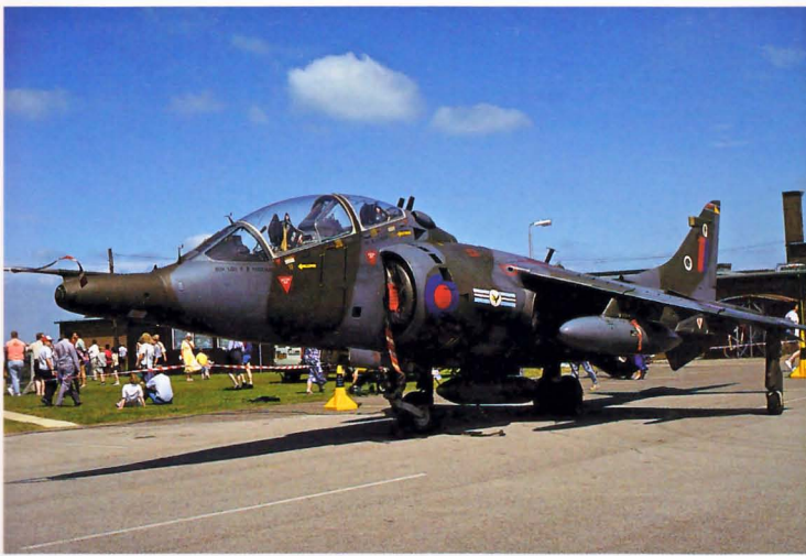
Above: This two-seater is the second variant of the Harrier trainer and is designated T4 . ZD990 Q of 20 Squadron is at Cottesmore, July 1993.
