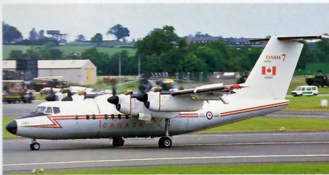
Above: Following the company trend of STOL aircraft de Havilland (Canada) produced the DHC7 Dash 7 . This was a four-engine fifty-seat aircraft. It was used for some years by the Canadian Armed Forces under the designation CC132 . 132001 of 412 Squadron arrived at Fairford in July 1985 in what was then a standard colour scheme for Canadian transport aircraft.
