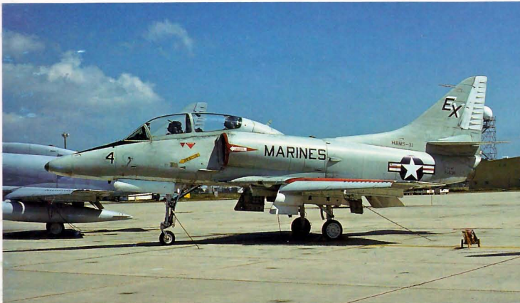
Above: Ten years after the A4 entered service the two-seat TA4F followed. As well as being a trainer it could also carry weapons and was used as a forward air controller (Fast FAC) with the USMC. 154311 4/EX is operated by H&MS 31. This is a Marine Corps HQ and Maintenance squadron. It is pictured at Pensacola, October 1981.
