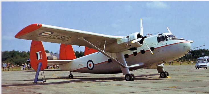
Left: The Beagle 206 was a British made 5/8-seat cabin monoplane powered by a pair of Rolls-Royce Continental piston engines. Twenty were built for the RAF as the Basset CC1 and they were used by a number of communications squadrons. XS770 was the last on charge being used by the A&AEE at Boscombe Down. It is pictured at Finningley, September 1984.
