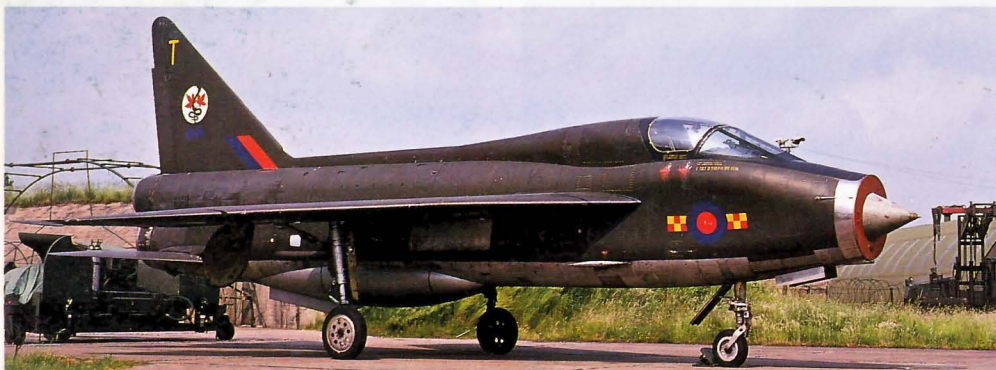
Below: To train F3/F6 pilots the two-seater used was the T5 ; this had the clipped fin top of these two variants. XS419 of T/23 Squadron is at the unit's base Leuchars, September 1975.
