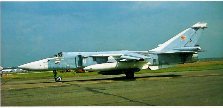
Left: The Sukhoi Su-24 (NATO code-name Fencer ) is a long-range low-level Russian attack bomber. With swing-wings and a top speed of Mach 1.35 it is a very formidable warplane. 11(White) was photographed at the Zhukovsky test airfield near Moscow in August 1997. (JDS)
