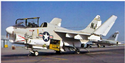
Above: The conversion trainer for the Corsair II was the TA7C. These were converted 'B' & 'C' models. Showing the two cockpits open is 156795 204/NJ of VA122 (USS Lexington), at Lemoore, CA, October 1979.
