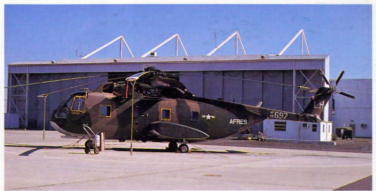
Below: Sikorsky CH3E 65-5697/LH is operated by 302nd SOS AFres at Luke AFB, AZ, October 1979. The H3 was a USAF variant of the SH3 with major design changes including a rear loading door and new undercarriage.
