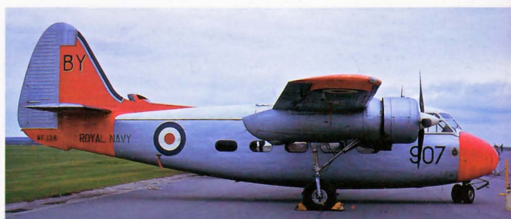
Below: Three years before the RAF had the Pembroke the Royal Navy had received the first Sea Prince. The role of the type was as a light transport; later versions were used as navigation trainers. Sea Prince C1 WF138 907/BY is an early short-nosed variant. It is operated as the station hack at RNAS Brawdy where it was photographed in July 1963. (AG)
