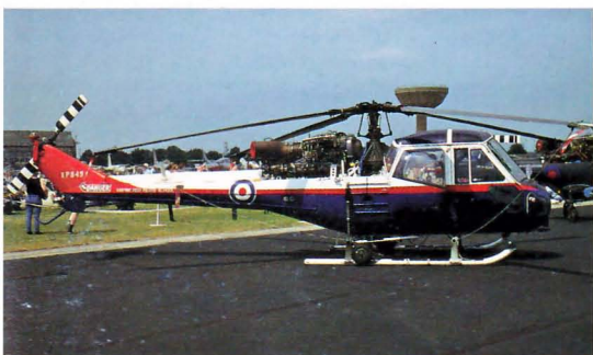
Above: Westland developed two helicopters side by side; they were the Scout for the Army and the Wasp for the Navy. Both were basically the same and were identified as 'A Wasp has wheels and a Scout has skids'. The Army Air Corps used the Scout as a general-purpose helicopter with the capability for firing anti-tank rockets. Scout AH1 XP849 was passed on to the ETPS for test pilot training. It is pictured at Yeovilton, July 1994.
