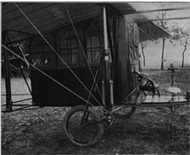
The first 'Aerial Limousine', 1911. "The limousine has doors with mica windows and seats for four persons fitted with pneumatic cushions, the pilot seats in front. A number of flights have been made, with and without passengers, with entire success."
