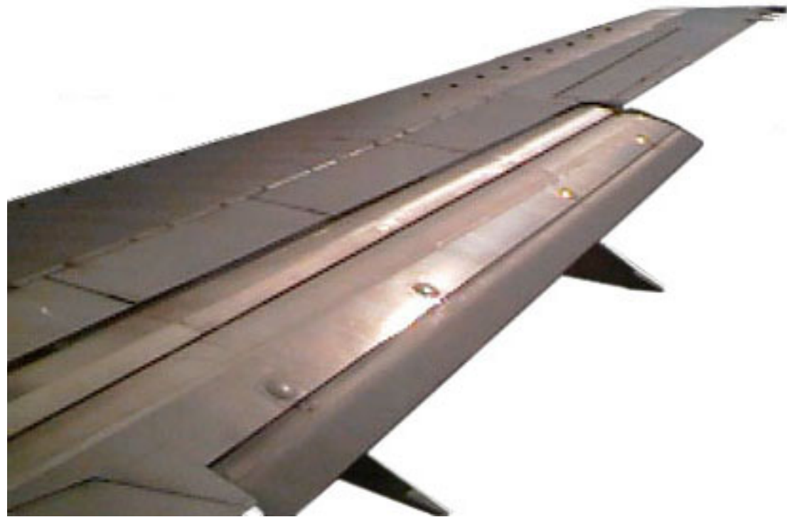
Figure 2. The triple-slotted flap system used on a 737.
