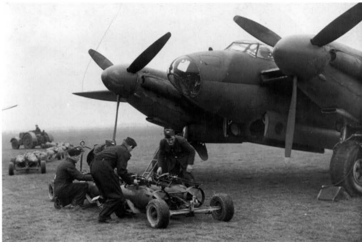
Armourers prepare to load 500 lb (226 kg) bombs. To enable four of these bombs to fit into the Mosquito's bomb bay, a bomb with shortened vanes was developed and underwent successful test drops from the Mosquito B.V, W4057. This was soon adopted as standard for bomber versions of the Mosquito. (via Phil Jarrett)
