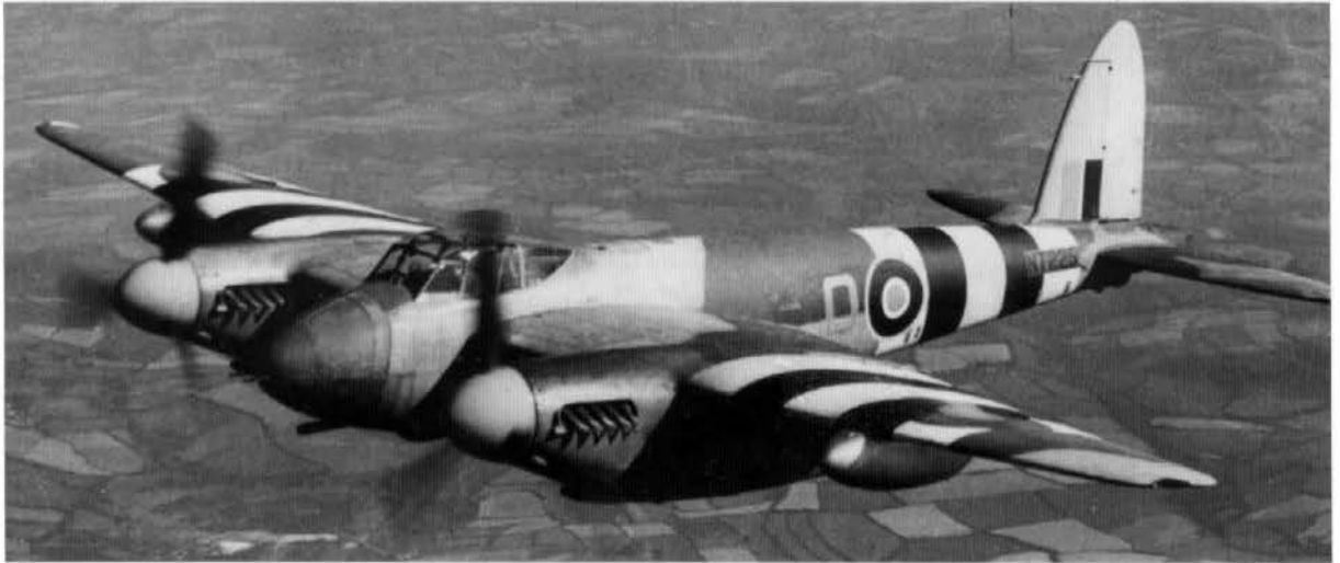
A 'Tsetse' Mosquito FB.XVIII of No 248 Squadron wearing 'invasion' stripes. The Mk.XVIII's, with their powerful 57 mm guns, proved effective against coastal craft and submarines operating in the Biscay area. (via Phil Jarrett)
