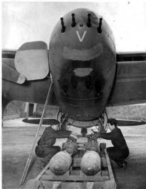
Armourers loading a clutch of four short-vane 500 lb (227 kg) bombs into a Mosquito FB.Mk.VI. The shortened vanes did not affect the bombs' stability, as had been feared. (via Phil Jarrett)
