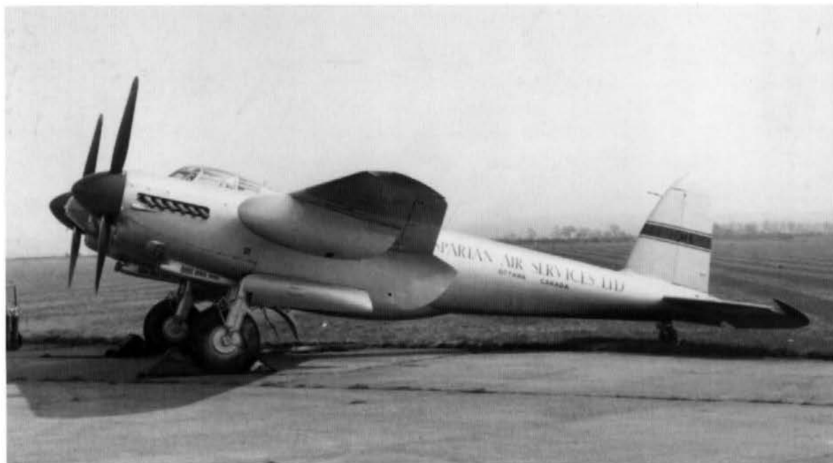
Above and below: Two of the ten Mosquito B.35s refurbished by Derby Aviation Ltd for Spartan Air Services of Ottawa. They were fitted with new transparent noses, and camera stations forward and aft of the bomb bay. (via Phil Jarrett)
