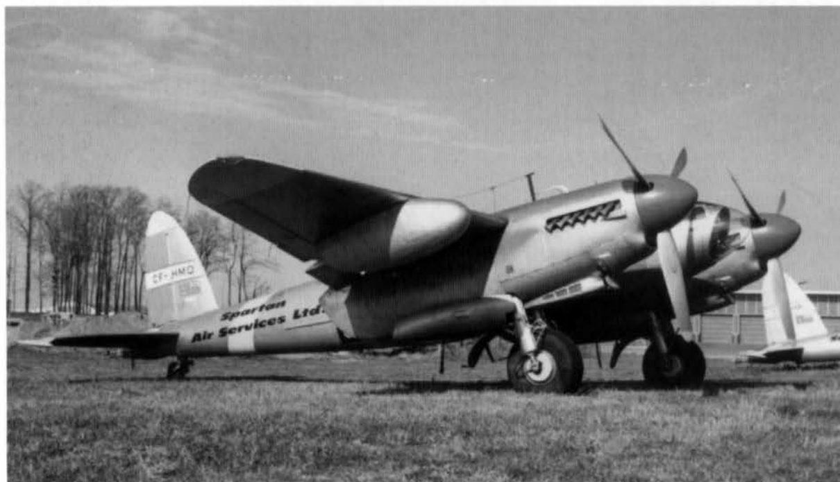
Above and below: Two of the ten Mosquito B.35s refurbished by Derby Aviation Ltd for Spartan Air Services of Ottawa. They were fitted with new transparent noses, and camera stations forward and aft of the bomb bay. (via Phil Jarrett)
