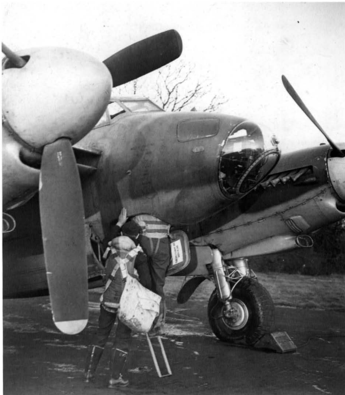
Bomber and PR versions of the Mosquito had an under-fuselage escape hatch; in the fighter-bomber variants this was in the starboard side of the nose, the position of the nose armament ruling out an under-fuselage exit point. Whichever configuration was used, the Mosquito was not an easy aircraft from which to escape. (via Phil Jarrett )
