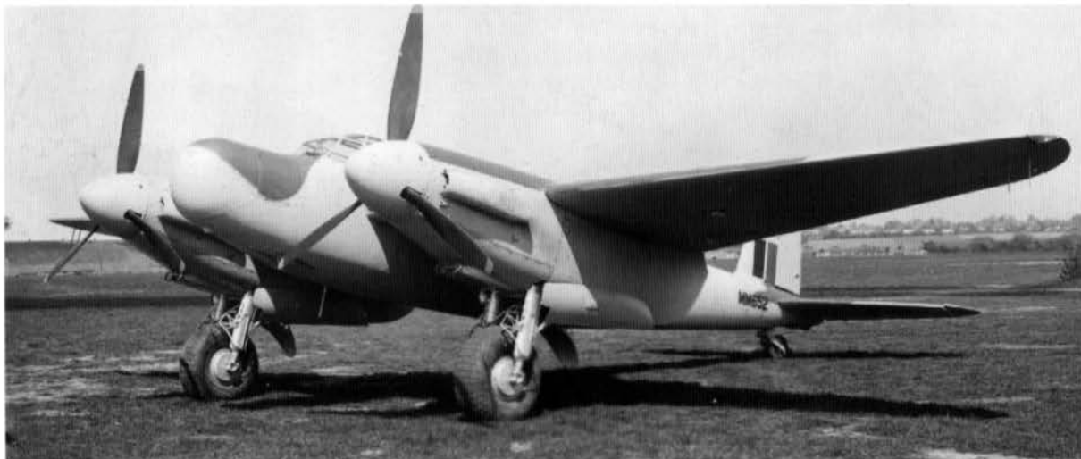
Mosquito NF.Mk.XIX MM632. This variant was equipped with the Merlin 25 engine and X/SCR720/729 radar in a 'thimble' or Universal Nose. It could reach 378 mph (608 km/h) at 13,000 ft (3965 m) with an operational load. It flew for the first time in April 1944. (via Phil Jarrett)
