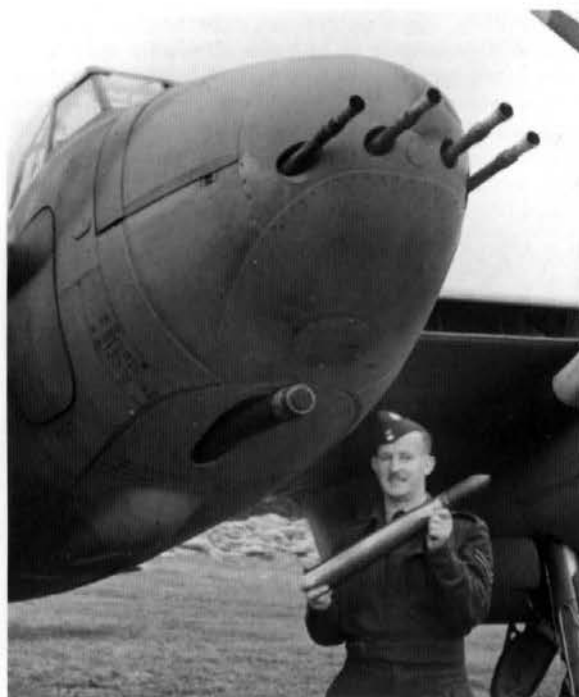
An armorer displays the 57 mm 6-pounder shell that was the primary armament of the Mosquito Mk.XVIII 'Tsetse' ground attack and anti-shipping fighter. The 57 mm gun weight 1580 lb (715 kg). The four 0.303 in (7.7 mm) machine guns were retained, and eight 60 lb rocket projectiles could also be carried. (via Phil Jarrett)
