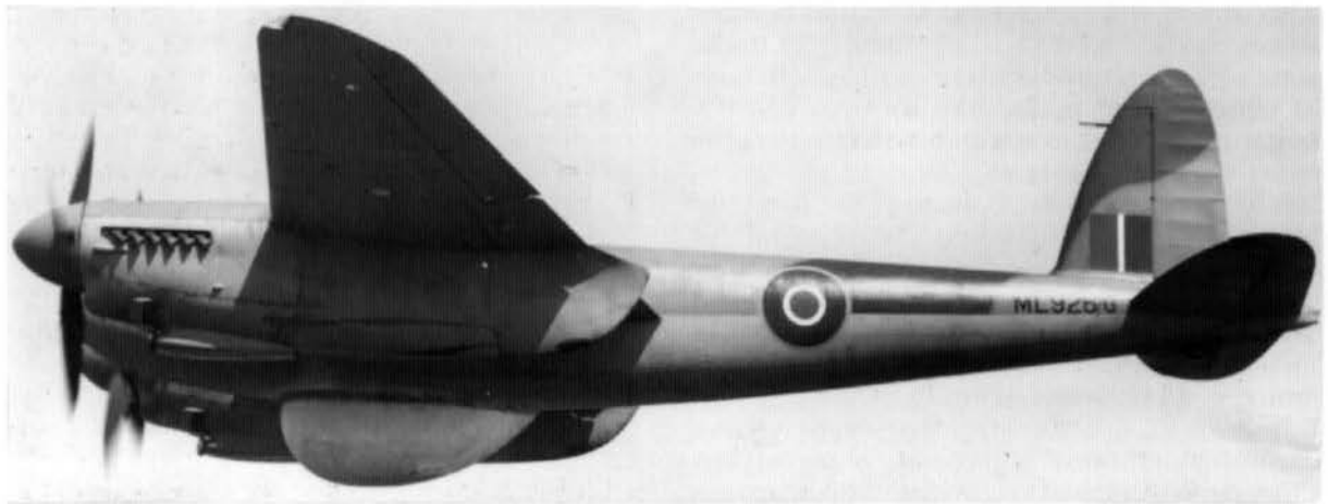
A Mosquito Mk.XVI with H2S radar equipment in the bomb bay. The Pathfinder Mk.XVIs carried a wide variety of electronic equipment, including Oboe , Boozer , Monica , Fishpond and Album Leaf . The Mk.XVI Mosquito flew for the first time on New Year's Day, 1944. (via Phil Jarrett)
