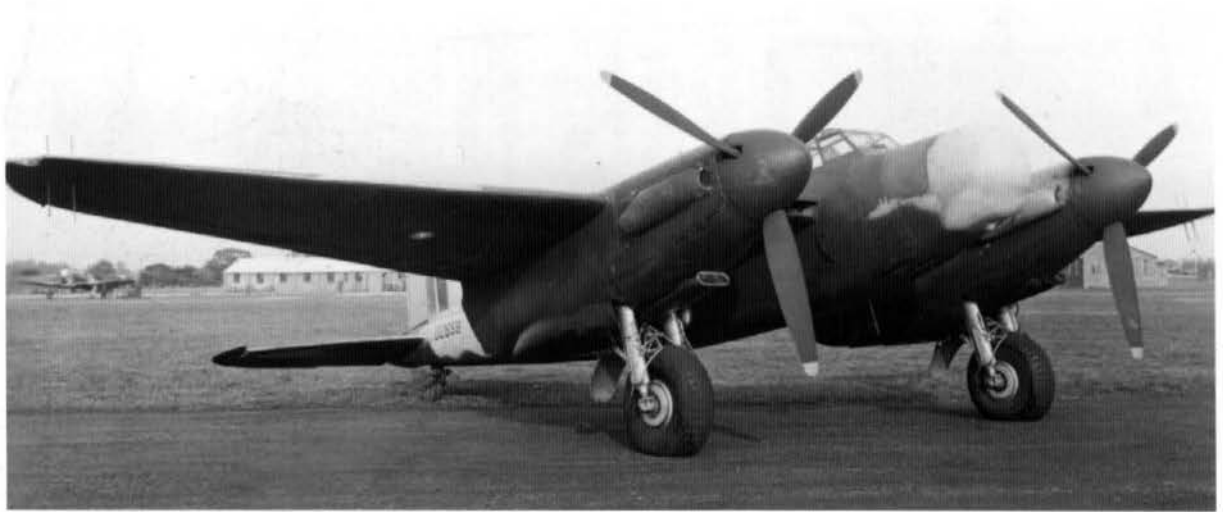
Mosquito NF.Mk.XVII DZ659 pictured in October 1944. This night-fighter variant was equipped with the greatly improved AI.Mk.X radar and flew for the first time in March 1943. AI.Mk.X was the British designation for the American SCR720 centimetric radar. (via Phil Jarrett)
