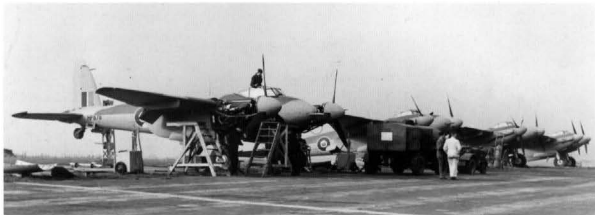
The finishing touches being applied to Mosquito FB.VIs at the Standard Motor Company's Coventry factory. These aircraft were part of a batch of 500 produced between June 1943 and December 1944; many were destined for service overseas. (via Phil Jarrett)
