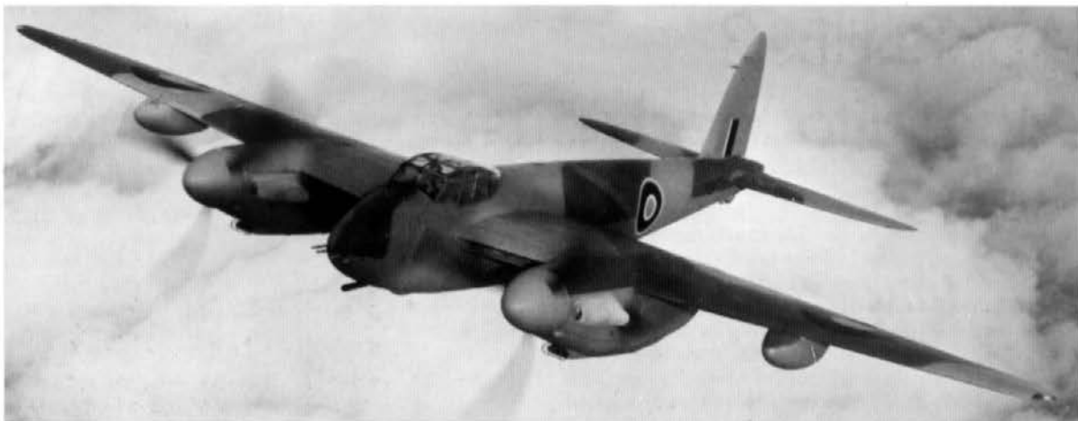
A view of PZ487, a trials Mosquito FB.Mk.XVIII 'Tsetse', armed with a nose-mounted Molins 6-pounder 57 mm gun for anti-shipping and ground attack. The weapon fired 25 rounds in 20 seconds, but rocket projectiles were much more effective. Only 18 production FB.XVllls served with Nos 248 and 254 Squadrons. (via Phil Jarrett)
