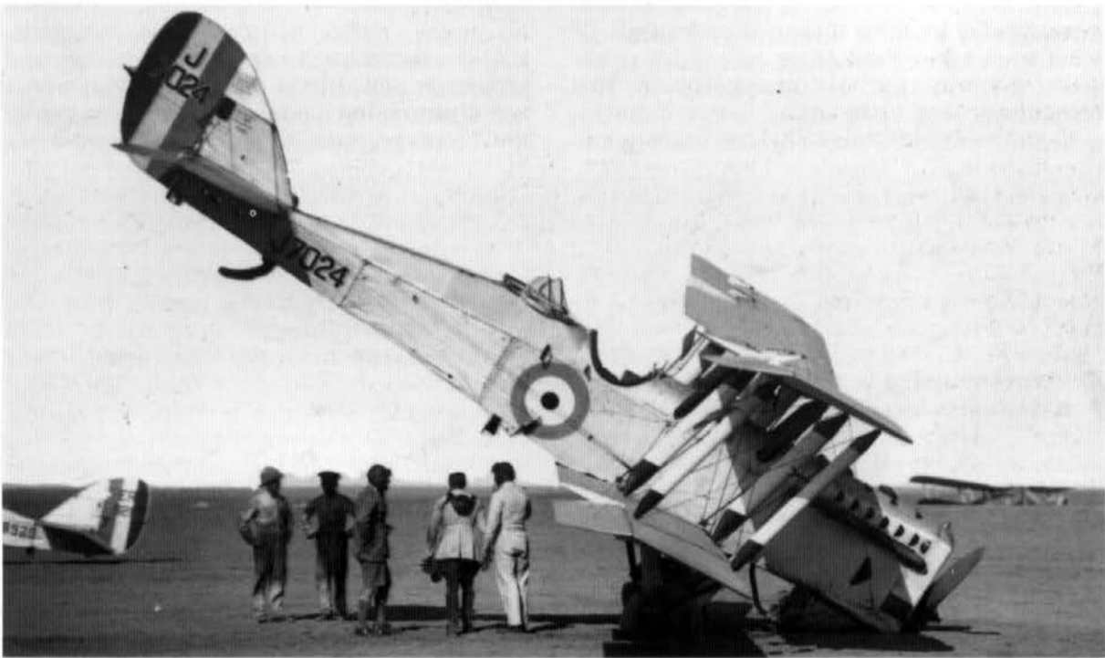
De Havilland's DH9 bomber design was less successful than the DH4, which it was intended to replace. Underpowered and accident-prone, it nevertheless played a major part in policing the trouble spots of the British Empire during the 1920s. This example came to grief in Iraq. (via author)
