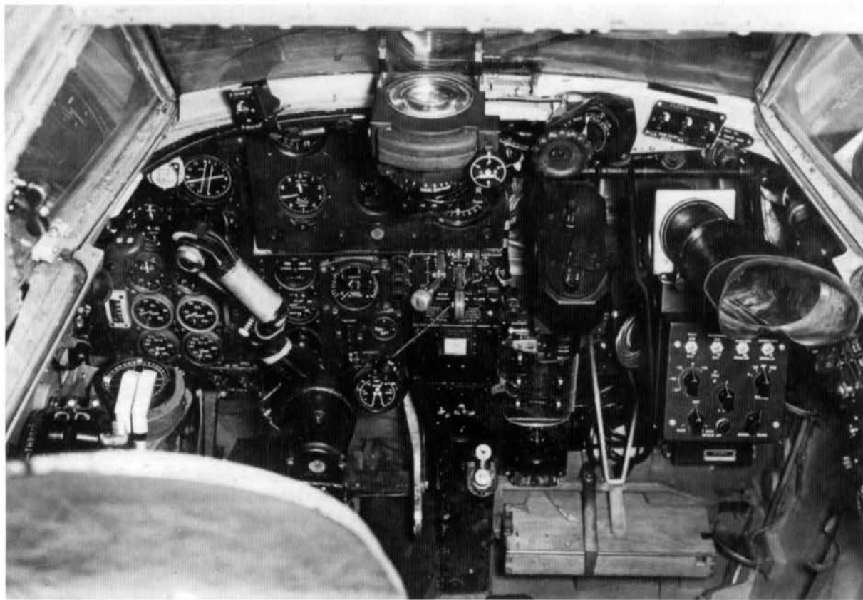
The cockpit layout of a Mosquito NF.II, showing the observer's AI Mk.IV installation and cathode ray tube (CRT) on the right-hand side. Positioning the radar operator alongside the pilot and not at a remote location in the fuselage greatly improved the teamwork which was vital for a successful AI interception. (via Phil Jarrett)
