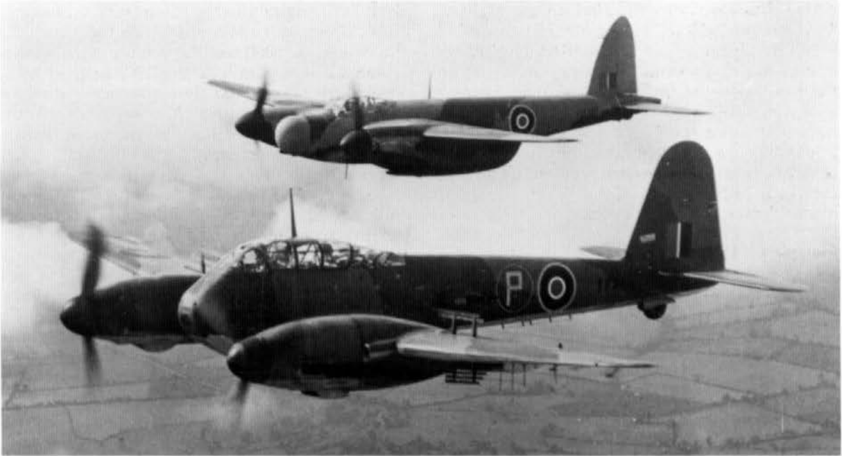
A Mosquito XVII flies in formation with a captured Messerschmitt Me 410, one of its main opponents during the so-called 'Little Blitz' of early 1944. The Me 410s approached the British Isles at high altitude, then made fast diving attacks on their targets. They also carried out low-level intruder operations. (via Phil Jarrett)
