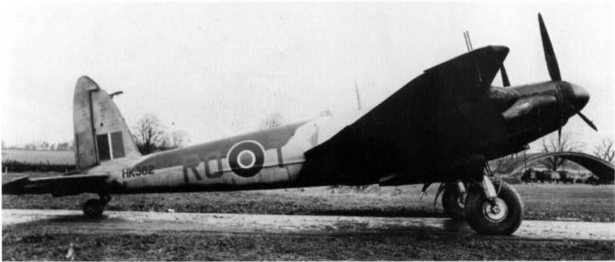
Mosquito NF.Mk.XIII HK382 of No 29 Squadron seen at Hunsdon, Hertfordshire, in January 1945. The aircraft is fitted with long-range tanks for intruder operations. The first NF.XIII flew in August 1943; No 29 Squadron re-equipped with the mark in October that year and used it until February 1945. (via Phil Jarrett)
