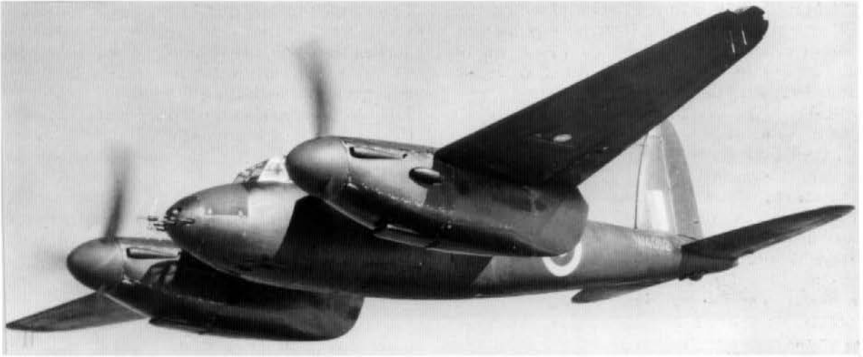
The Mosquito fighter prototype, W4052, seen during trials at the A&AEE in October 1941. The aircraft was finished matt black overall. Note the AI.Mk.IV radar aerials under the port wingtip. (via Phil Jarrett)
