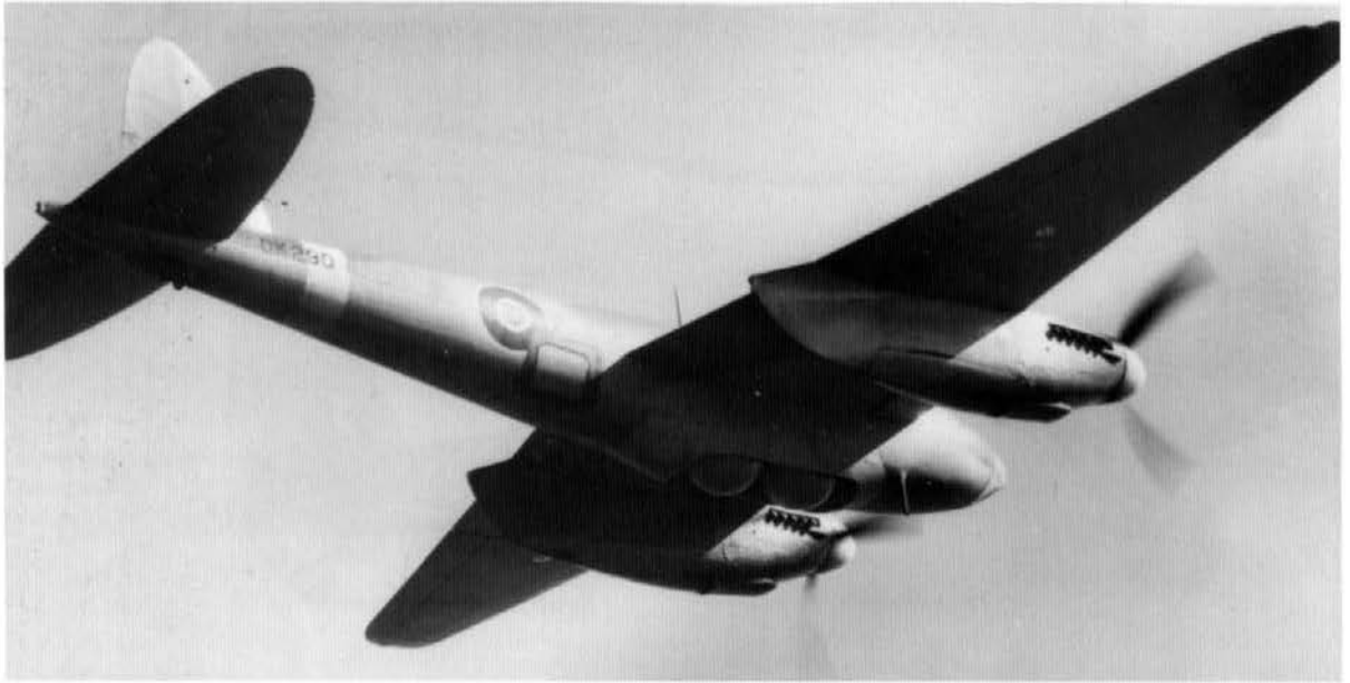
Mosquito B.IV DK290, with bomb-bay modified to accommodate two 'Highball' anti-shiping weapons. Intended for use against enemy capital ships such as the Tirpitz , Highball was deployed to the Pacific with No 618 Squadron. Difficulties arose from the fact that the operational area was under US Navy control. In any case, nearly every major Japanese warship had been sunk by April 1945. (via Phil Jarrett)
