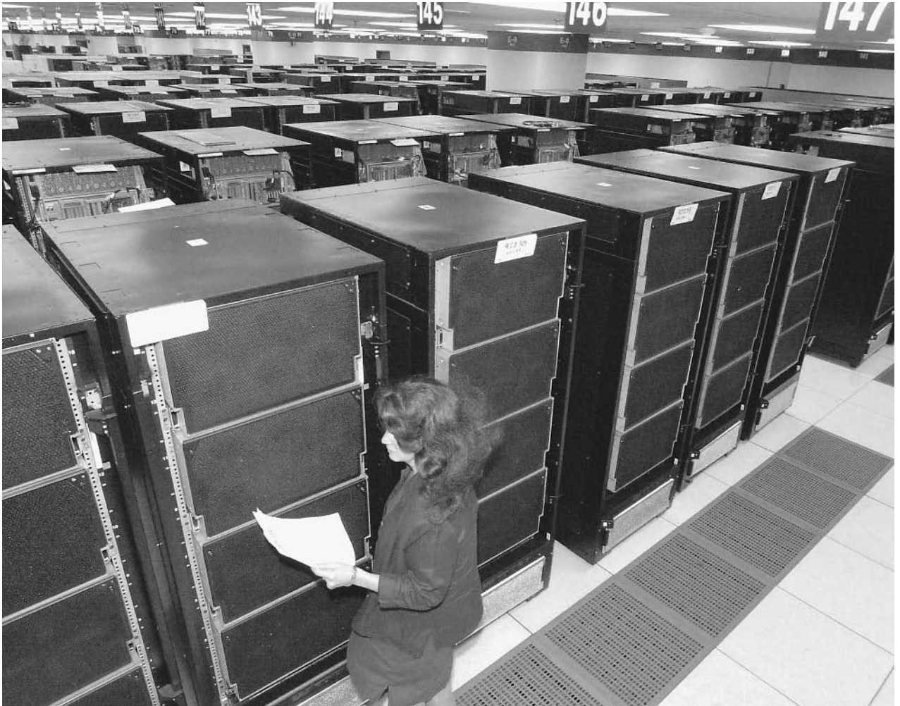
A technician monitors IBM's ASCI White in 2000, then the world's fastest supercomputer, that is capable of 12 trillion calculations per second. The Department of Energy uses ASCI White to analyze and protect the nation's nuclear weapons stockpile. AP/WIDE WORLD PHOTOS.
