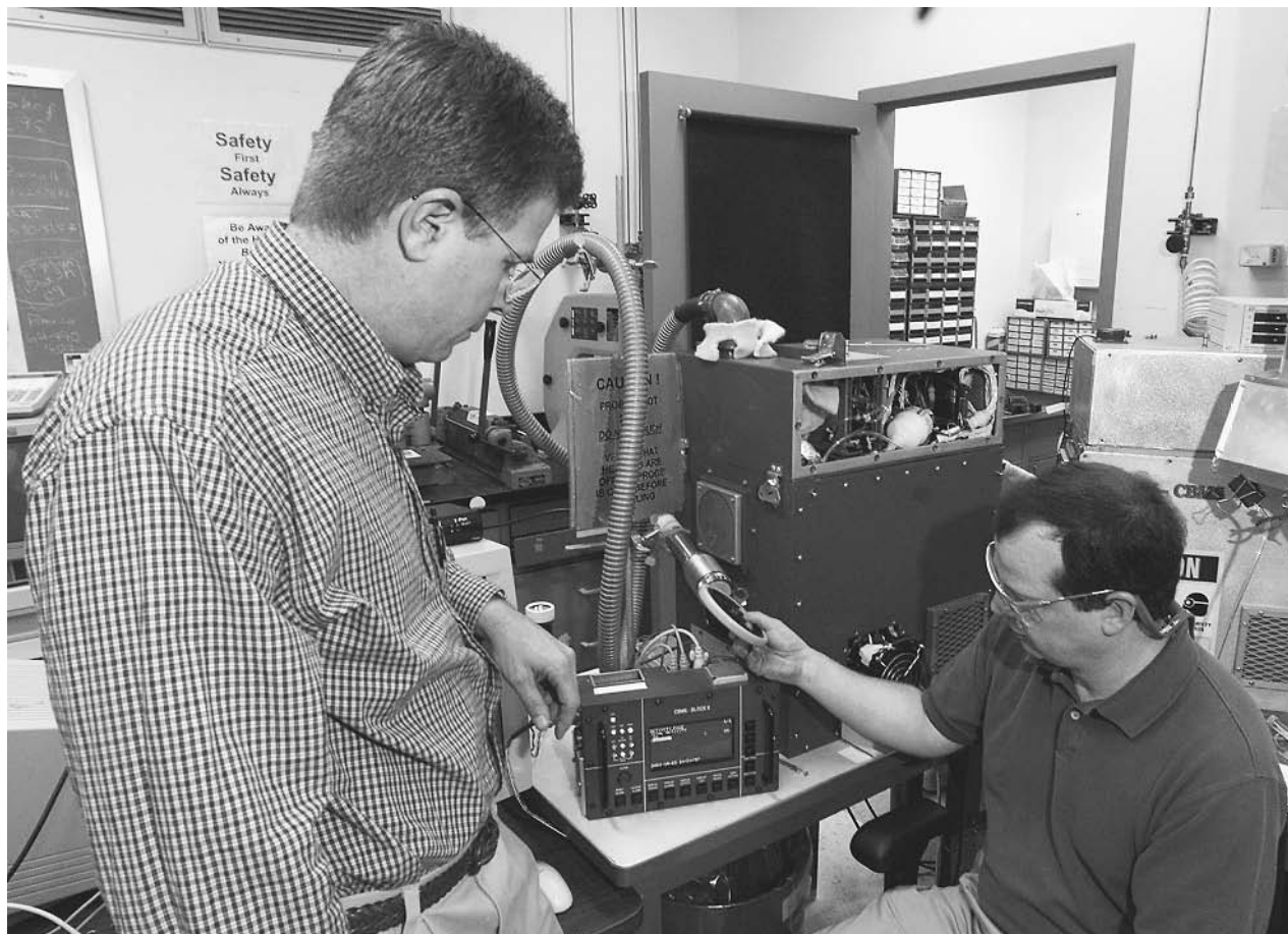
Researchers at the Oak Ridge National Laboratory in Oak Ridge, Tennessee, test a portable chemical and biological agent monitor developed for the army and marines in 2001. AP/WIDE WORLD PHOTOS.
