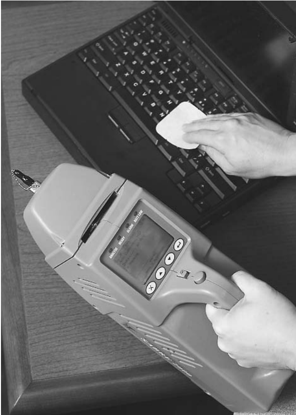
A technician collects a sample from a laptop computer that will be analyzed by the Sabre 2000 trace detection instrument, which can detect traces of explosives, drugs, or chemical weapons. AP/WIDE WORLD PHOTOS.
