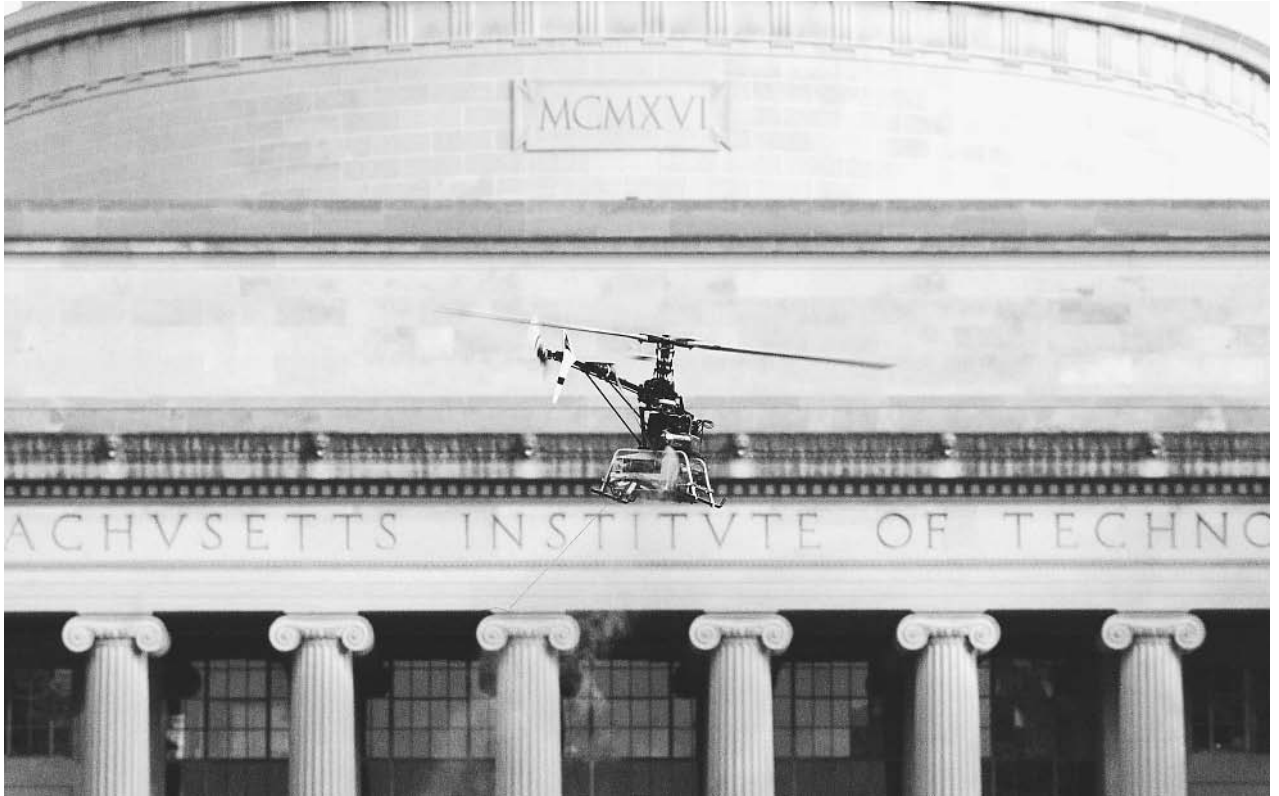
A 17-pound miniature helicopter created by a group of researchers at the Massachusetts Institute of Technology in 2002 could have future uses for civilian or military surveillance, shooting aerial camera footage, or scouting disaster areas and other dangerous terrain. AP/WIDE WORLD PHOTOS.
