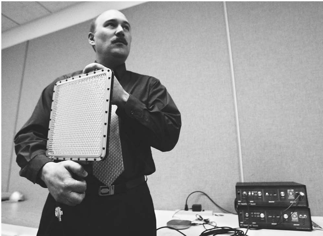
An executive with American Technology Corporation displays a type of sound-gun device that can beam sound to a person so that it appears to be coming from a wall or other inanimate object. Soldiers may someday have similar non-lethal weapons in their arsenals. AP/WIDE WORLD PHOTOS.
