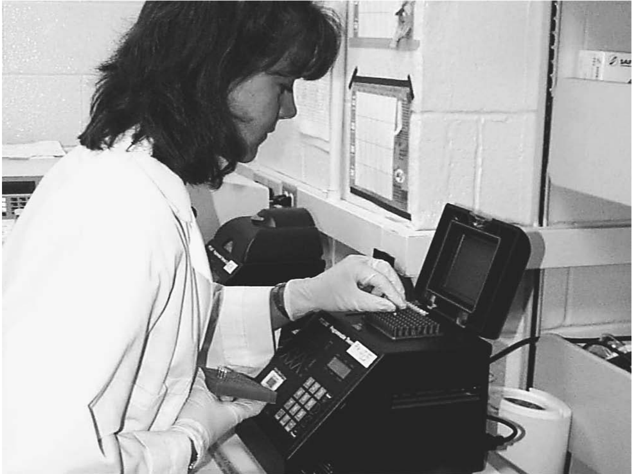
A scientist at the U.S. Army's biodefense laboratory at Ft. Detrick, Maryland, performs PCR analysis on anthrax samples. AP/WIDE WORLD PHOTOS.
