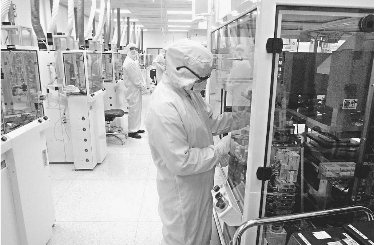
A technician places a gene chip into one of the photo lithography machines shown at a production facility in California. Gene chips are dime-sized pieces of glass infused with DNA fragments that allow researchers to study how and why genes react to various stimuli. AP/WIDE WORLD PHOTOS.
