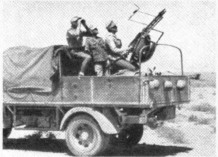
Plate 765. Kfz 4 based on the BMW le gl Einh PKW 4 x 4. Plate 766. The Zwillinglafette 36 mounted on a medium truck.
