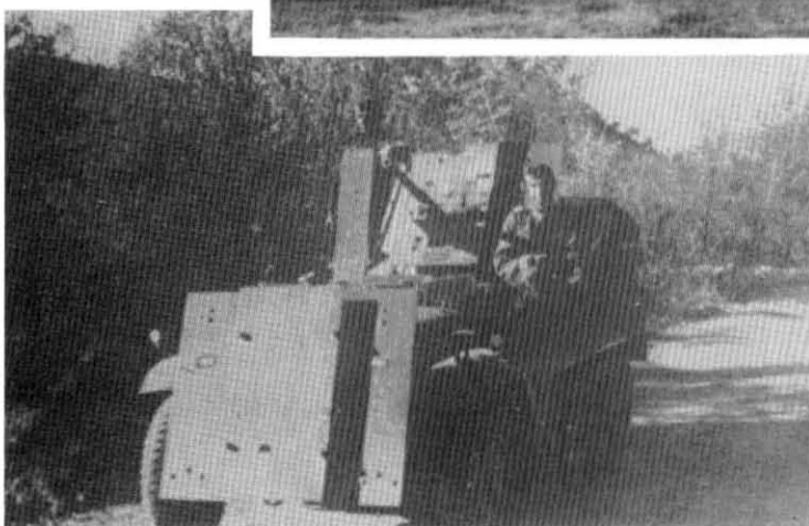
Plates 659-661. 3.7cm PaK35/36 on the Sd Kfz 10; right, with pedestal mount; below right, with additional armour plates on the front of the engine and at the side of the gun.
