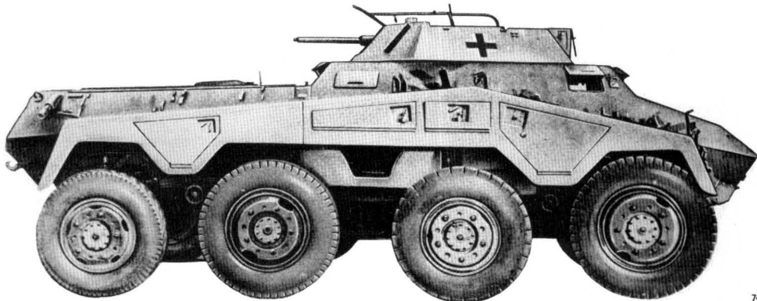
Plates 745-746. S Pz Sp Wg (2cm) (Sd Kfz 234/1). Plate 745 shows the 2cm KwK38 L/55 mounted in the open turret; in Plate 746, the turret is traversed and the gun points to the rear of the vehicle.
