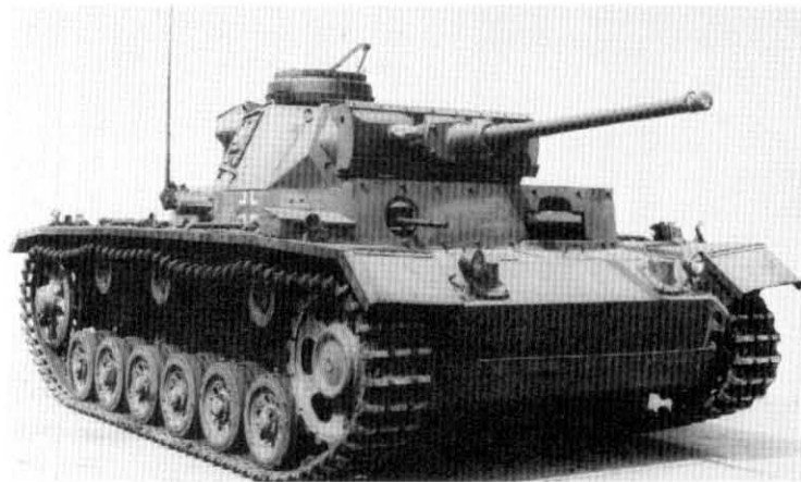
Plates 204-205. Pz Kpfw III Ausf L, showing the spaced armour on the gun mantlet and hull front. (Note also the elimination of the loader's vision port on the side of the turret.)
