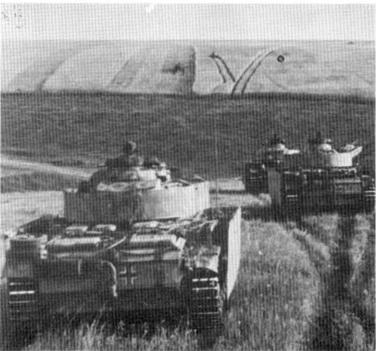
Plates 206-207. Pz Kpfw III Ausf M. Note the modified exhaust valve for deep wading and the absence of both the hull escape hatch and the loader's vision port in the turret side. Right: vehicles equipped with Schürzen (armour skirts) on the Russian Front.
