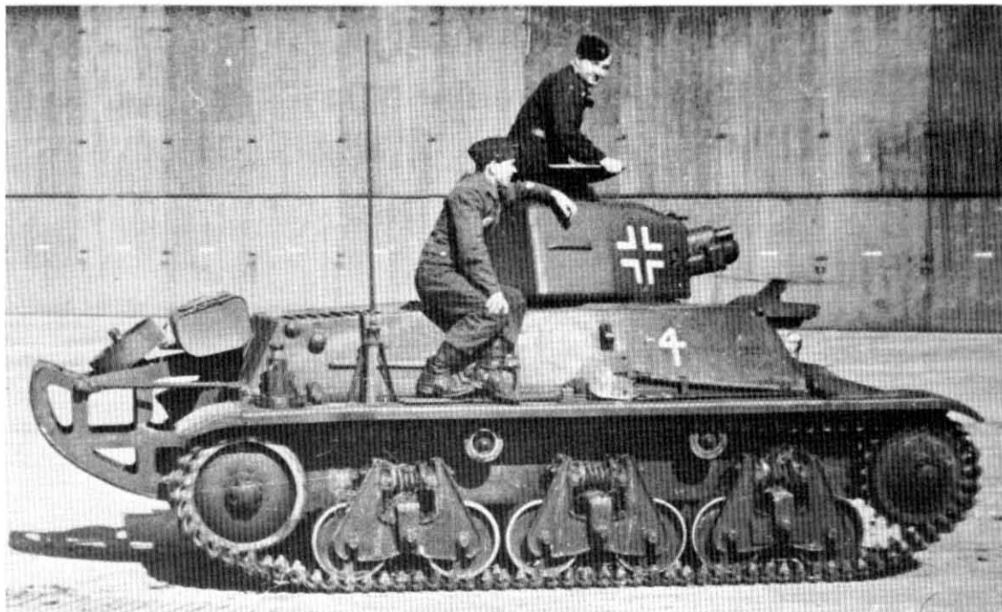
Plate 803. Pz Kpfw 38H in Russia. Plate 804. Pz Kpfw 39H on operations against Yugoslav partisans in 1944. Plate 805. Pz Kpfw 39H.
