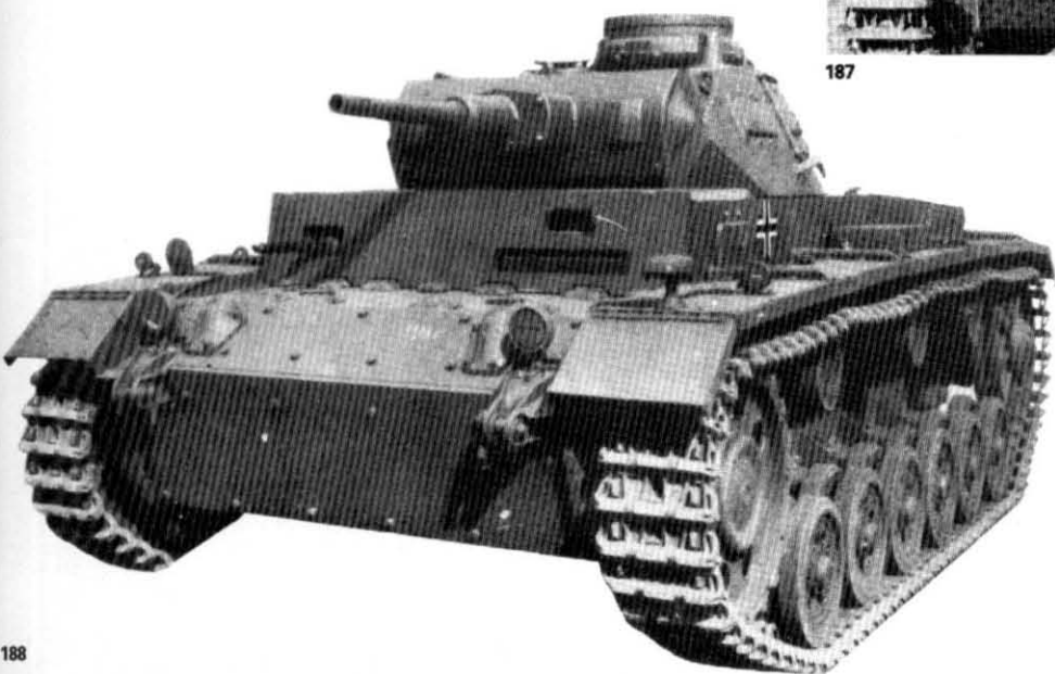
Plates 185-186. Pz Kpfw III Ausf E. Plates 187-188. Pz Kpfw III Ausf E or F, converted to mount the 5cm KwK L/42 gun in an external mantlet (in contrast to the internal mantlet used for the original 3.7cm KwK L/46.5 shown in Plate 186). Plate 188 also shows the additional armour that was added to the hull front. Plate 189. Kugelblende 30, the hull machine-gun housing used on Pz Kpfw III Ausf E, F, G and H, and on Pz Kpfw IV Ausf A, D and E.
