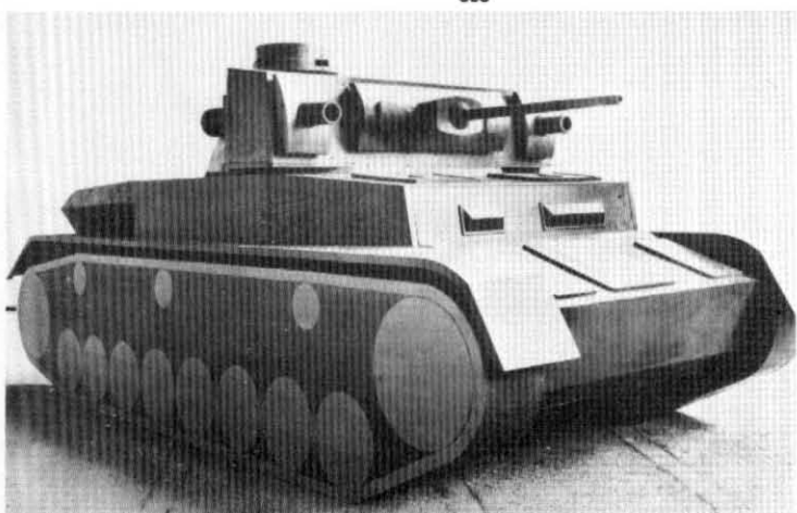
Plates 383-385 (right and below). Rocket projectors and recoilless gun mountings on Pz Kpfw IV chassis. Plate 383 shows the experimental Raketenwerfer auf Pz Kpfw IV; the turret was replaced by a fixed armoured hatch and a box-type rocket projector containing four rockets. Plate 384 shows front and rear views of a wooden mock-up of Pz Kpfw IV für zwei 7.5cm Ruckstossfrei Kanone 43 and 3cm MK103, a project to mount two 7.5cm recoilless guns and a 3cm automatic cannon on the Pz Kpfw IV chassis.
