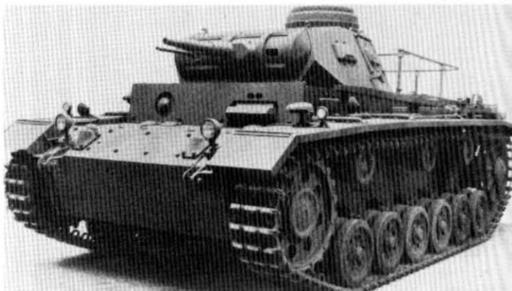
Plates 223 and 224 (opposite page, top). Pz Bef Wg III Ausf H, with additional armour on nose and front vertical plate.
