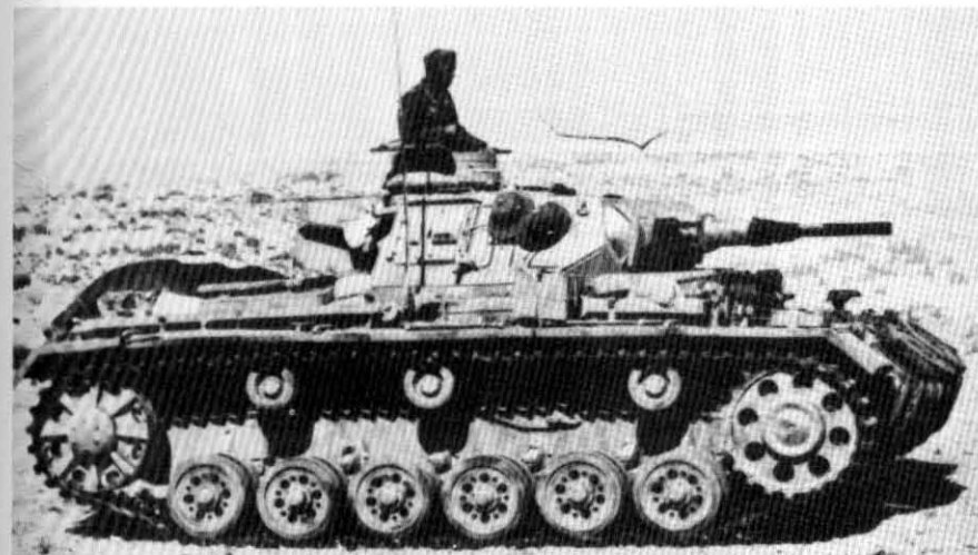
Plates 192-193. Pz Kpfw III Ausf G. The vehicles in the top photograph have the redesigned cupola and driver's visor (and the third vehicle along mounts the 5cm KwK L/42). The vehicle shown in North Africa (left) has the 5cm KwK L/42, but retains the old type of cupola. Plate 194. The cupola used on Pz Kpfw III Ausf G, H, J, L, M and N, and on Pz Kpfw IV Ausf E, F and G.
