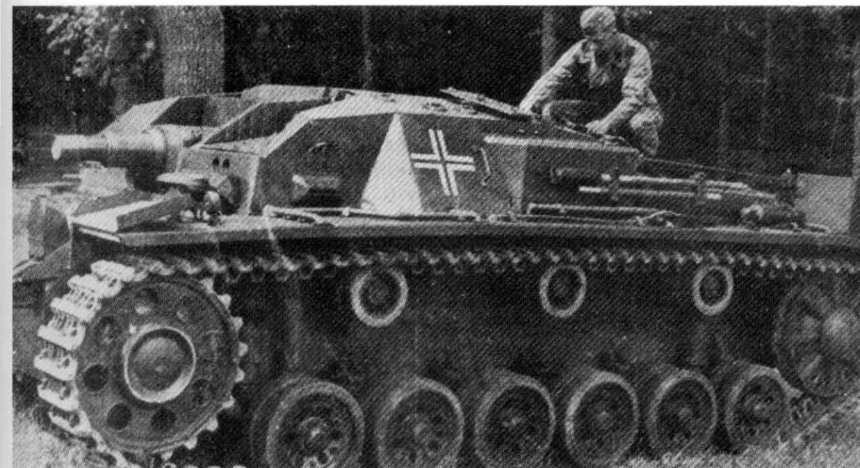
Plates 244-245. StuG III Ausf A (showing the Pz Kpfw III Ausf F suspension). Plate 246. One of the prototype (0-series) vehicles.
