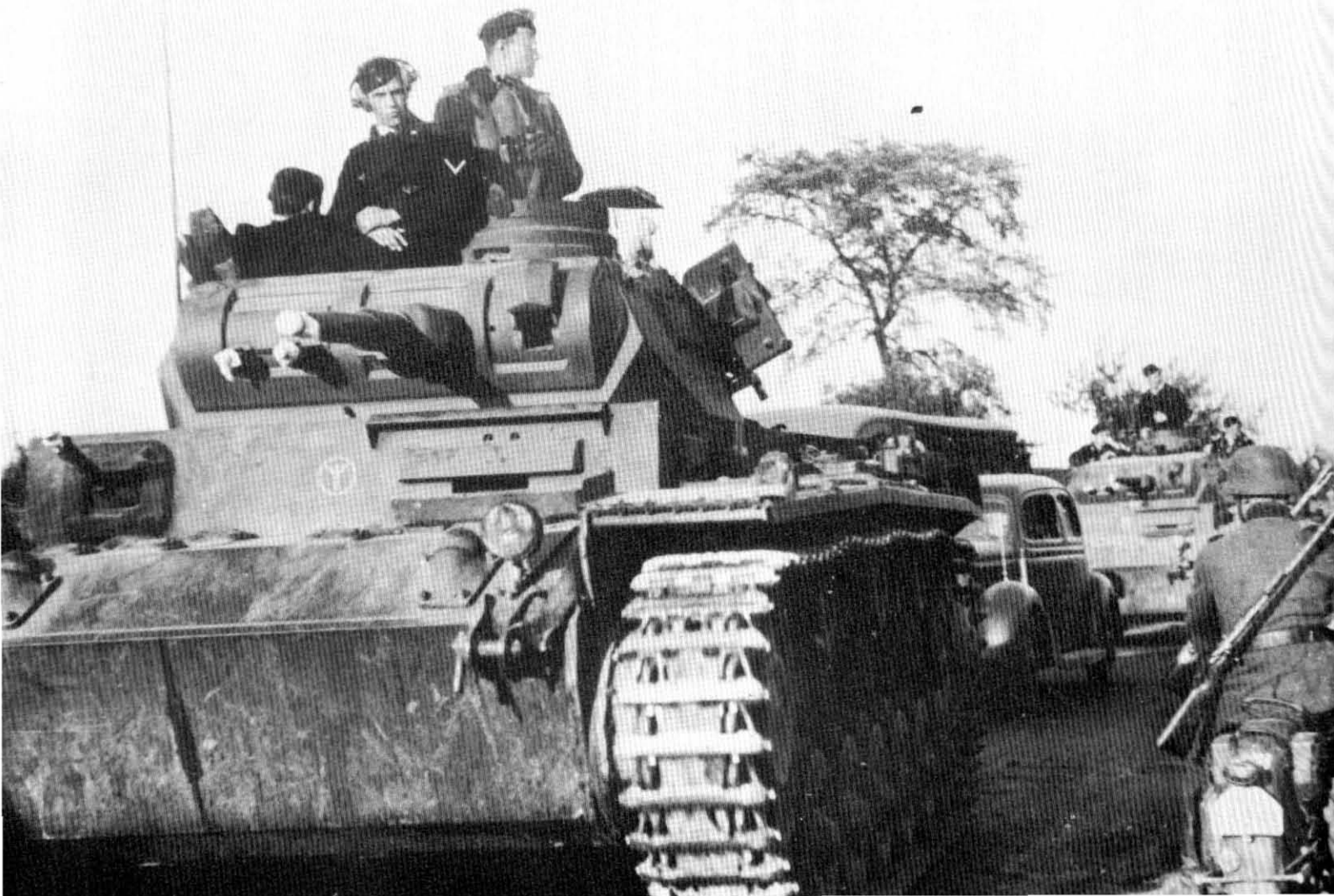
Plates 190-191. Pz Kpfw III Ausf F. The vehicle shown above carries the 5cm KwK L/42 gun in an external mantlet.
