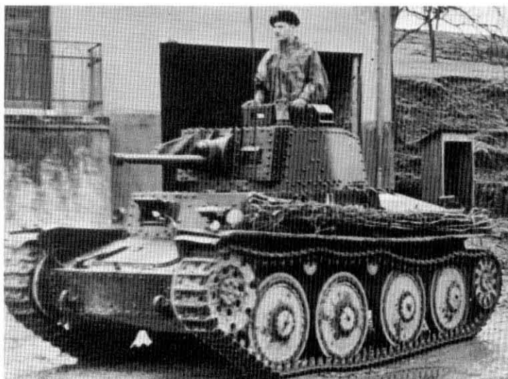
Plate 127 (right). Pz Kpfw 38(t) Ausf C with the hull machine-gun removed and the port plated over.
