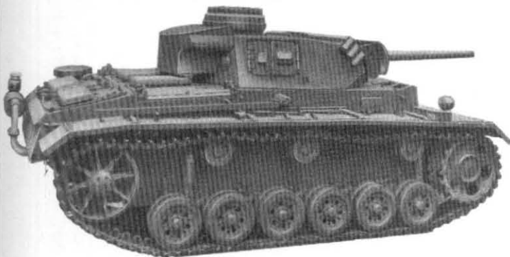
Plates 206-207. Pz Kpfw III Ausf M. Note the modified exhaust valve for deep wading and the absence of both the hull escape hatch and the loader's vision port in the turret side. Right: vehicles equipped with Schürzen (armour skirts) on the Russian Front.
