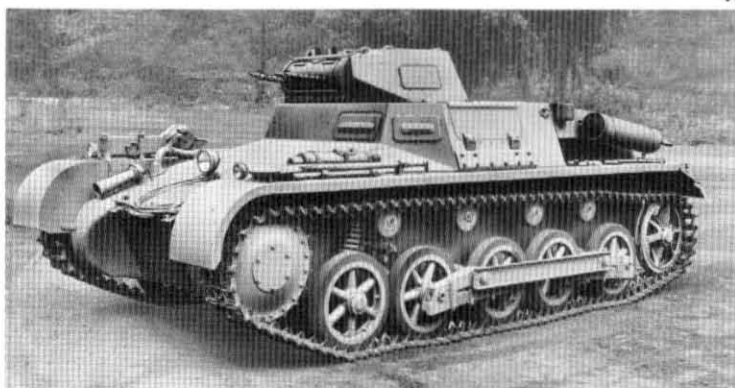
Plates 44-46. Pz Kpfw I Ausf B: top, in France, 1940; above, an experimental vehicle powered by an air-cooled Krupp M601 diesel engine in an attempt to increase speed; below, the Ausf B in Poland in 1940.
