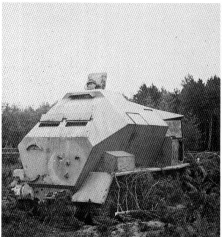
Plates 673-674. Feürlleitpanzerfahrzeug für V-2 Raketen auf Zgkw 8t; left, in travelling order, towing the 'Bodenplatte' (launching-pad base plate); right, in position for a launch, with the armoured rear section as the control point.
