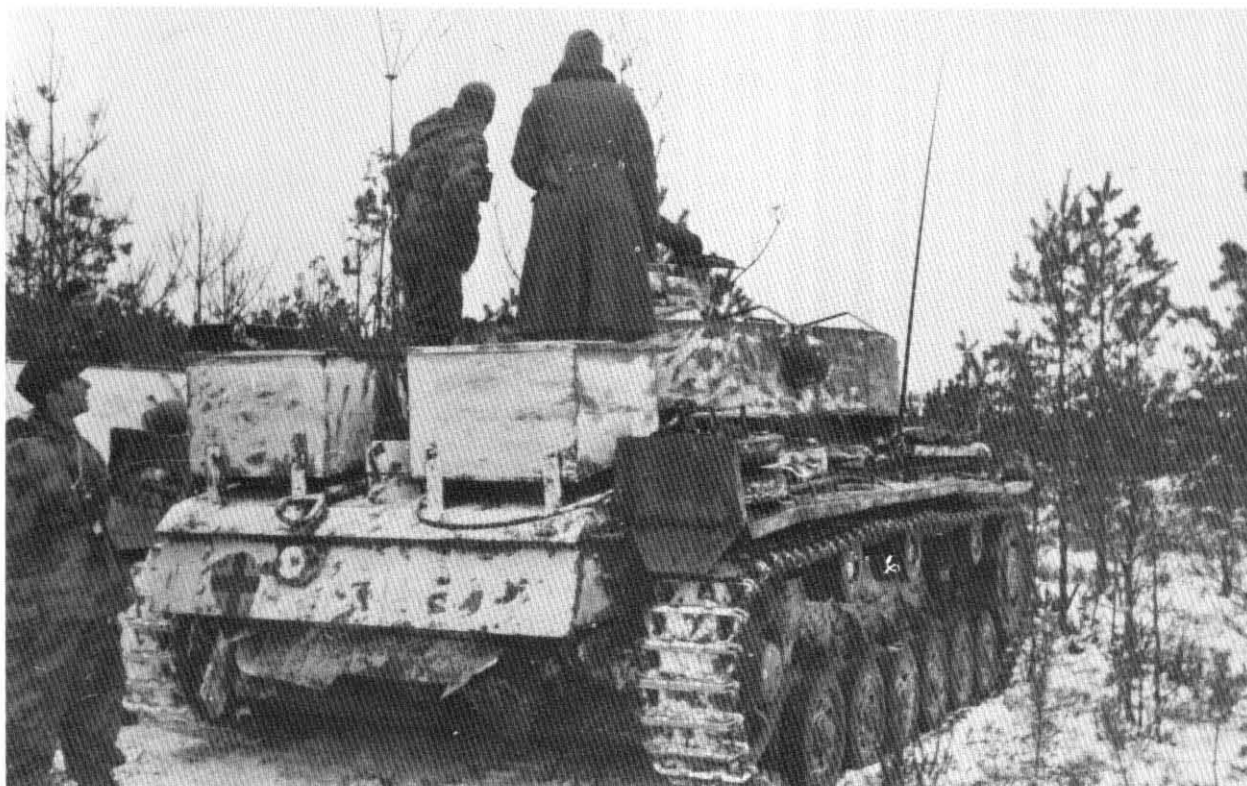
Plates 226-227. Pz Bef Wg III Ausf K. Plate 226: a vehicle disabled during fighting on the Ukrainian Front. Plate 227: in Russia, with supplementary armour plate on the front superstructure. Plate 228. A command tank based on the Ausf L.
