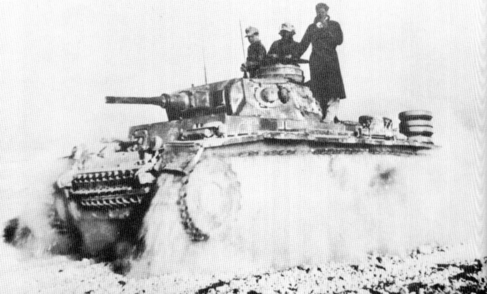
Plates 195-196. Pz Kpfw III Ausf H. A new type of drive sprocket, with six D-shaped holes and open eight-spoked rear idler, was introduced with this model. Note the 30mm armour plates bolted on to the upper and lower nose plates. Above: in Sofia, 1941; below, at speed in North Africa.
