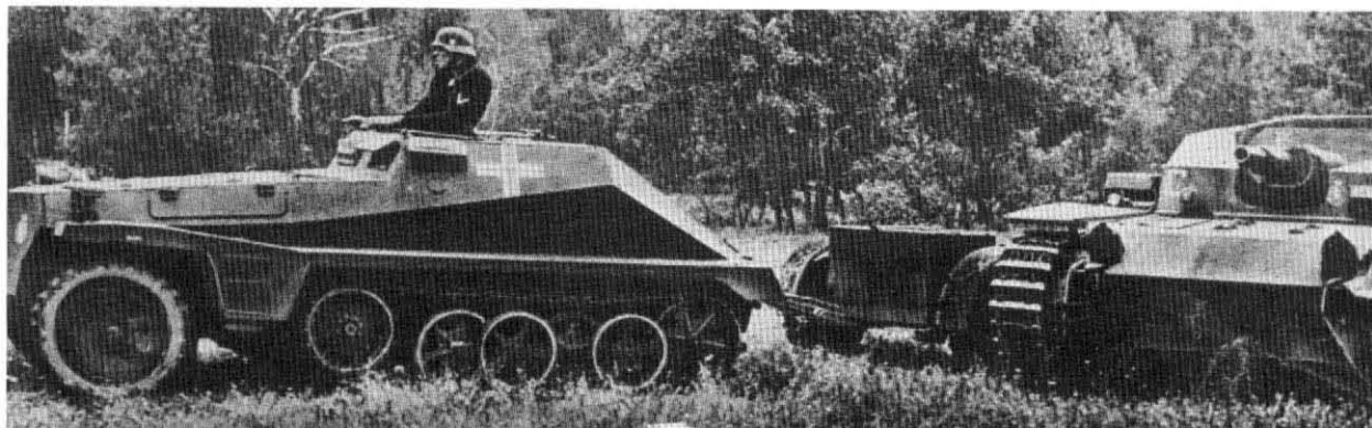
Plates 583-584. Sd Kfz 252 leichter gepanzerter Munitionskraftwagen with its Sd Ah 3 1/1 trailer (left, passing a Sturmgeschütz).
