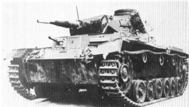
Plates 190-191. Pz Kpfw III Ausf F. The vehicle shown above carries the 5cm KwK L/42 gun in an external mantlet.
