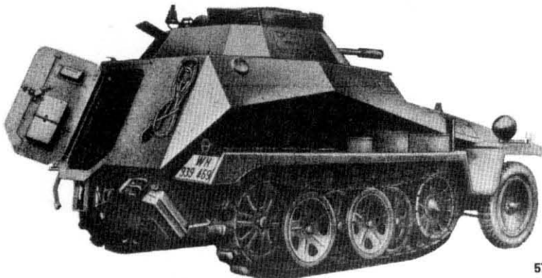
Plates 571-574. Sd Kfz 250/9 leichter Schützenpanzerwagen (2cm). That in Plate 573 is based on the 'Neu' vehicle, as well as having the later Hängelafette turret (see page 192). Below, vehicles operating in Russia.
