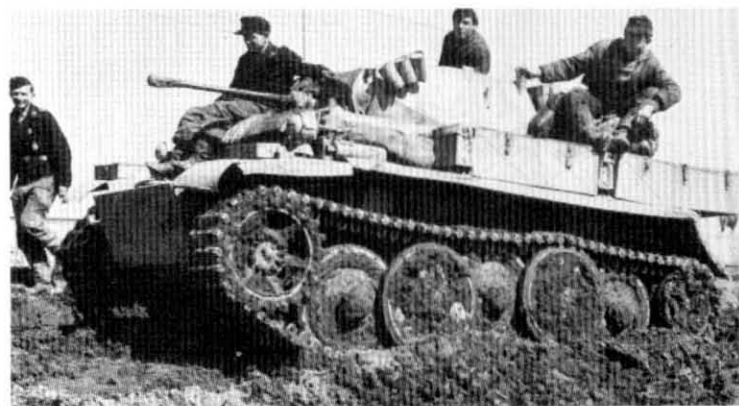
Plates 97-98. Pz Kpfw II Ausf L: Plate 97 shows the vehicle in service on the Russian Front. (Note the additional armour on the nose plate.)
