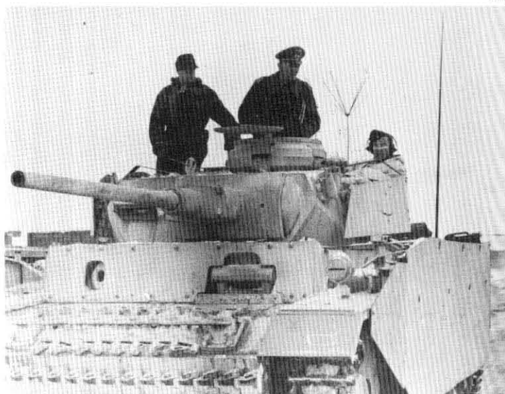
Plates 226-227. Pz Bef Wg III Ausf K. Plate 226: a vehicle disabled during fighting on the Ukrainian Front. Plate 227: in Russia, with supplementary armour plate on the front superstructure. Plate 228. A command tank based on the Ausf L.
