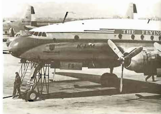
Above: A Lockheed 049 Constellation of Modern Air in January 1965 Right: Friesland , an L-749 of KLM's Flying Dutchman service. The 749 was similar to the 649 but had a larger fuel capacity and consequently longer range
