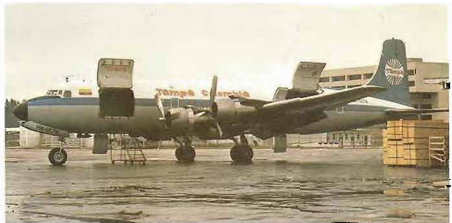
Above: HK-1276, a DC-6A of Tampa Colombia photographed in February 1978. Several DC-6As and -Bs are still in service for small South African airlines. There are no fuselage windows and two upward-opening freight doors on this aircraft Left: An American Airlines DC-6A freighter with its water-methanol injection 2400-hp Double Wasp CB16 engines
