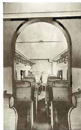
Above: F-ANPG Albatros which entered Air France service in 1935 Far left: F-AOTU, delightfully named La Séduisante (the Seductress ) Left: The spacious cabin was well decorated, soundproofed and had heating and air-conditioning systems
