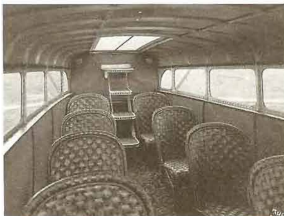
Left: The simple interior of the S-38 amphibian. The seating arrangement could be revised to almost any plan specified Below: A Hawaiian Airlines S-38 delivering newspapers to the island
