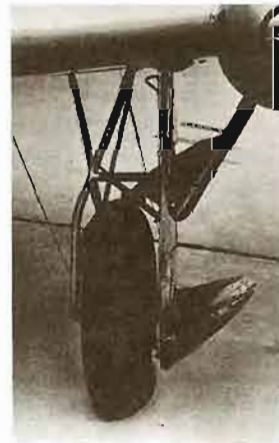
Far left: The Orion flown by the aviators Post and Rogers Left: Orion was very probably the first transport aircraft to use a retracting undercarriage; the mainwheels retracted sideways and into the wing Below: One of the two Swissair Orions
