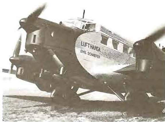
Above: D-ALAN Edward Dostler in its prewar Lufthansa livery Left: The three Junkers Jumo 5 heavy-oil engines of D-AJYR Emil Schaefer Below left: Södermanland , a 12-seat floatplane version
