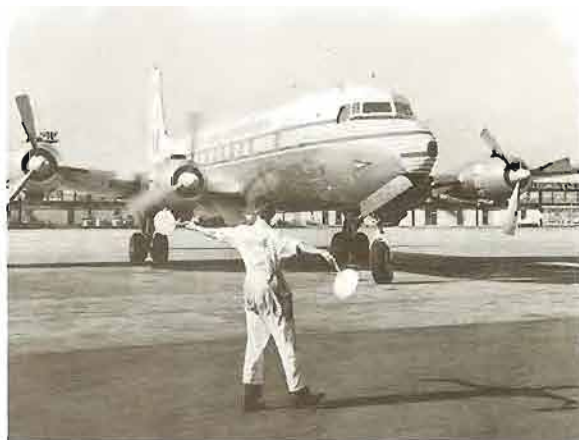
Left: A DC-6B of Alitalia's former charter subsidiary Società Aerea Mediterranea (SAM). The DC-6B was without the reinforced floor and main deck cargo doors of the DC-6A and was produced in larger numbers than any other version in the DC-6 series Below: A Guest Aerovias Mexico DC-6 on the runway at Paris in 1939
