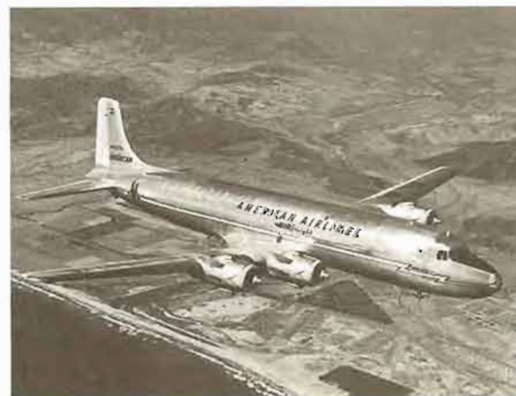
Above: HK-1276, a DC-6A of Tampa Colombia photographed in February 1978. Several DC-6As and -Bs are still in service for small South African airlines. There are no fuselage windows and two upward-opening freight doors on this aircraft Left: An American Airlines DC-6A freighter with its water-methanol injection 2400-hp Double Wasp CB16 engines
