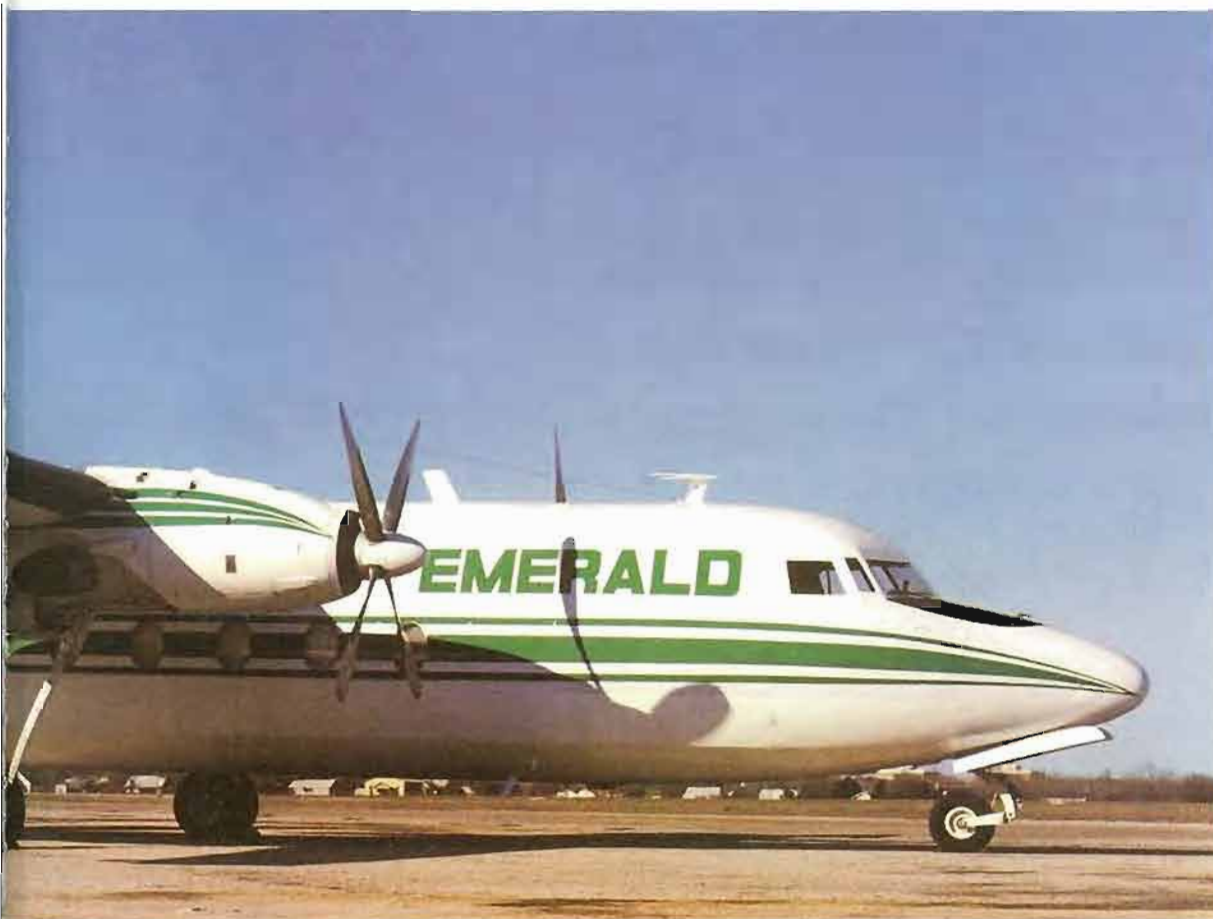
Far left: An F27-400 operated by Gulf Aviation, which has been called Gulf Air since 1973 Left: A Fokker Friendship at Austin, Texas. The special long-nosed version, built by Fairchild, was designed to incorporate an all-weather radar
