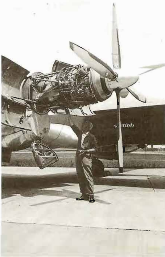
Left: Checking the right-hand engine of a BAe 748. The twin Rolls-Royce Dart RDa.7 Mk 536-2s each drive a Dowry Rotol four-blade constant-speed fully-feathering propeller
