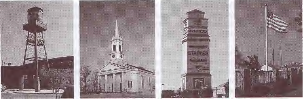
Figure 239: The many and various places where microwave masts are hidden to keep their location secret of the public
