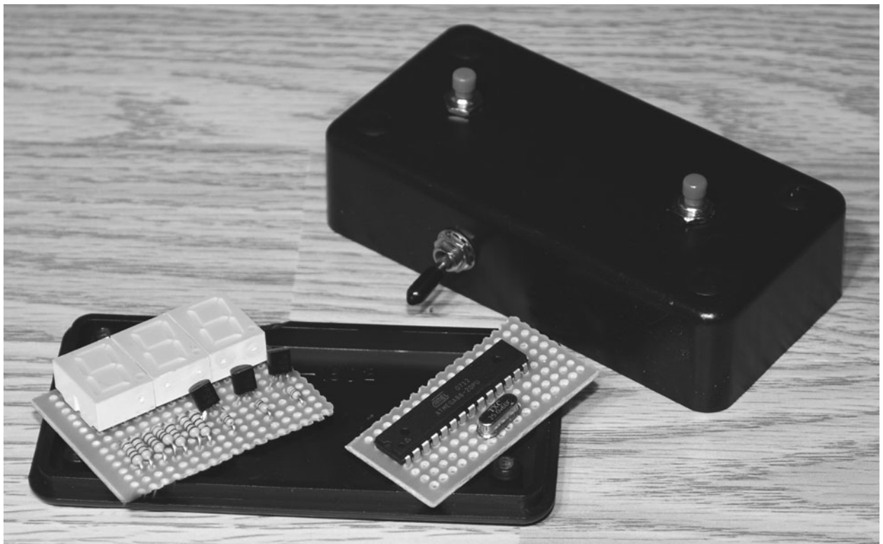
Figure 16-4 Deciding on a cabinet and board layout.
