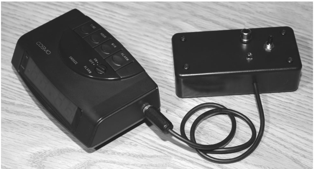
Figure 10-10 Alarm clock and relay board ready to use.
