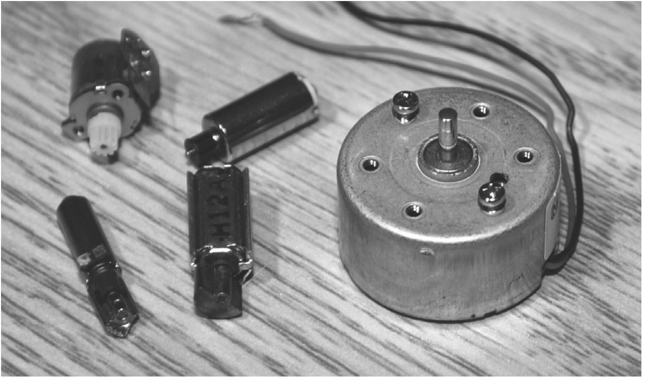
Figure 9-3 Small dc motors that can make vibrations.
