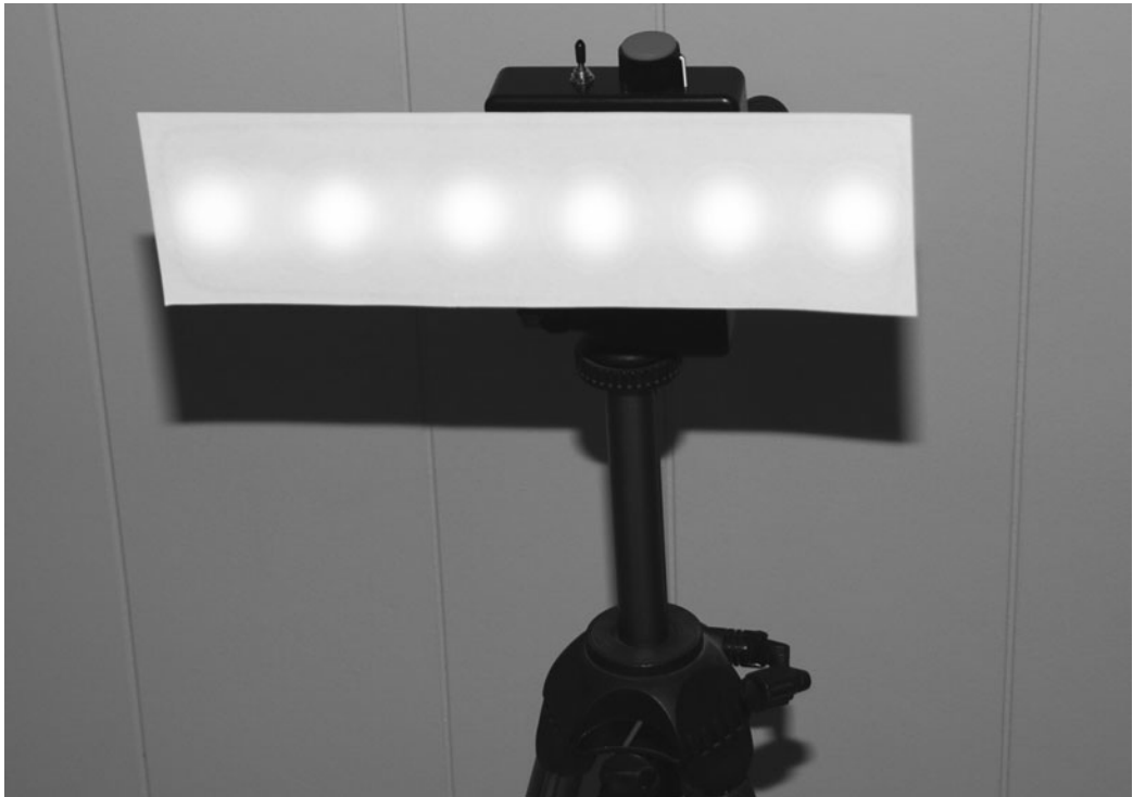
Figure 17-6 Diffuser screen lit by the LEDs.
