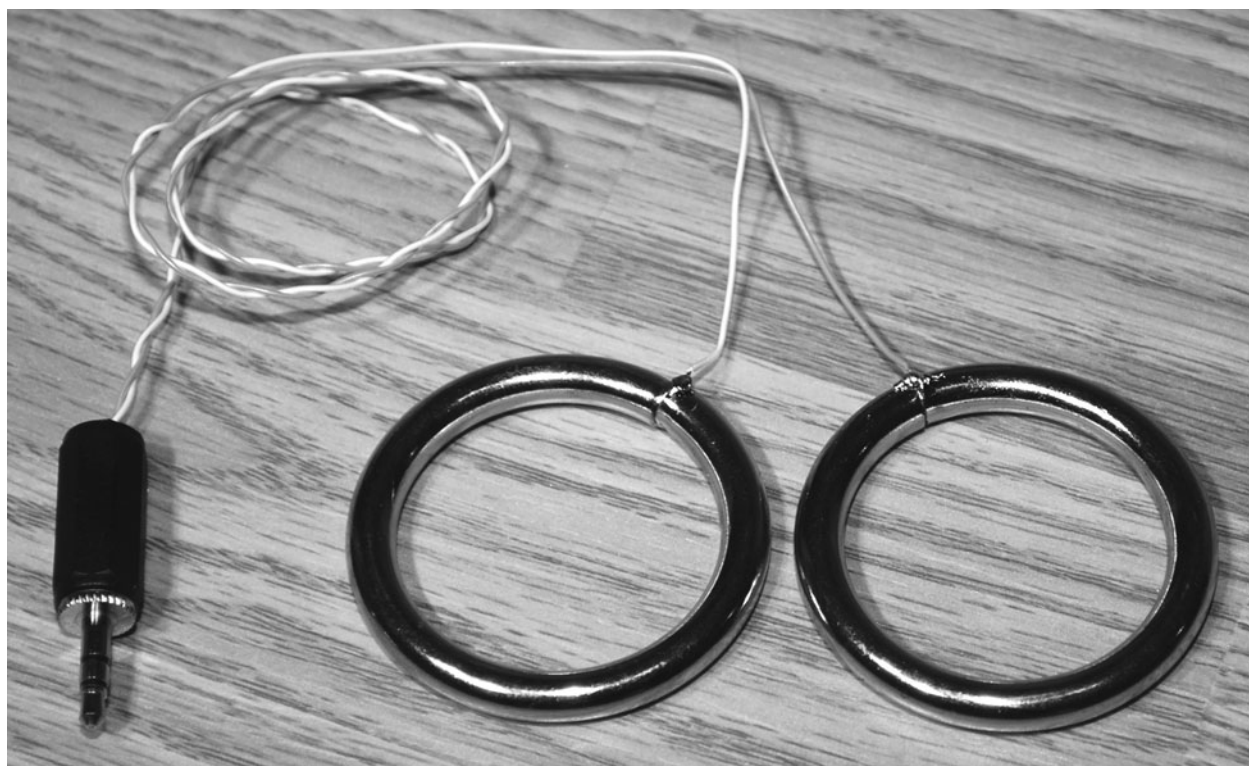
Figure 6-6 Making probes for the subject’s hands.
