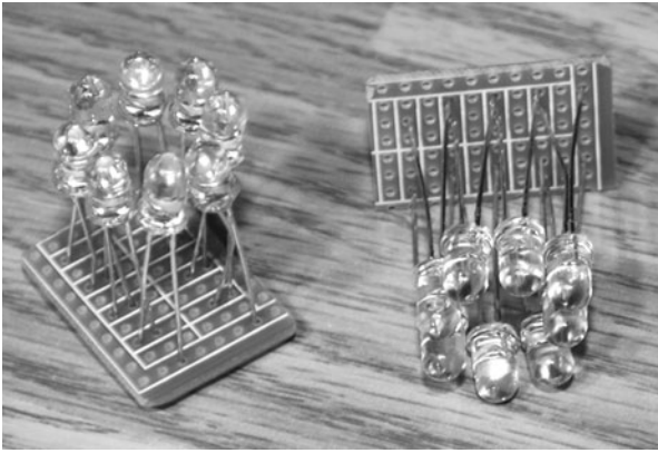
Figure 14-8 Soldering the LED clusters to a perf board.
