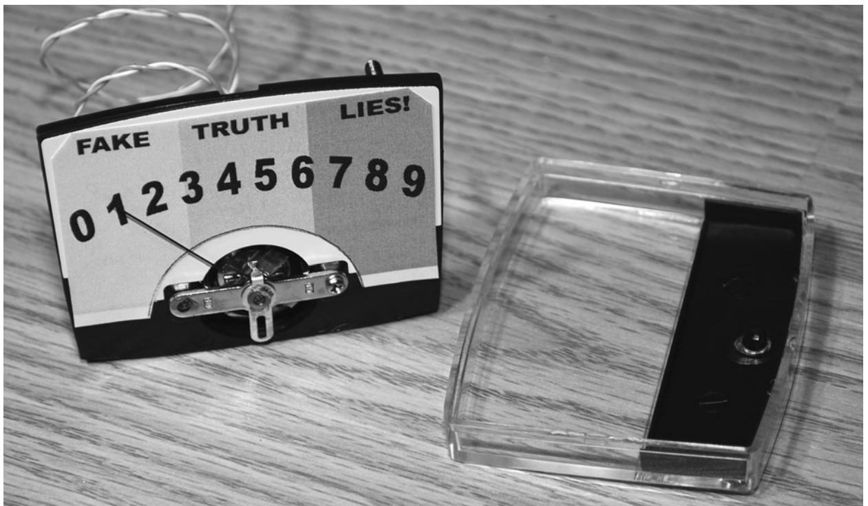
Figure 6-5 Gluing the new display over the old one.
