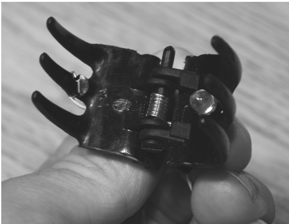
Figure 5-9 Open jaws reveal the LED and the LDR.
