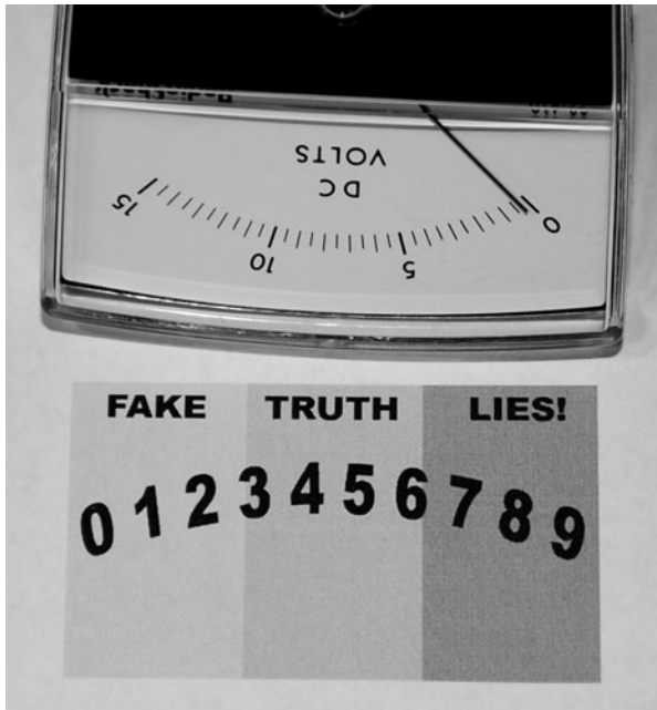
Figure 6-4 Making a replacement readout plate.
