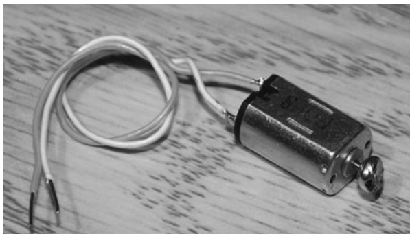
Figure 9-5 Motor with counterweight attached.
