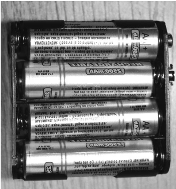
Figure 2-7 Six volts from four batteries.
