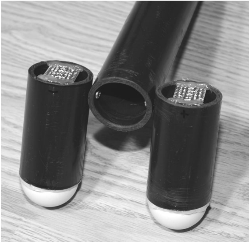
Figure 14-11 Adding a support tube for tripod mounting.
