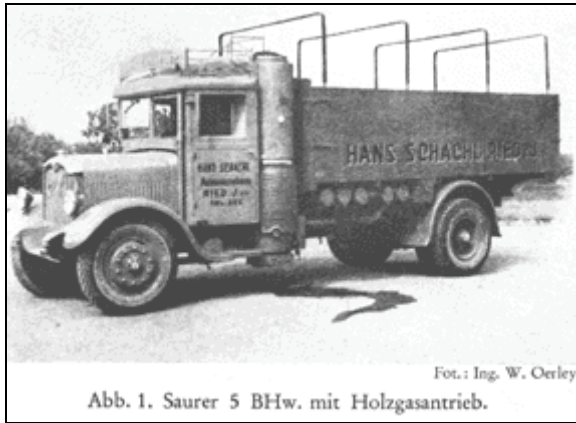
Illustration 3: A German wartime producer gas truck form Saurer (Type 5 BHw, produced until 1935; Rudolf 2003, p. 461)
