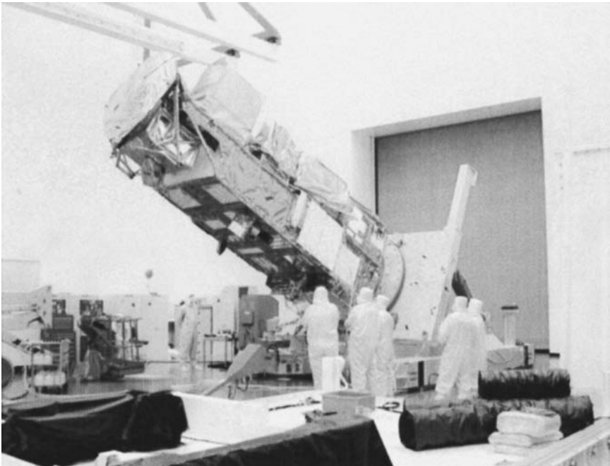
The inner workings of the Terra satellite being erected to a vertical orientation so that the final assembly of the space vehicle can be completed. (Courtesy of the National Aeronautics and Space Administration)
