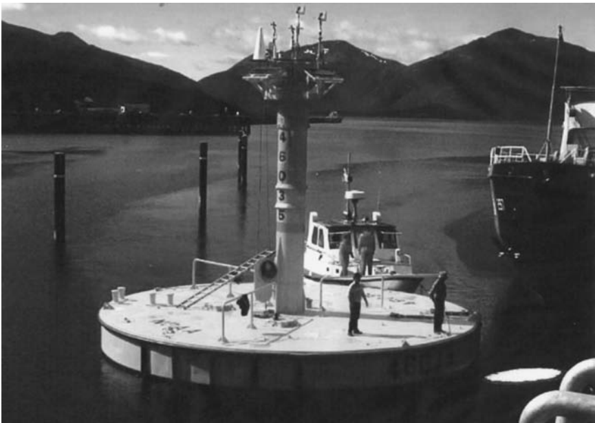
Weather buoys are automated, floating weather stations. They are deployed and maintained by specialists aboard weather ships. The meteorological data taken in by the instruments on the buoy are relayed via satellite to central computers. (Courtesy of the National Weather Service)
