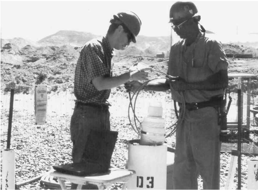
Lightweight, rugged detectors or chemical “sniffers” are needed to monitor possible leaks or breakdowns of containment of toxic materials. Department of Energy technicians are testing models of such devices. (Courtesy of the Department of Energy)
