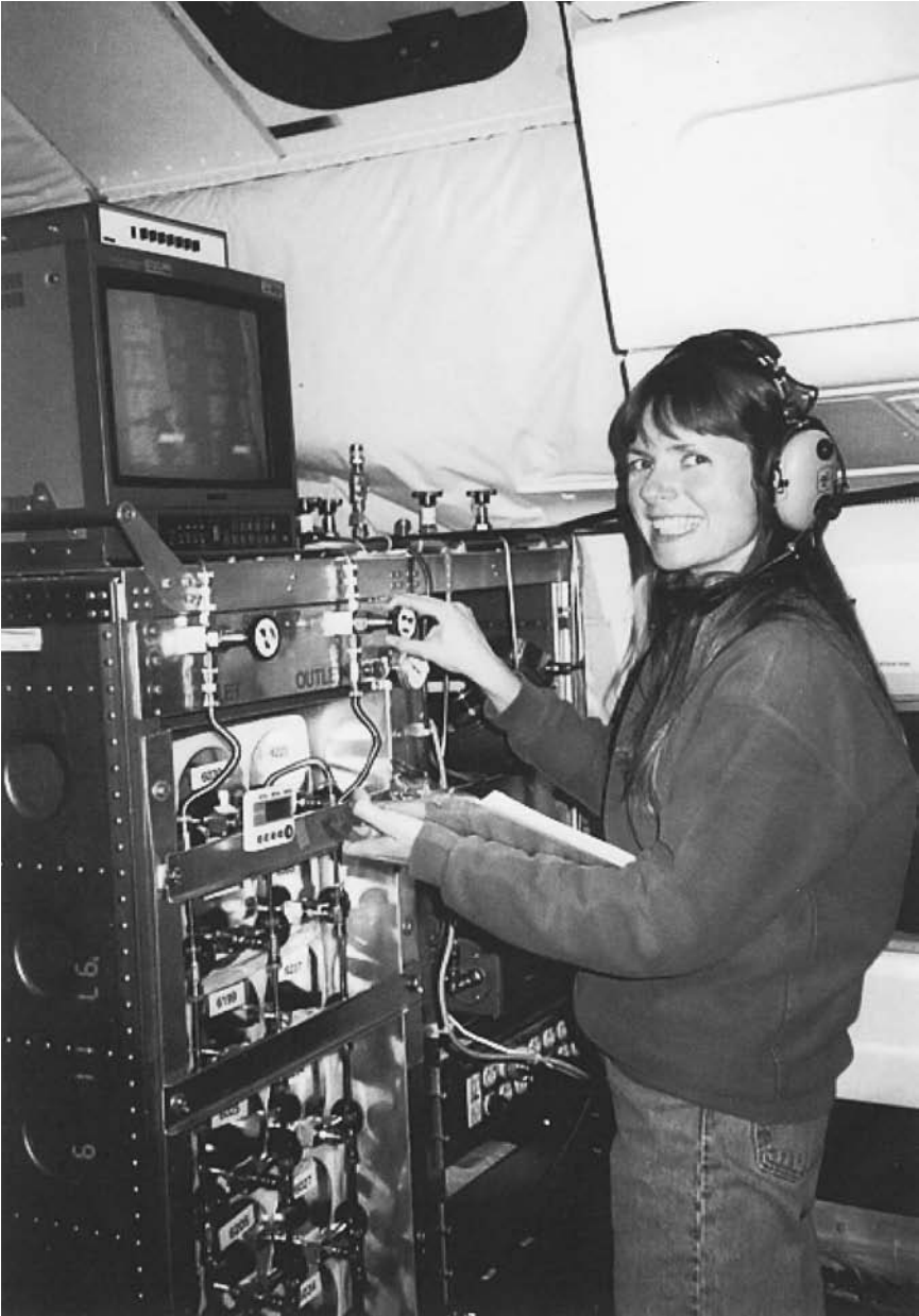
Dr. Nicola Blake, a member of F. Sherwood Rowland's research team, checking on the instruments for determining the level of trace materials—including chlorine compounds—at stratospheric altitudes (Courtesy of the National Aeronautics and Space Administration)
