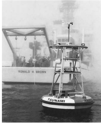
The DART buoy is linked to an underwater pressure gauge that activates a warning signal when a tsunami wave passes. (Courtesy of the National Oceanographic and Atmospheric Administration)
