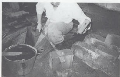
Next the block is hammered down and folded over.
