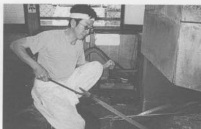
When the charcoal fire is at the right temperature, the smith picks up the sword and puts it into the forge.
