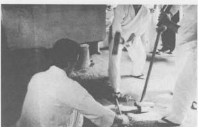
Kawagane and shingane being forged together.
