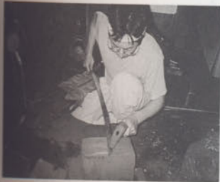
After arabi-zukuri, the blade is heated again. At the section which will become the tip, or kissaki, the harder kawagane is hammered into a sharp point. This process is called hi-zukuri, or rough shaping.
