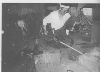
When the charcoal fire is at the right temperature, the smith picks up the sword and puts it into the forge.
