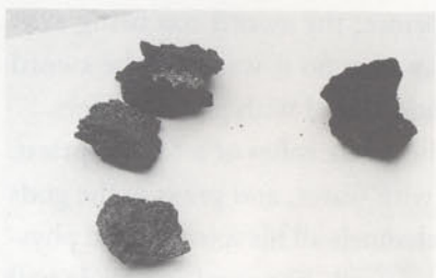
The kera that is used to make swords is called tamahagane.
