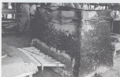
A tatara, or clay smelter, in operation. A tatara is used to convert raw materials into the starting steel needed for the sword.
