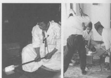
After the kawagane and shingane have been welded together, the block of steel is hammered and shaped into a bar.
