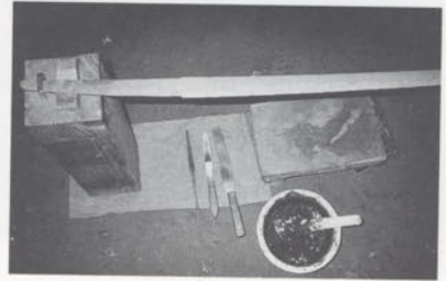
The sword just before tsuchioki, the application of a clay coating that will harden the edge. The way the paste is applied will determine the pattern along the hamon (cutting edge).
