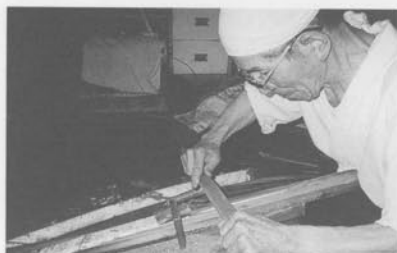
If the condition of the sword after kaji-oshi is satisfactory, the smith then makes diagonal file marks on the tang.
