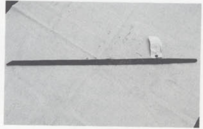
Arabi-zukuri. The flat bar has been forged and shaped to the desired length. What looks like the tip and the cutting edge here is actually the part that will become the blunt end of the blade.
