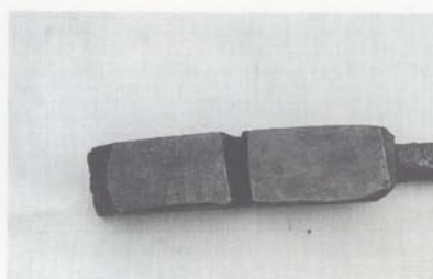
The block, after a cleft has been made with the tagane.
