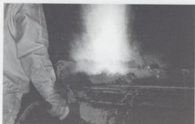
The mass of smelted iron ore and carbon from the charcoal flows from the tataro, resembling the eruption of a volcano.
