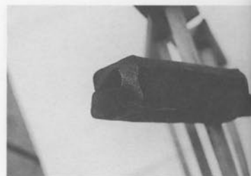
Makuri gitae. This is similar to kōbuse gitae, but in this case the shingane is completely enclosed by a single jacket of kawagane.
