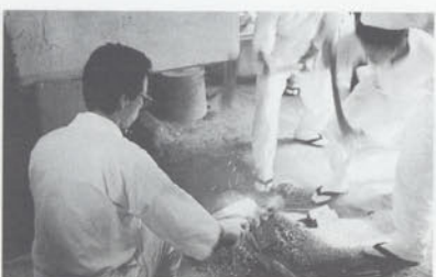
The block is forged and gradually elongated into a steel bar with a square cross-section.
