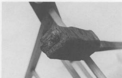
Detail of the surface that will become the cutting edge of the sword.
