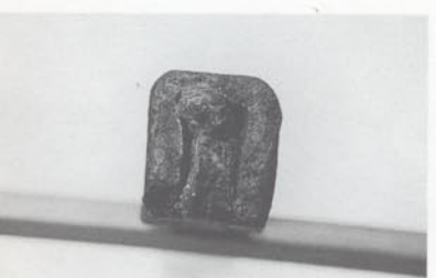
Detail of sword blade construction. The method used here is called kobuse gitae. A core of softer shingane (core steel) is sandwiched between a U-shaped jacket of harder kawagane (jacket steel).
