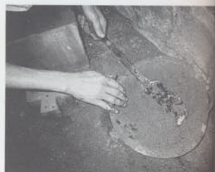
The stack of kōwari is then wrapped with Japanese washi paper and coated with a clay slurry, onto which straw ash and charcoal powder are applied.
