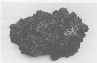
Close-up view of the kera after it has been broken into smaller pieces.
