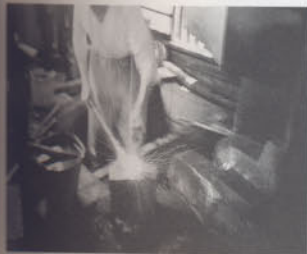
The swordsmith makes a deep cleft into the small block with a cutting tool known as a tagane.
