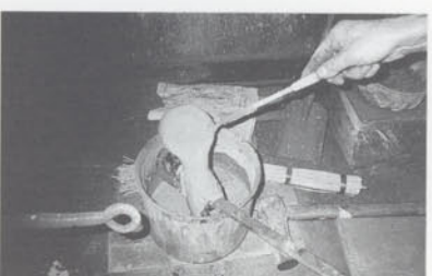
The stack is then coated with a clay slurry and straw ash, after which it is fired to a high temperature in a charcoal furnace, and again hammered into a steel block.
