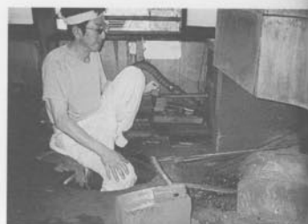
After tsuchioki, the sword is ready for yakiire, or heat treating. The smith here is using bellows to bring the charcoal to the right temperature.
