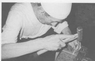
The swordsmith then chisels his name onto the tang.
