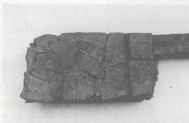
Tsumiwakashi. Using a high-temperature charcoal fire, the tamahagane is formed into small steel wafers called kōwari. These are stacked and welded to a steel bar.
