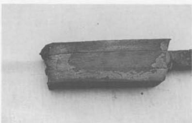
Detail of the hon sanmai (also called san-mai gitae) method. In this case, a layer of softer shingane is sandwiched between two layers of kawagane.
