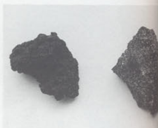
The kera is broken into yet smaller pieces, and separated from zuku, pig iron that contains too many impurities to be used in forging a sword.
