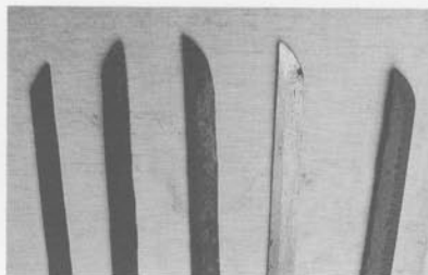
The shapes of the tip at different stages of forging, from left to right.
