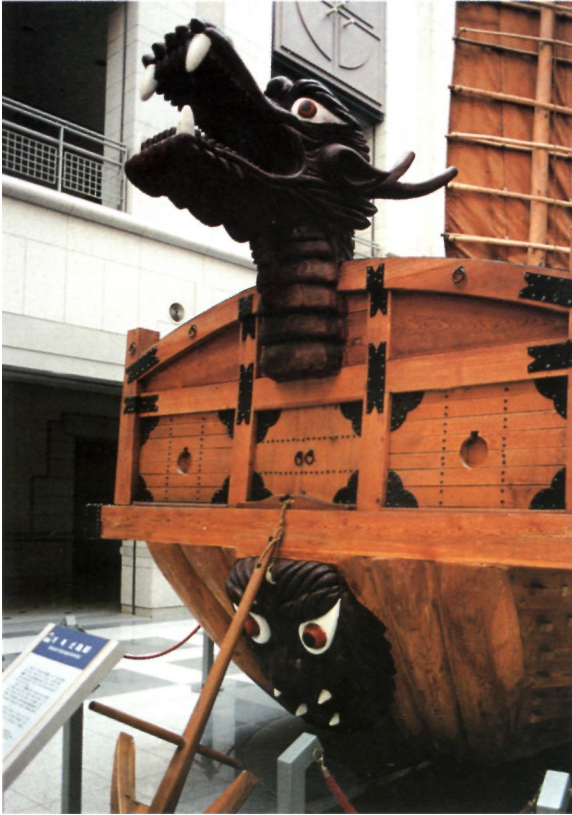
The bow of the 1:2.5 scale replica of the turtle ship in the War Memorial, Seoul. This reconstruction is based on the best available evidence and is regarded as the most accurate ever made. The dragon's head and the lower 'face' for ramming is clearly shown.
