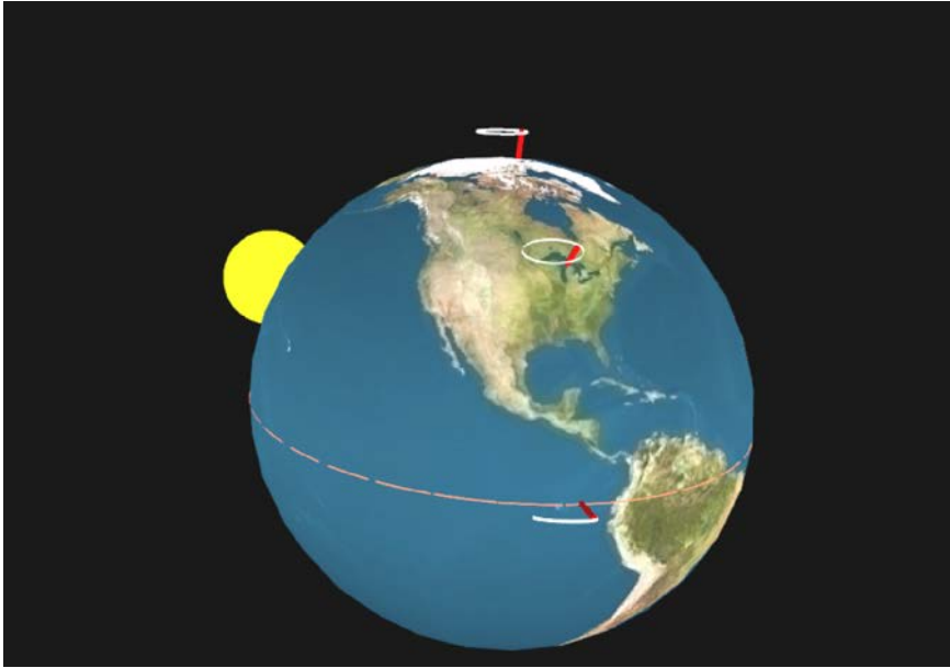
Figure 1: The Earth, moving counterclockwise in the heliocentric system, has passed in front of the sun. The three positions of aberration: the circle at the North Pole; the ellipse at 45° latitude, and the horizontal line at the equator are represented in white.
