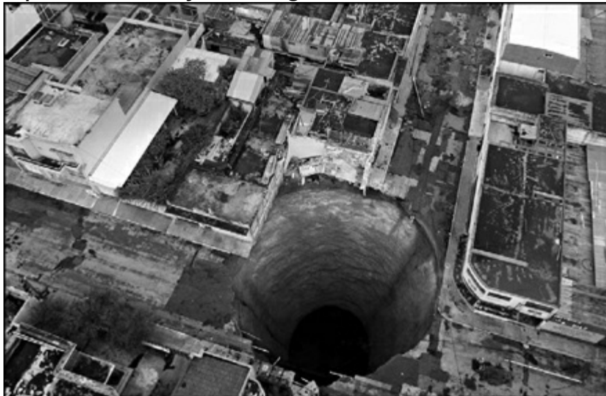
The 2010 sinkhole in Guatemala had likely been forming for several weeks or even years before floodwaters caused it to cave in. (Photo Credit 9.6)
