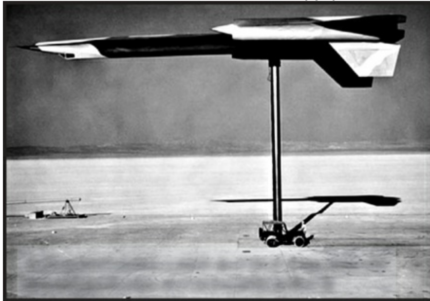
In an undated picture, a mock-up of the A-12 spy plane sits perched upside down on a testing pylon at Area 51. (Photo Credit 5.4)
