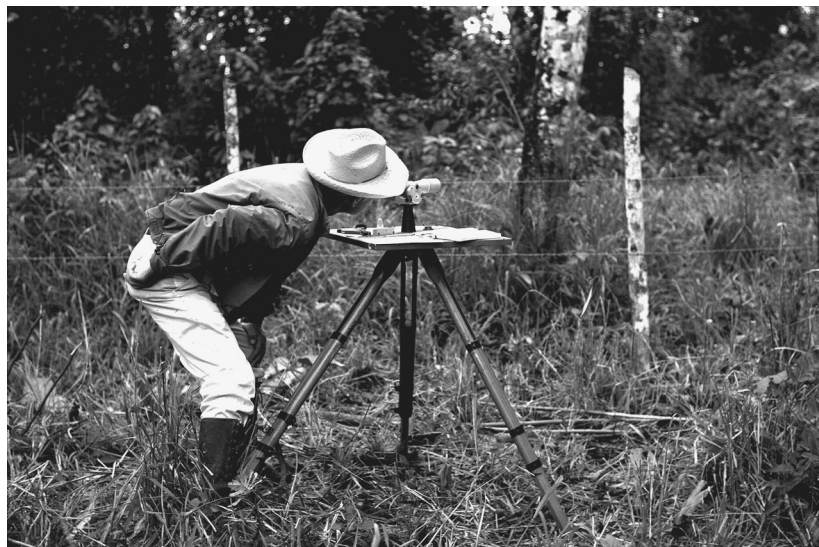
Fig. 9.2. Ray Krotser mapping at San Lorenzo with an alidade and plane table. In spite of the site's size and tropical vegetation, he created a very detailed topographic map of the San Lorenzo plateau. Photo courtesy of Michael D. Coe.
