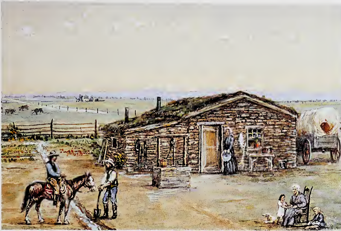
Sod House by William Henry Jackson, 1936. On the treeless prairies lumber was at a premium, so pioneers often used densely packed sod for building their homes.
