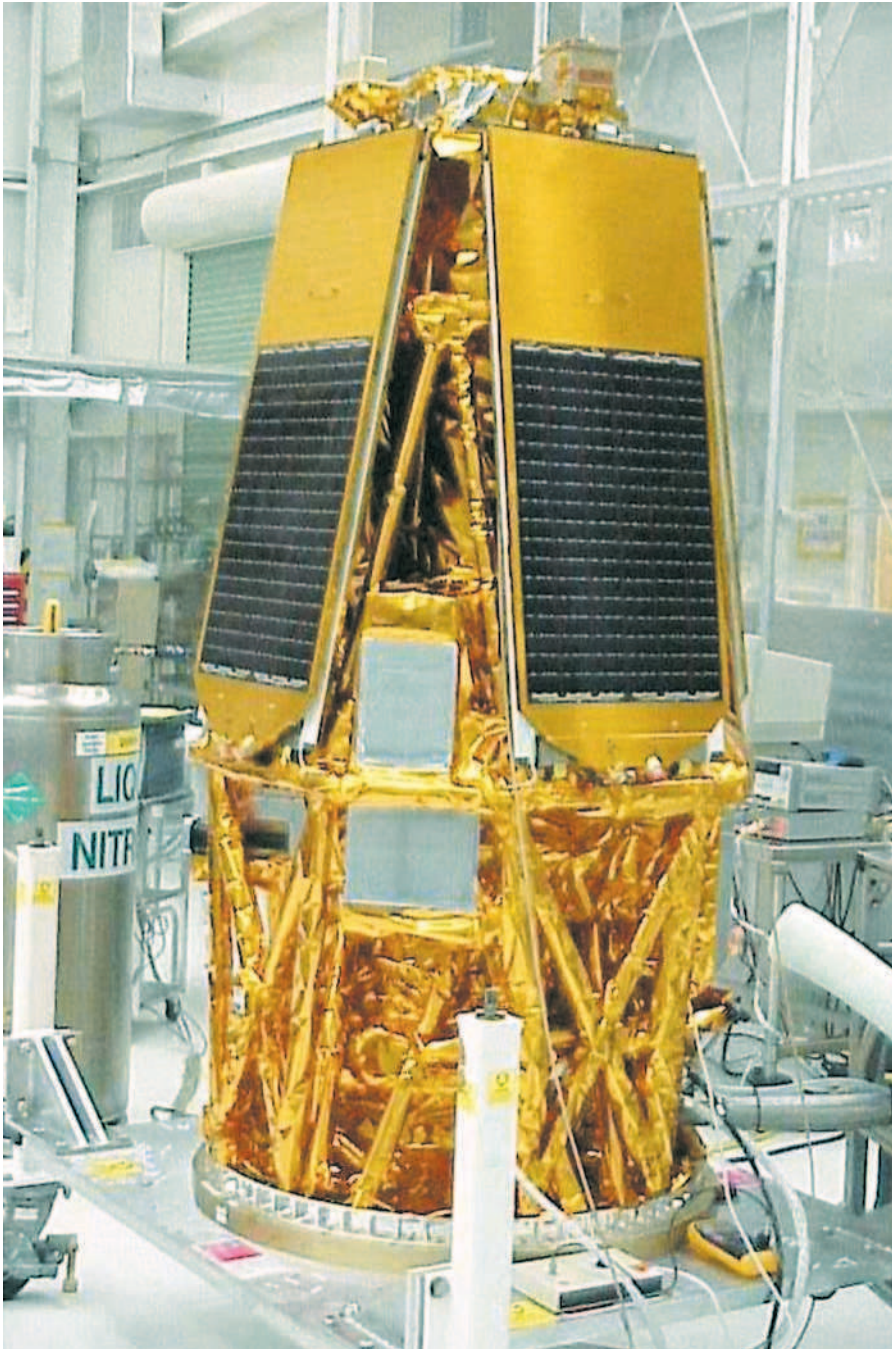
Typical spacecraft bus (High Energy Solar Spectroscopic Imager [HESSI] built by Spectrum Astro, Inc., for NASA).
