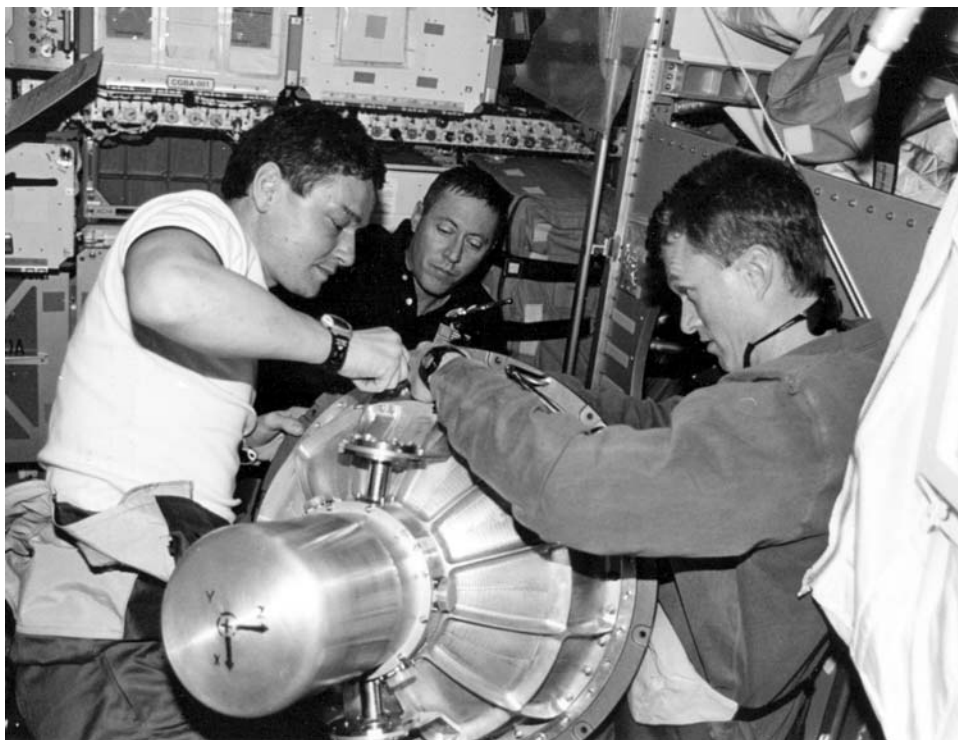
Valeri Korzun (left) works with Mike Baker and Brent Jett to unstow a gyrodyne device for attitude control, and then transfer it to Mir. They are pictured in the SpaceHab double module which is packed with logistics to transfer to the space station
