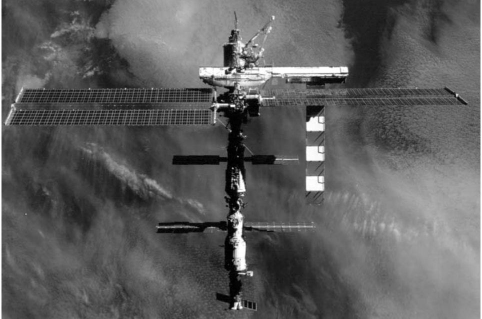
The International Space Station as of October 2002. The departing Atlantis crew photographed the station following the undocking, and the newly added Starboard 1 (S1) Truss is visible in upper centre frame
