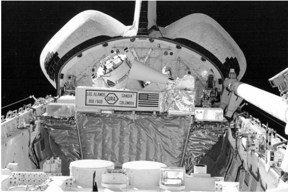
This view of the payload bay of Discovery reveals some of the STS-39 payload, including the top of the STP-1 payload on the Hitchhiker carrier, and the AF-675 package comprising CIRRIS-1A, FAR UV, HUP, QIMMS and the URA
