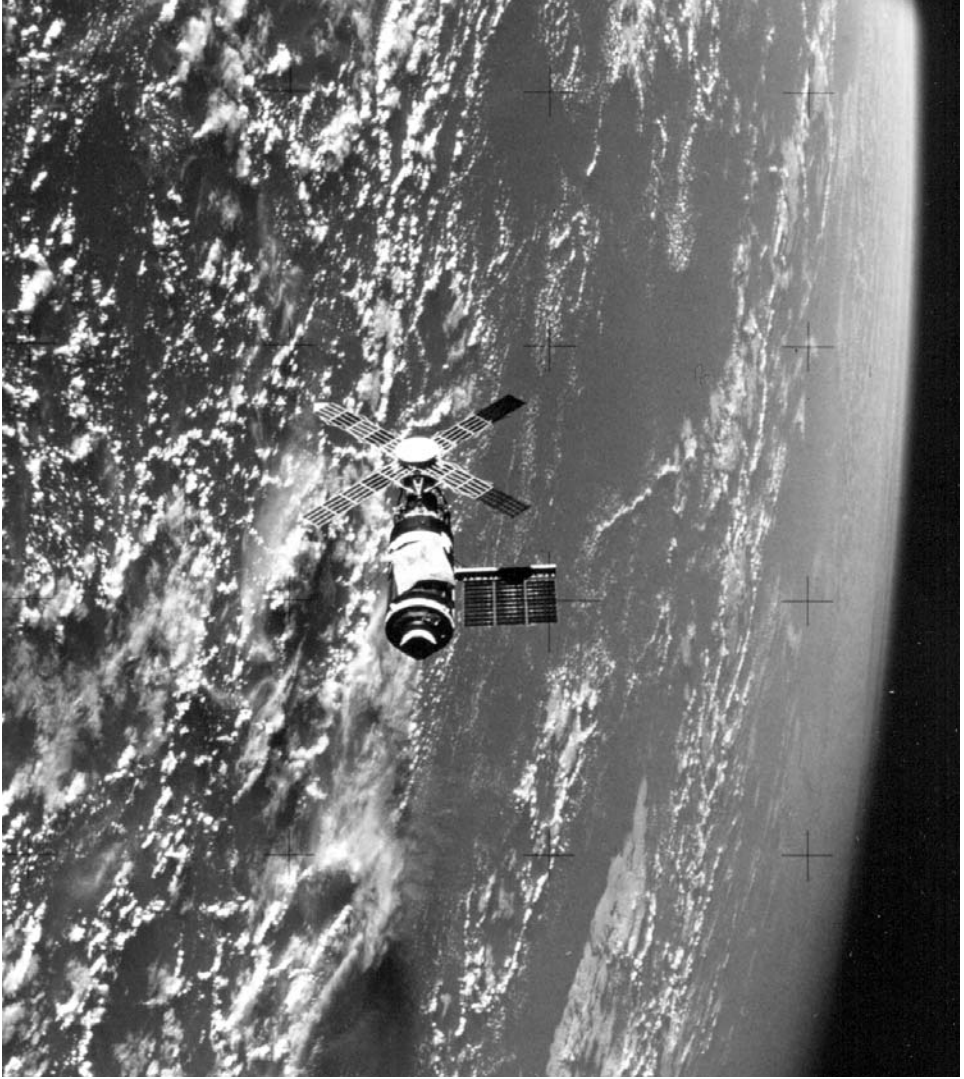
The Skylab Orbital Workshop in orbit, showing its one remaining solar panel and the parasol sunshield
