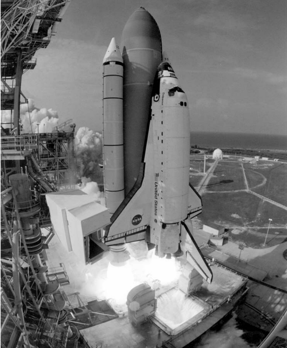
With the Solid Rocket Boosters lit, the Shuttle is committed to launch
