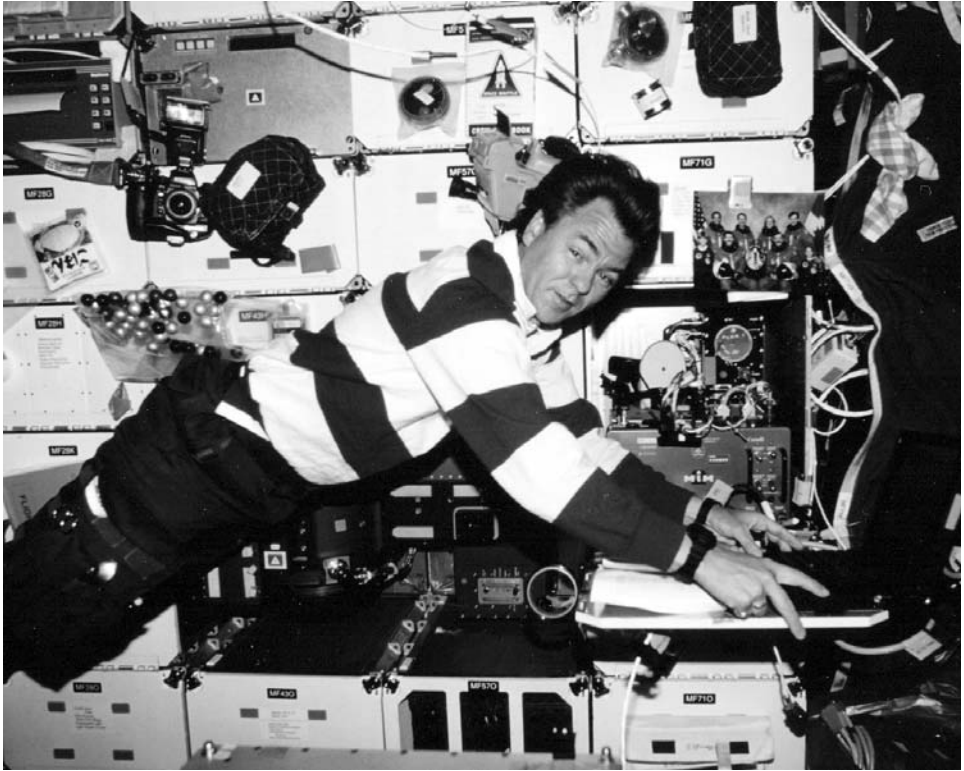
Canadian astronaut Bjarni Tryggvason inputs data into a computer for the Microgravity Vibration Isolation Mount (MIM) experiment located on the mid-deck of Discovery. Behind him, the use of mid-deck lockers for stowage both inside and outside is evident
