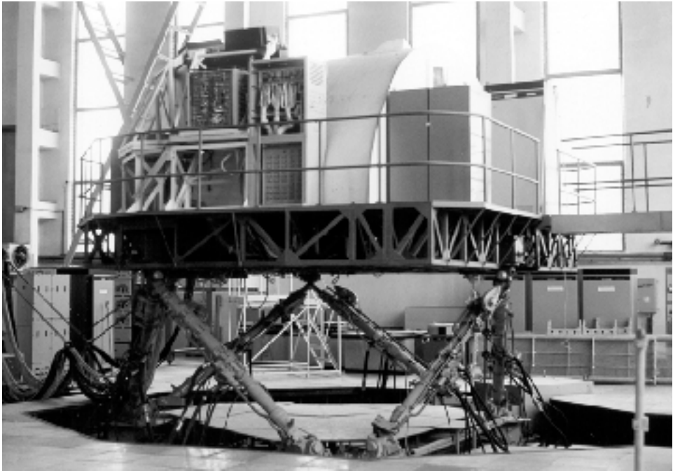
TsPK's motion-base Buran simulator (B. Vis).
