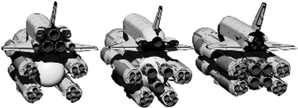
Soviet shuttle evolution. From left to right : OS-120, OK-92, and Buran ( source: www.buran.ru ).
