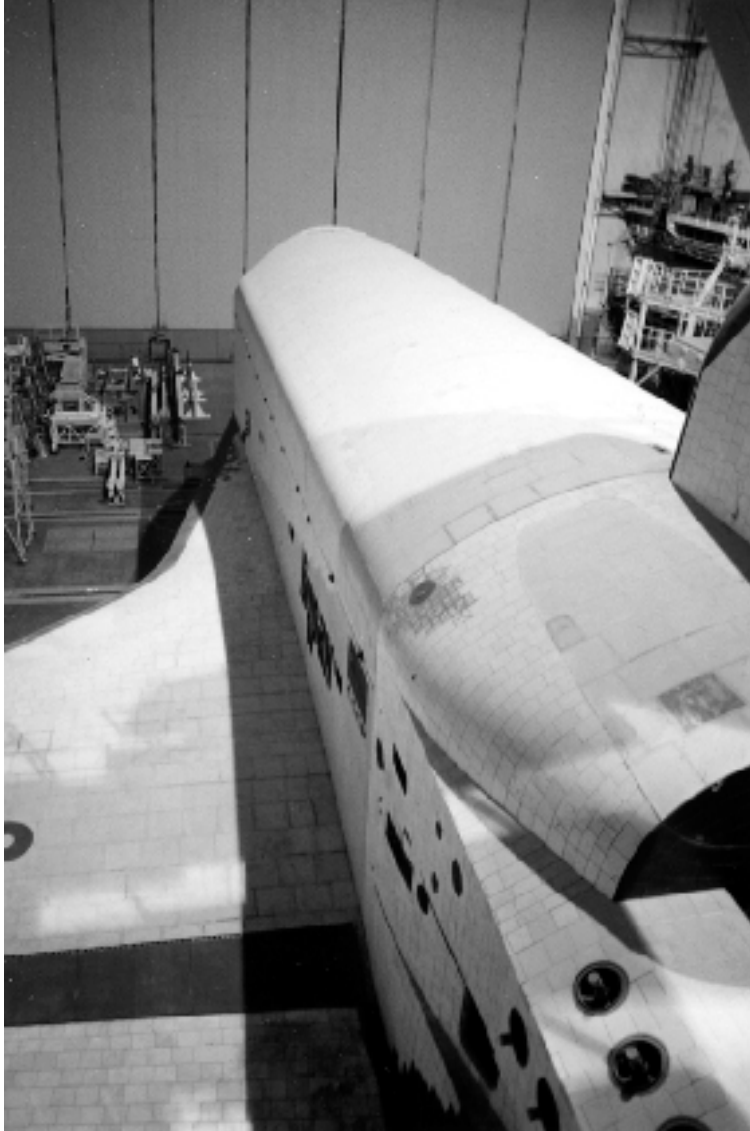
Post-flight picture of Buran shows one of the engine niches covered with flexible thermal insulation panels (B. Vis).
