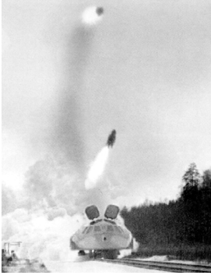
Ejection seats fired from a mock-up of Buran's cockpit (B. Vis files).
