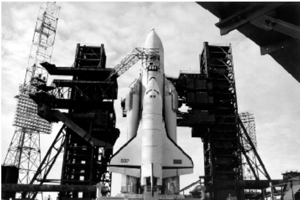
Image of Energiya–Buran showing the arm connected to the azimuthal alignment plate ( source: www.buran.ru ).
