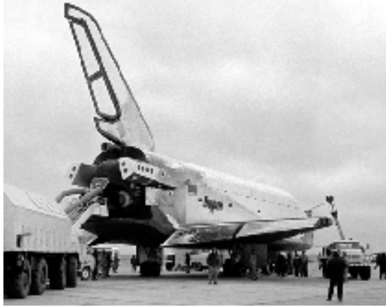
Post-landing operations underway. Note heavy scorching on aft fuselage and elevons ( source: www.buran.ru ).
