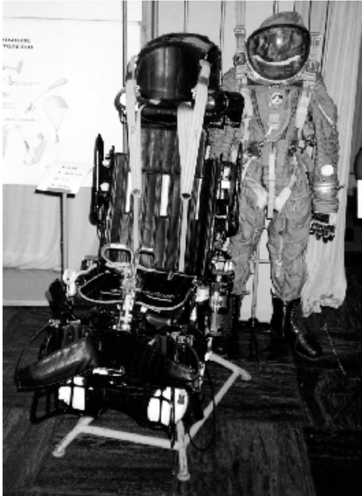
K-36RB ejection seat and Strizh pressure suit (B. Vis).
