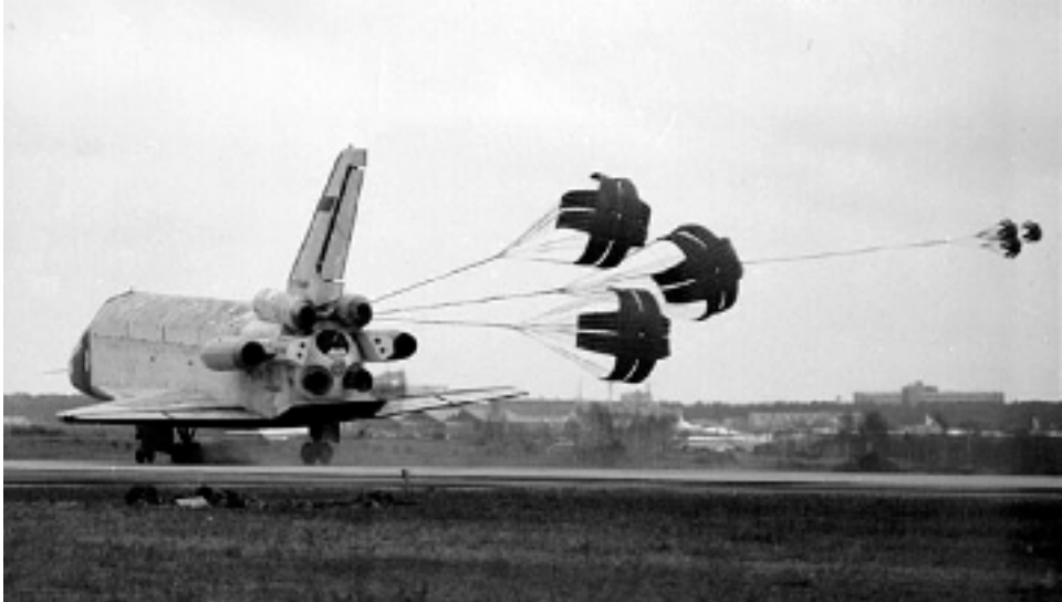
BTS-002 atmospheric test model with drag chutes deployed ( source: www.buran.ru ).
