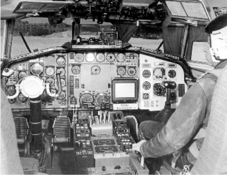
Rimantas Stankyavichus at the helm of a Tu-154LL flying laboratory with Buran cockpit lay-out (B. Vis files).
