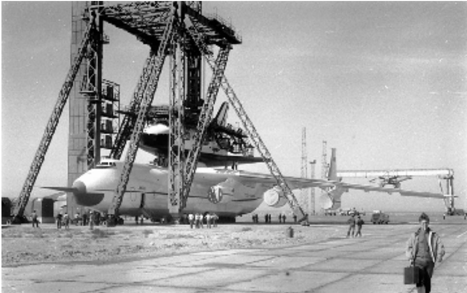
Buran being installed atop Mriya using the PUA-100 mate-demate device ( source: Sergey Grachov ).
