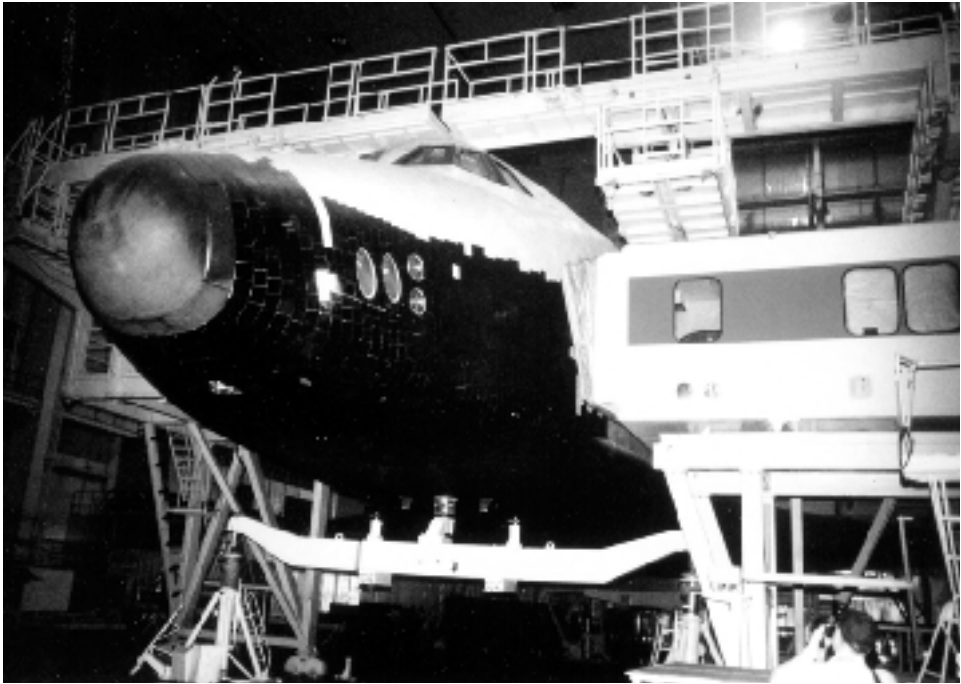
GRAVIMOL material covers Buran's nosecap (B. Vis files).
