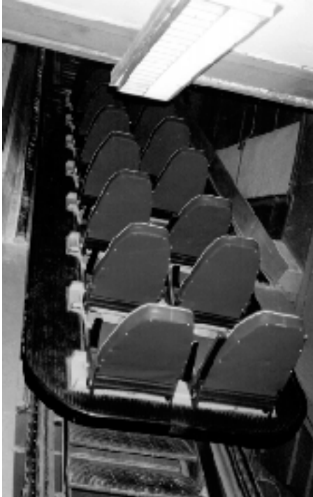
Trolleys used to ferry crews and personnel to and from the orbiter access arm ( source : Edwin Neal Cameron).
