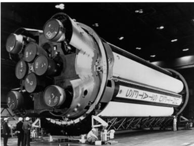
The eight-engine first stage of the Saturn C-1 launch vehicle.
