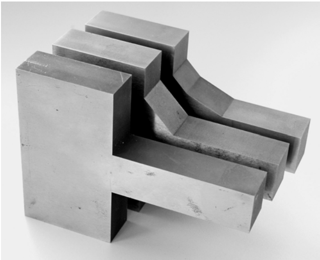
Figure 9: Non-optimized specimen (front) and two specimen with different degree of optimization.
