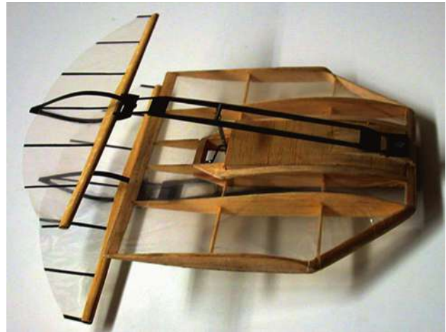
Fig. 18 First complete MAV prototype with a fixed forward wing for lift. Span length = 15 cm
