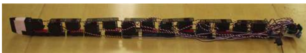
Fig. 3 The image shows the 13 servomotors comprising the robotic lamprey. Each servomotor is connected to its neighbours by rigid links
