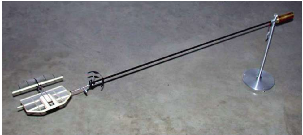
Fig. 19 Rotating-arm test stand for the MAV to measure lift and drag
