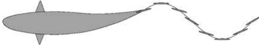
Fig. 1 The tail (caudal fin) of a thunniform swimmer (e.g., tuna and many sharks) forms the main source of propulsion. The tail can be effectively approximated as a heaving and pitching foil
