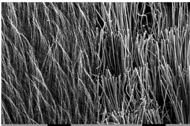
Fig. 17 Surface structure of the natural owl wing (left) and the applied velvet (right). The black bar at the bottom represents a length of 400 \mu\text{m}
