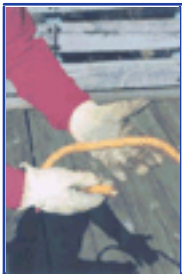
Figure 25-7 Example of ½-inch, nylon, static, kernmantle rope of the type commonly used in rescue. Rescue rope should be checked over its entire length for damage before use.
