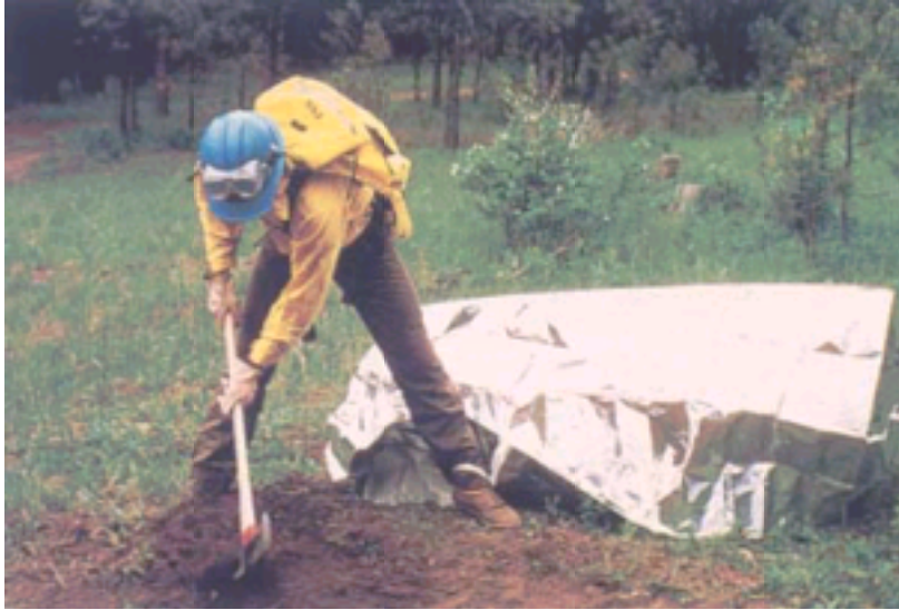
Figure 12-7 An aluminized fire shelter, carried in a waist pouch, is deployed by firefighters as a last resort to provide protection from radiant heat and superheated air. (Courtesy the USDA Forest Service.)
