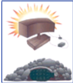
Figure 20-9 Above, A directional type mine used against unarmored vehicles or personnel. Below, An improvised mine, or booby trap, manufactured from a hand grenade and materials at hand.
