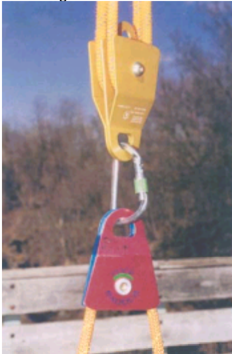
Figure 25-14 Two types of pulleys commonly used for rescue. Top , 2-inch double pulley. Bottom , 2-inch, "Prusik-minding." Note that rescue pulleys are applied to rope by removing the carabiner and swiveling the side plate to allow the introduction of the rope.
