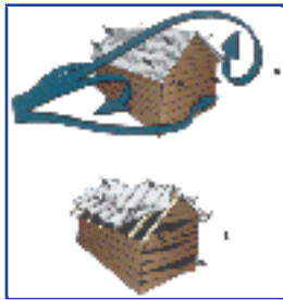
Figure 68-8 How high winds damage buildings. A , Wind blowing into a building is slowed at the windward face, creating high pressure. The airflow separates as it spills around the building, creating low pressure or suction at the end walls, roof, and leeward walls. B , The roof may lift off and the walls blow out if the structure is not specially reinforced. (Courtesy Disaster Management Center, University of Wisconsin.)
