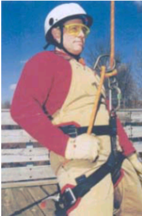
Figure 25-11 Example of figure-8 plate descending device (with "ears") commonly used in rescue.
