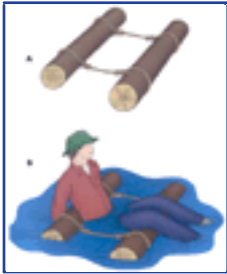
Figure 29-8 Log flotation device. A, Two lightweight logs are tied together. B, Device in action.
