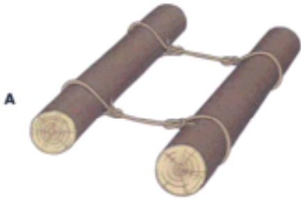
Figure 29-8 Log flotation device. A , Two lightweight logs are tied together. B , Device in action.
