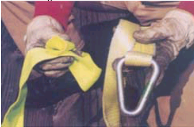
Figure 25-8 Left , Tubular webbing with cross section visible. Right , Flat webbing used in anchor sling.
