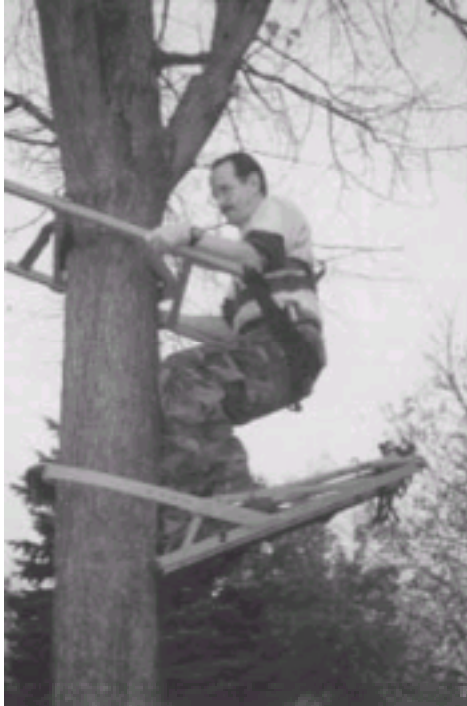
Figure 20-2 A commercially produced tree stand can be used to climb the tree and obviates the need for a ladder or steps, which are the cause of many falls.
