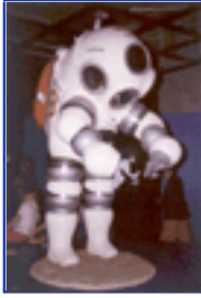
Figure 57-1 JIM diving suit. The diver remains at sea level pressure inside the suit and can work for prolonged periods of time at extreme depths underwater.
