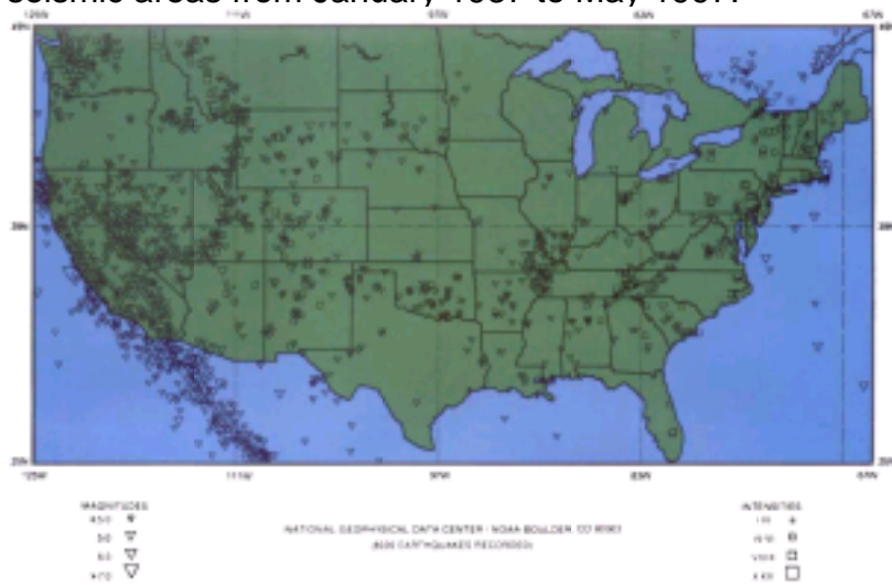
Figure 67-5 Earthquake risk in the continental United States. Triangles represent active seismic areas from January 1937 to May 1997.
