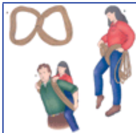
Figure 19-43 Split-coil seat. A , Rope coil is split. B , Victim climbs through rope. C , Rescuer hoists the sitting victim.
