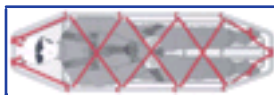
Figure 26-32 One 10-m (30-foot) web or rope can be used to secure a person into a litter.
