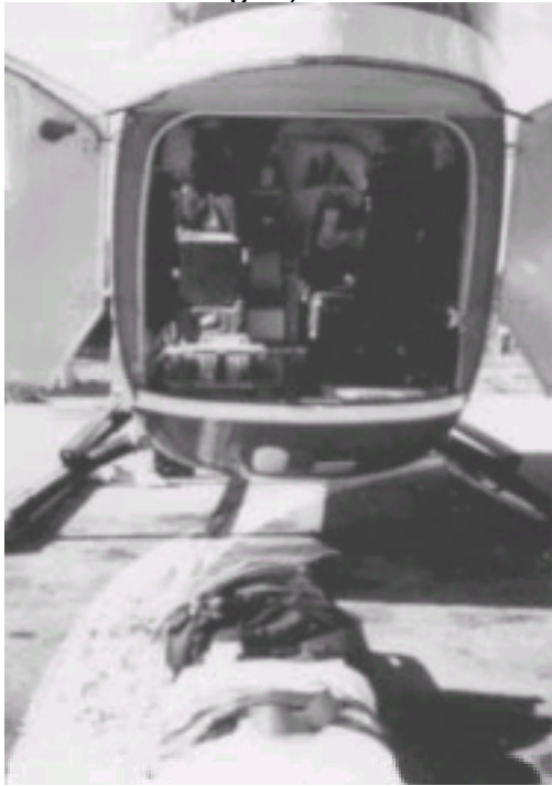
Figure 27-6 MBB BK-117 with rear clamshell doors open. (Courtesy Susan Lockman, Stanford Lifelight.)
