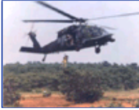
Figure 27-1 MH-60G Pave Hawk hoisting a pararescueman during a search and rescue exercise. A variant of the UH-60 Blackhawk, the Pave Hawk is flown by U.S. Air Force rescue squadrons. Modifications include forward-looking infrared equipment, night-vision-compatible cockpit lighting, terrain and navigation radar, air refueling probe, auxiliary fuel tanks, and hoist. (Courtesy U.S. Air Force.)
