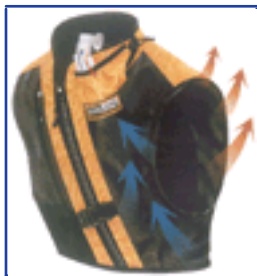
Figure 69-4 The AvaLung (Black Diamond, Ltd.). A lightweight vest designed to improve avalanche survival. Victims are able to draw air from even a dense snowpack via the front using an air exchange mouthpiece. A one-way valve permits exhalation of carbon dioxide expelled through the vest back.
