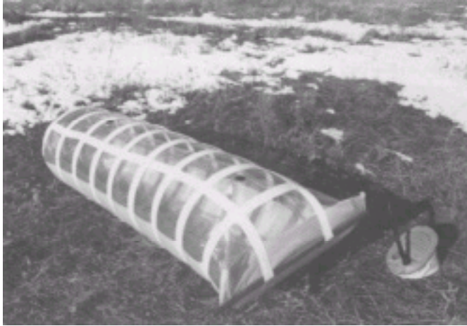
Figure 1-12 The HELP System (Live High, Boulder, Colo.) uses breathing bladder technology to minimize the pumping necessary to circulate air in the hyperbaric compartment.
