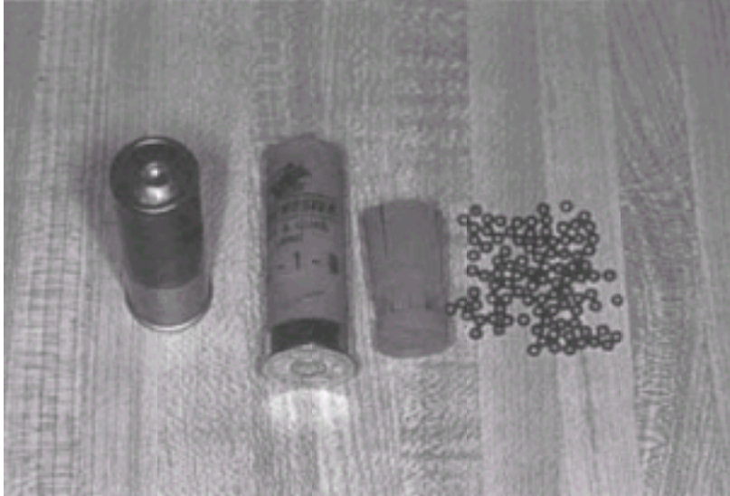
Figure 20-6 Examples of shotgun rounds. Left to right , 12-gauge slug round, empty 12-gauge plastic round, plastic 12-gauge wadding, and number six shotgun pellets.
