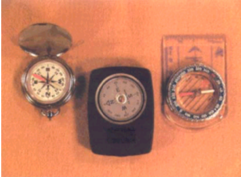
Figure 73-2 The three basic compass types. From left to right: Fixed dial compass, magnetic card compass, baseplate compass. Note the deviation in indicated north resulting from local magnetic influences.
