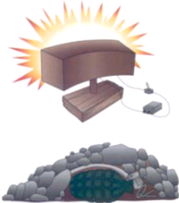
Figure 20-9 Above, A directional type mine used against unarmored vehicles or personnel. Below, An improvised mine, or booby trap, manufactured from a hand grenade and materials at hand.
