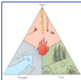
Figure 12-5 Combustion is a process involving the combination of heat, oxygen, and fuel. An understanding of the variation of these three factors is fundamental to an understanding of fire behavior.
