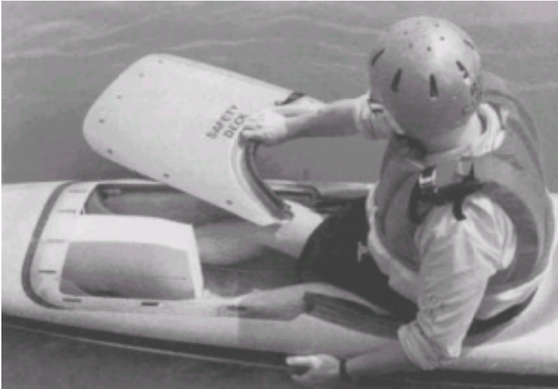
Figure 30-10 Safety Deck system, which offers an emergency exit for a kayaker in distress.
