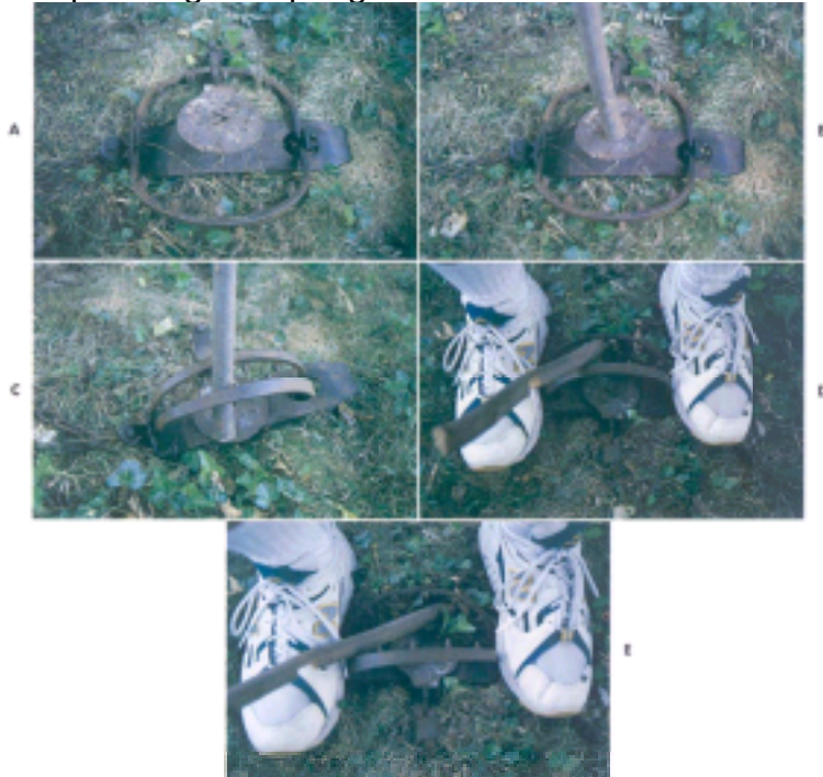
Figure 20-7 A , A leghold trap set. B and C , A leg hold trap sprung. D and E , How to release a trap that has been sprung by standing on each end of the trap and compressing the spring.
