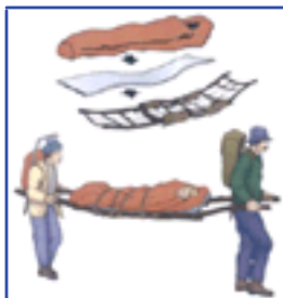
Figure 26-12 Packframe litter. Note that the sapling poles on the litter can be attached to the rescuer's pack frames to help support the victim's weight.
