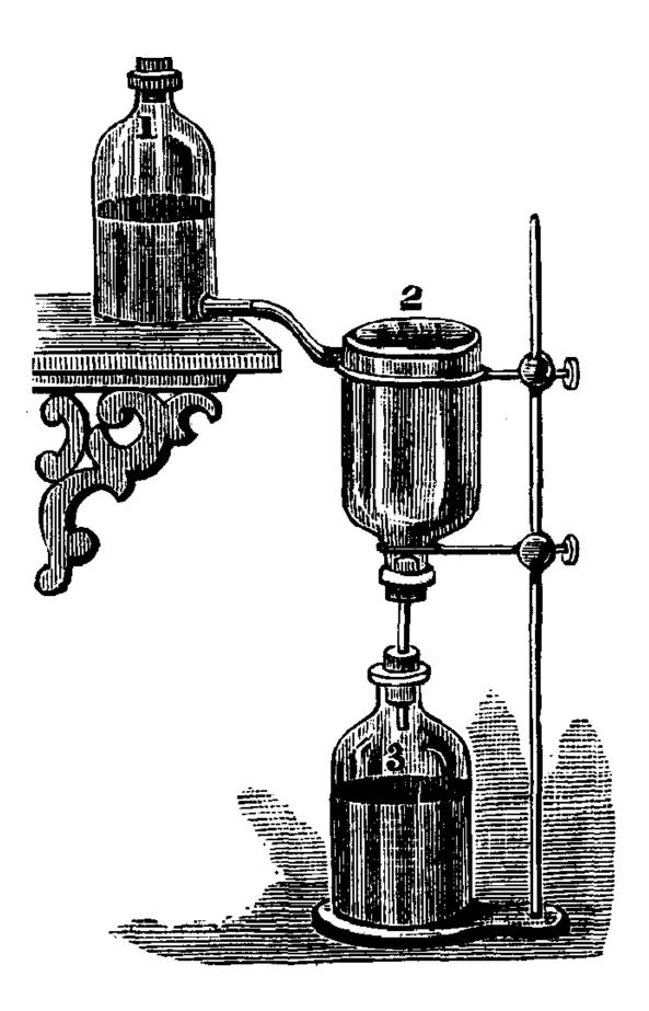
The lower orifice of No. 1 is connected with No. 2 by means of a short piece of vulcanized rubber tubing.
