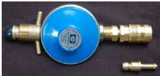
Fig 5.9.1 LPG regulator and 2mm jet used to control nitrogen flow
