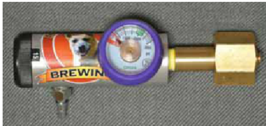
Fig 5.9.2 High pressure Max Dog nitrogen regulator with click flow rate output
