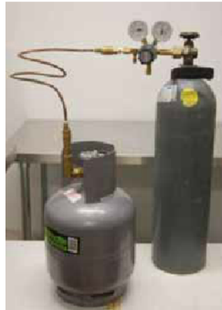
Fig 5.3: Filling a 4Kg LPG cylinder with 400 psi of Nitrogen
